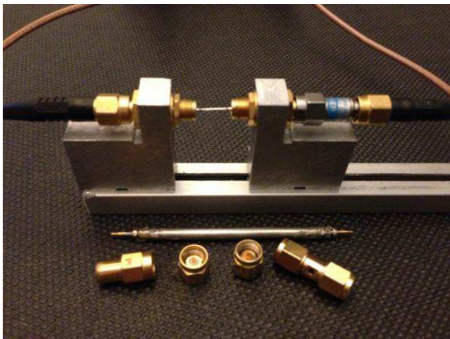
Figure 8 ~ Rail-mounted test fixture. The two end brackets each hold an SMA connector, which are connected with different length pins to hold a ferrite bead or toroid. The left image shows a close-up and the right image shows the fixture used with the VNWA-3E vector network analyzer setup in transmission mode. (images © 2013, K. Poulsen)
