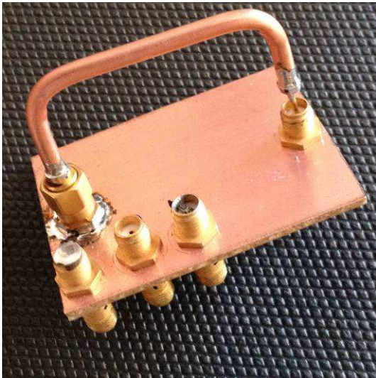
Figure 7 (left) ~ Poulsen's version of the PCB fixtures with built-in SMA SOL calibrators seen on lower-left corner. The U-shaped loop is made from a piece of semi-rigid coaxial cable with the shield and center conductor soldered together on the right end in the image. The arrangement shown allows the loop to be removed and reused in a test chamber shown later. It also allows larger solid beads and toroid cores to be slipped over the loop. (image © 2013, K. Poulsen)
