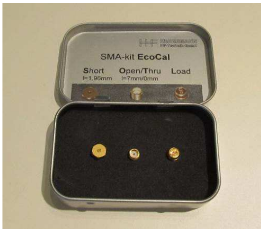
Figure 6 ~ Precision Short, Open and Load calibrators used for VNA calibration prior to bead measurements. These calibrators are based on SMA connectors and when not in use are stored in a small tin box. Note the dimensional information for the Short and Open/Thru units that is used to determine their electrical delays. (image © 2013, W. Reeve)
