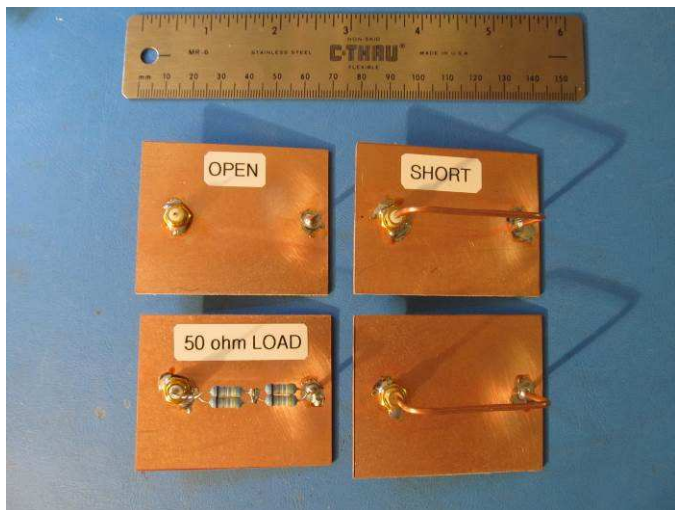
Figure 2 ~ Printed circuit board (PCB) fixtures with SMA connectors. PCB dimensions are 2.0 x 2.5 in (51 x 64 mm). A layout drawing was provided in Part I. These fixtures are used as Short, Open and Load for vector network analyzer calibration. A ferrite bead is then placed on the Short fixture for measurements. These fixtures provided usable measurements up to about 100 MHz. (image © 2013, W. Reeve)
