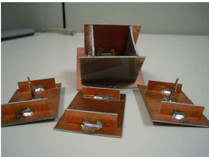
Figure 3 ~ Printed circuit board (PCB) fixtures built by Hagen with end brackets and sides. These fixtures provided no measurement advantages over other types. (image © 2013, T. Hagen)
