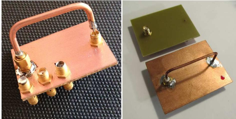
Figure 1 ~ Test fixtures made from printed circuit board (PCB) material. Left: The 2.5 x 2.0 in plate holds several SMA connectors. Three are for Short, Open and Load calibration. The loop holds the clamshell bead and plugs into the connectors on each end. The left connector shorts the loop to the copper PCB material and the other connects to the VNA. Right: Two PCB fixtures with a fixed shorting loop, one shown upside down. (left image © 2013 K. Poulsen, right image © 2013 W. Reeve)
