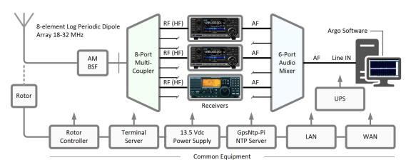
Figure 3 ~ System block diagram for the receiver instrumentation and related common equipment at Anchorage, Alaska. The receivers consisted of two Icom R-8600 wideband receivers and one Icom R-75 general coverage receiver, all set to LSB mode and connected through an audio mixer to the PC soundcard and ultimately demodulated by Argo. The HF log periodic antenna was pointed on a 107° true azimuth toward WWV. Image © 2021 W. Reeve
