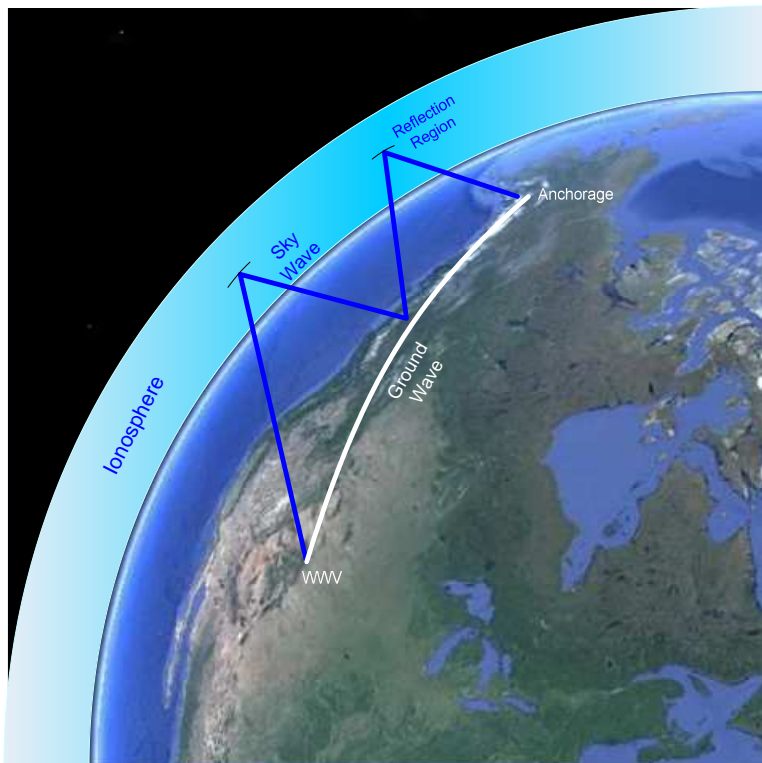
Figure 4 ~ Ground wave and sky wave propagation concepts. A 2-hop sky wave path and a ground wave path are shown for illustration, but ground wave propagation from the WWV transmitter to Anchorage is highly improbable because of the distance (about 3800 km). Underlying map image courtesy Google Earth.
