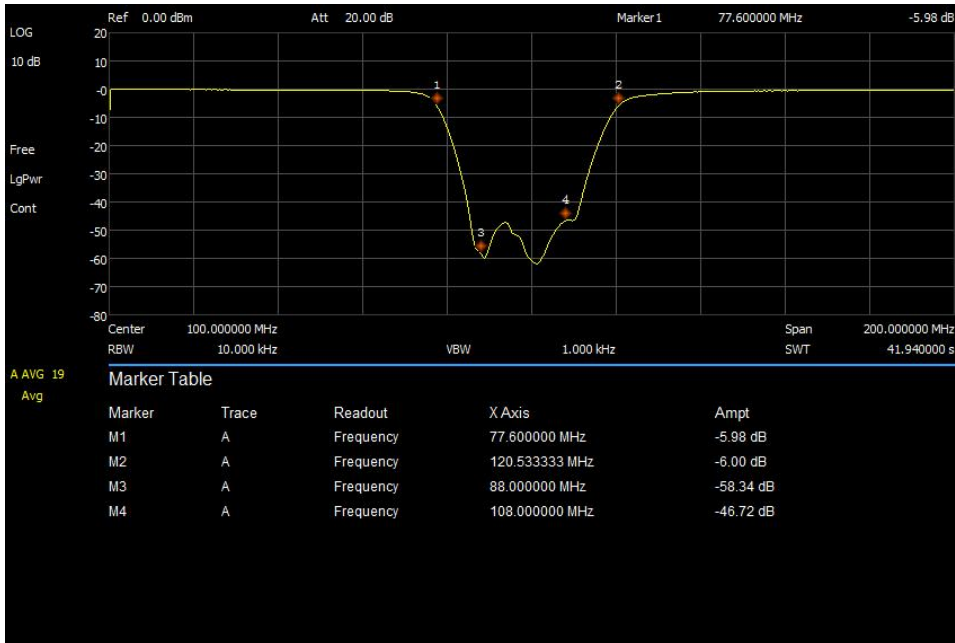
Figure 6 ~ Response of a Mini-Circuits FM broadcast bandstop filter. Markers 1 and 2 are set to the 6 dB corner frequencies (other values may be used such as 1, 3, 10 or 20 dB). The FM broadcast band edges are indicated by markers 3 and 4. The passbands are flat with rounded transitions into the stopband. The response decreases by about 50 dB in a span of only 10 MHz on the lower side and about 40 dB in a span of about 12 MHz on the upper side. This filter provides over 50 dB average loss in the band between 88 and 108 MHz. Image © 2020 W. Reeve
