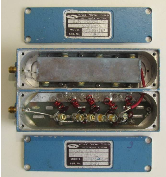
Figure 7 ~ AEL MW11200-167 bandpass filter for the 225 to 400 MHz US military aerospace frequency band. This is a cascaded filter designed as two mechanically and electrically separate lowpass and highpass filters (upper and lower sections, respectively). Each section has its own cover and RF connector (see at left). Both filters are made with lumped elements and were obviously hand-built and aligned by adjusting the variable piston capacitors and by bending the coils to adjust their inductance. A copper plate shields the lowpass section, and a red insulated conductor connects the two sections through a hole between the two enclosures on the right side of this image. This conductor has significant inductive reactance at VHF and UHF and so is part of the overall filter design. The filter components are mounted on printed circuit boards that consist only of isolated pads for soldering the component leads. The enclosures are machined from aluminum blocks and have tight-fitting covers. This construction is typical of AEL filters for the HF, VHF and lower UHF bands. Image © 2020 W. Reeve
