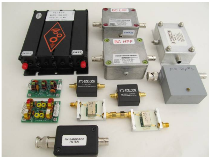
Figure 2 ~ Typical connectorized commercial filters of various types (highpass, lowpass, bandpass, bandstop) and covering various frequency bands. These filters include Mini-Circuits, Par Electronics, Industrial Communication Engineers, RTL-SDR.com, two exposed hand-built HF bandpass filters from kitandparts.com, and others. Note the variety of mechanical form factors and RF connectors, which include type SMA, BNC, pin header, and RCA phono jack. Not shown are specialized filters and a digitally controlled HF preselector that will be discussed in a future article. Image © 2020 W. Reeve
