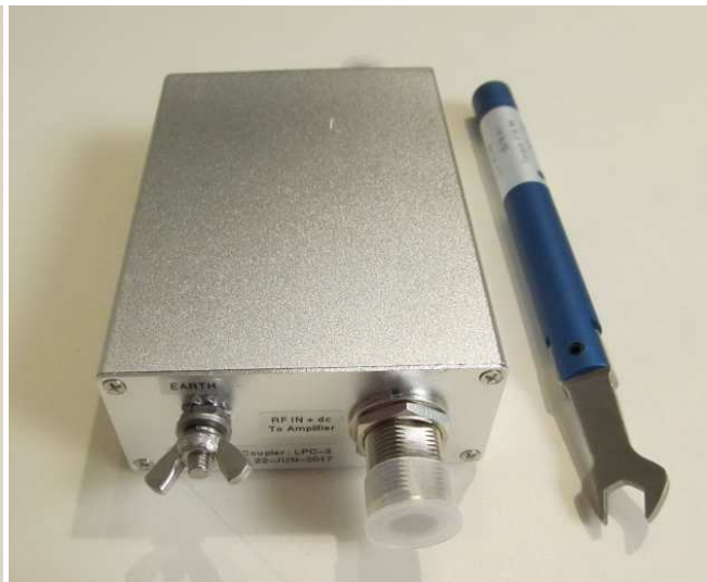
Figure 9 ~ Three views of the completed bias-tee package: Upper : The inside view shows all components and cabling in place. Lower : Bias-tee assembly with cover in place. The wrench is an 8 mm (5/16 in) torque wrench for the SMA connectors. The type N connectors are shown with protective caps.
