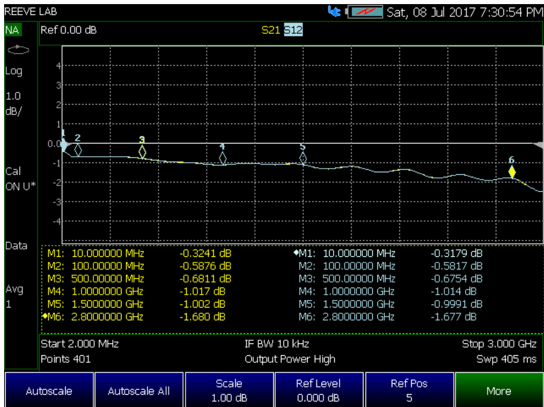
Figure 11 ~ S21 and S12 scattering parameters from 2 to 3000 MHz. S21 (yellow trace) and S12 (blue trace) are insertion losses in terms of dB reduction from zero with scale factor of 1 dB/div. The two traces are almost indistinguishable. S21 measures the loss from the RF+dc port to RF port and S12 is the reverse direction. The more positive the insertion loss value, the better (0.0 dB is ideal). These measurements indicate the insertion loss increases steadily as frequency increases but is less than 1.7 dB at 2800 MHz.
