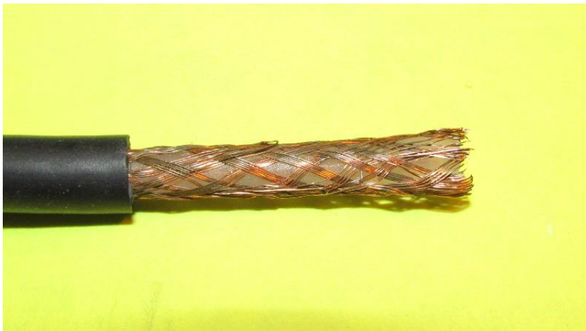
Figure 5 – Coaxial cables stripped 25 mm to reveal the shields. The five cables on the left have very few strands in the shield and the strands are very loosely braided. All cables except the RG-213/U, RG-58A/U, RG-59/U and Jasco “RG-59U” have a foil shield under the braid. The 75 ohm cables shown here are for in-home cable television and satellite television distribution. The LMR-400-DB cable is designed for direct burial applications – the interstitial spaces are filled with a waterproofing compound.
