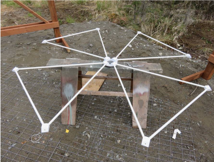
Figure 12 ~ A sawhorse holds the four triangular tie and link frames, which have been fastened to the cast steel flange fitting at center. The assembly supports the four dipole elements – two for each dipole of the crossed-dipole assembly. The triangular supports are made from solid fiberglass rods fastened to trapezoidal blocks at the vertices of each triangle assembly. The four individual frames are supplied preassembled. Note the ground grid. Image © 2017 W. Reeve
