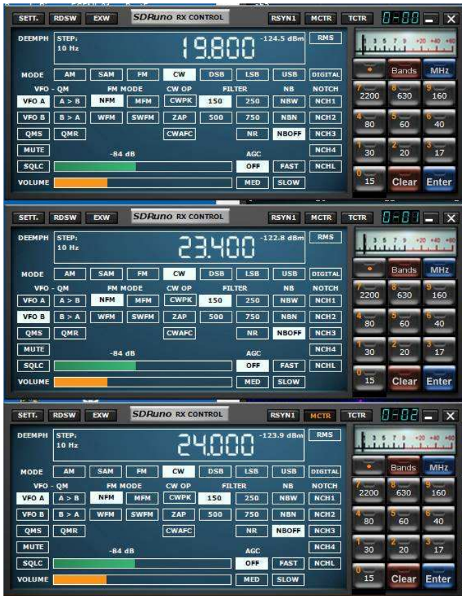
Figure 10 ~ Three RX Control (VRx) windows shown tiled. These are numbered consecutively 0-00, 0-01 and 0-02 as seen in the upper-right corner of each window. The VRx window is used to set the desired receiver frequency. This frequency also will be displayed in the corresponding Main Spectrum window SP1 as the receiver frequency. The LO frequency displayed in all virtual receiver Main Spectrum windows will be the same.
