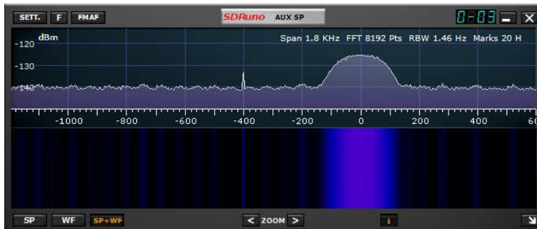
Figure 15.a ~ Auxiliary Spectrum window showing the IF spectrum for the received signal at 16.4 kHz, which is centered at 0 Hz on the frequency scale. FFT averaging was used to smooth out the visible noise floor and accentuate the signal. Note the smooth Gaussian shaped spectrum indicative of VLF transmissions used by the US Navy. The resolution bandwidth indicated is 1.46 Hz.
