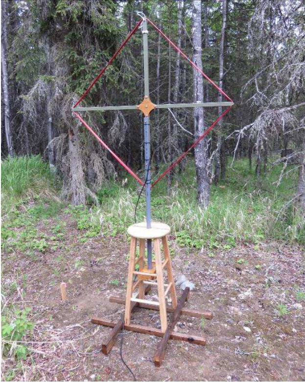
Figure 6 ~ Temporary installation of the square loop antenna on a modified bar stool. The loop frame is fastened to a 1 in (trade size) PVC conduit mast, which is inserted in the stool for easy rotation. The bar stool is equipped with braces for the mast and outriggers to prevent upset in the wind. The whole assembly is very easily relocated. The loop locations investigated are in a heavily wooded area mostly with quaking aspen and black spruce trees and some open spaces frequented by rampaging moose (the permanent installation places the antenna high enough to prevent moose interference). Image © 2018 W. Reeve
