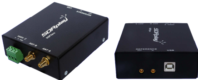
Figure 3 ~ SDRPlay RSP2Pro software defined radio receiver. Dimensions are 99 x 87 x 33 mm, 0.3 kg. The balanced high-impedance antenna interface is the green pluggable connector on far-left. The receiver is powered through its USB connection and draws about 170 mA at 5 Vdc. Images source: SDRPlay, used with permission.
