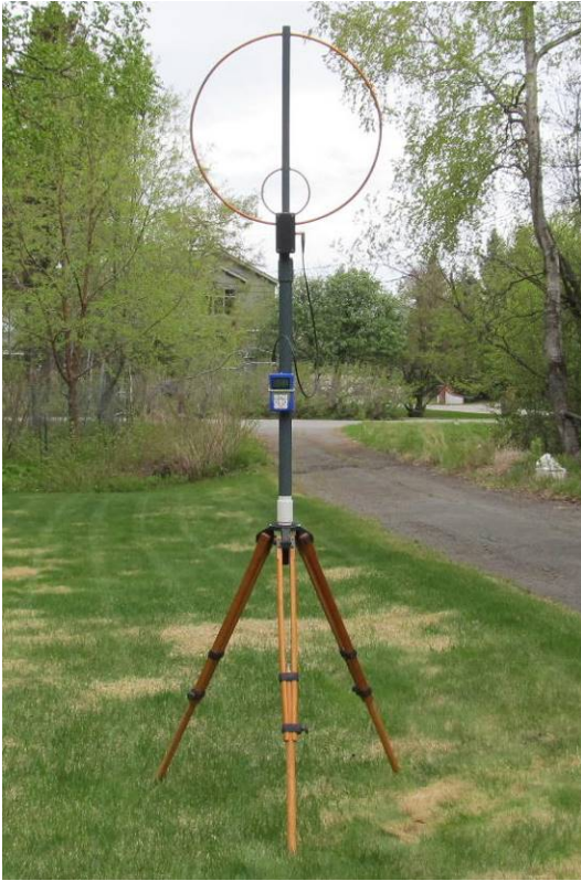
Figure 11.d ~ Shop-built loop antenna specifically made for locating HF band interference. A loop like this is not very sensitive but still useful if the interference source is nearby. The main loop has 1-turn of 3/8 in (10 mm) diameter copper tubing mounted on a mast made from a piece of PVC pipe. The main loop diameter is 24 in (610 mm). The small coupling loop is made from 1/4 in (6 mm) diameter copper tubing and has a diameter of 6 in (152 mm). A variable tuning capacitor is mounted in a small plastic box at the base of the loop and is used to resonate the main loop in the HF band. A balun couples the small loop to a BNC-F connector for connection to the analyzer via a short jumper cable. In this image, the loop support mast is temporarily installed on an EMC testing antenna tripod. The WSUB1G+ is lashed to the mast with a small bungee cord and is visible in the center of the image. Image © 2020 W. Reeve
