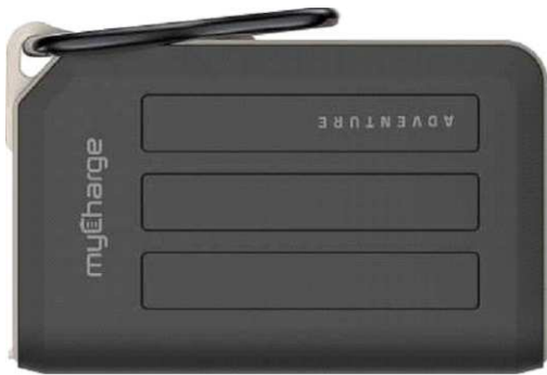
Figure 2 ~ myCharge – Adventure Max portable charger is typical of battery power supplies that may be used for powering the instruments through their USB ports. The battery in this unit is advertised as 10 050 mAh. It is charged through a micro-USB port and it has two USB-A output ports that supply 5 Vdc. Dimensions are 1.0 L x 2.4 W x 4.4 H in (25.4 x 61.0 x 112.3 mm) and weight is 0.55 lb (0.25 kg) – approximately the same size as the RF Explorer WSUB1G+.
