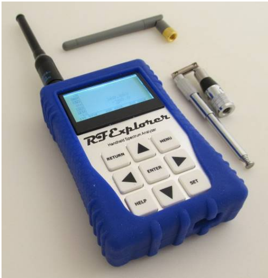
Figure 11.a ~ The RF Explorer WSUB1G+ is quite sensitive and is most useful when paired with a directional antenna, unlike the three mostly useless non-directional stub antennas shown here. The black collapsible whip antenna on the instrument extends to 15.5 in (390 mm), corresponding to a 1/4\text{-}\lambda at 200 MHz. The silver collapsible hinged whip antenna on the right extends about the same length. The hinged antenna at top is designed for 2.4 GHz applications (it was supplied with the instrument along with the black antenna). For lower frequencies, physically larger antennas are required unless the interfering signals are extremely strong and their source is nearby. Image © 2020 W. Reeve
