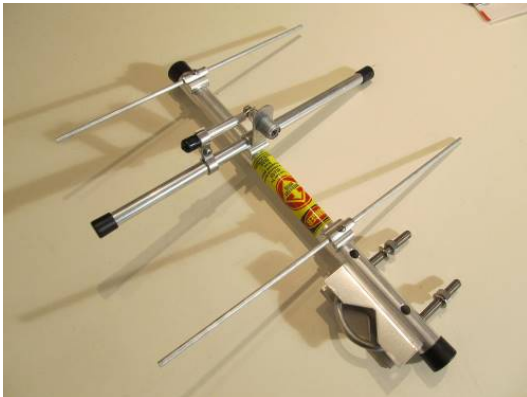
Figure 11.b ~ Laird P4063, 3-element Yagi antenna for the 406-430 MHz radio bands. The advertised gain is 6 dB and the 3 dB beamwidth is 100 H x 65 V degrees. It includes a mast clamp (lower-right) that may be mounted to a piece of non-conductive pipe or wood dowel for a hand-hold. An antenna like this can be useful for locating interference produced by arcing in powerline insulators and hardware. Image © 2020 W. Reeve
