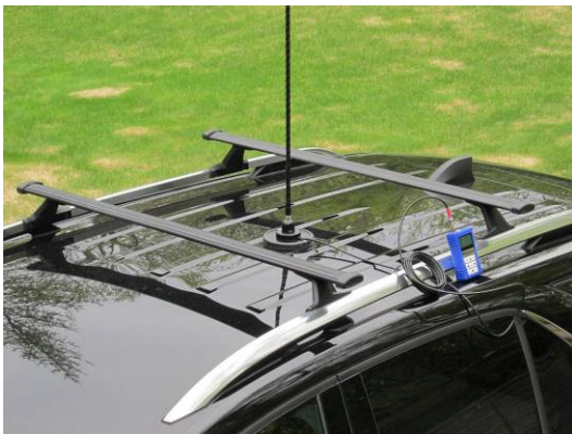
Figure 11.c ~ Tram magnetic antenna mount for vehicle roof installation (base can be seen in center of image). The mount is shown with a Procomm PCF15 antenna, which is a mobile vertical antenna designed for the 15 m (21 MHz) radio amateur band. It has a 44 in (1.1 m) long fiberglass lower section (visible on the mount) and adjustable stainless-steel upper section (not visible). The lower section has conformally coated integral inductors for modifying the antenna current distribution and effectively extending its electrical length. The antenna is roughly 1/8\text{-}\lambda at 20 MHz and may be used for locating powerline interference in the HF band. The WSUB1G+ is visible at center-right leaning on the luggage rack rail. Image © 2020 W. Reeve
