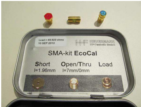
Figure 6 ~ Rosenberger calibration kit consists of Short, Open, Load and Thru standards that use SMA connectors. The kit is supplied in a tin box. The Open and Thru standards are the same barrel connector shown upper-middle. The slightly different reference plane locations of the Open and Short affect the calibration so a phase delay is manually entered into the software configuration to compensate. The Short (upper-left) and Load (upper-right) components are mechanically similar and have been color-coded for easy identification (red for the short and blue for the load). Image © 2016 W. Reeve
