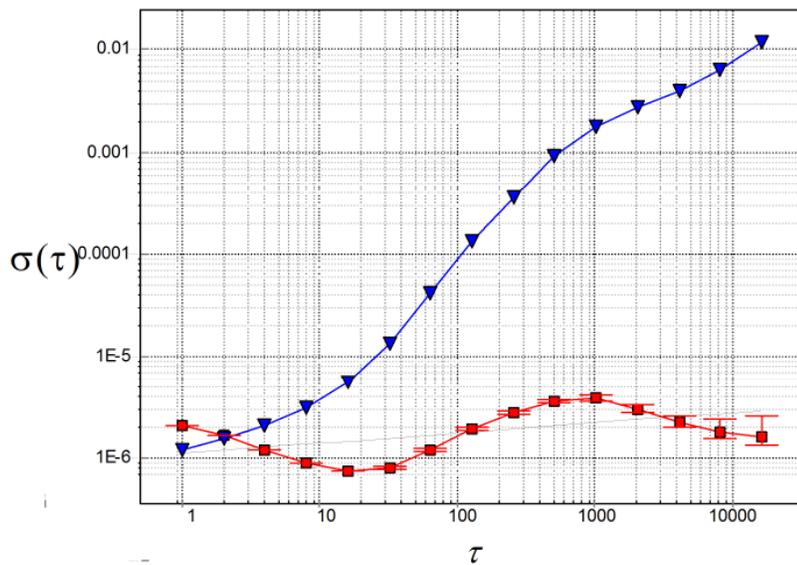
Figure 6(a) ~ TDEV (blue trace) and ADEV (red trace) with error bars for GpsNtp-Pi based on Adafruit board with GTop receiver. Standalone mode with 1 s sampling interval ( $\tau = 1$  s). The TDEV plot indicates some variation in offset for various averaging times. The ADEV plot shows that the stability is the best when the variance is calculated with an averaging time of approximately 17 s and is the worst at 1000 s.
