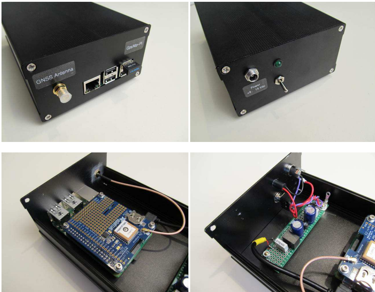
Figure 4 ~ Upper-left : GpsNtp-Pi system prototype packaged in an extruded aluminum enclosure 162 x 105 x 57 mm (external antenna not shown) with a dc-dc converter. A WLAN dongle can be seen in a USB port. Upper-right : The rear panel has a 2.1 x 5.5 mm dc power jack, power switch and power LED. Lower-left : The RPi is mounted on 6 mm standoffs and an adapter cable connects the Adafruit GPS receiver board to an SMA-F panel connector. Lower-right : A dc-dc converter converts the nominal 9...15 Vdc input to 5 Vdc for the RPi and is mounted on a small printed circuit card with a Pi input EMI filter and polarity guard diode. The RPi board supplies 3.3 Vdc to the receiver.
