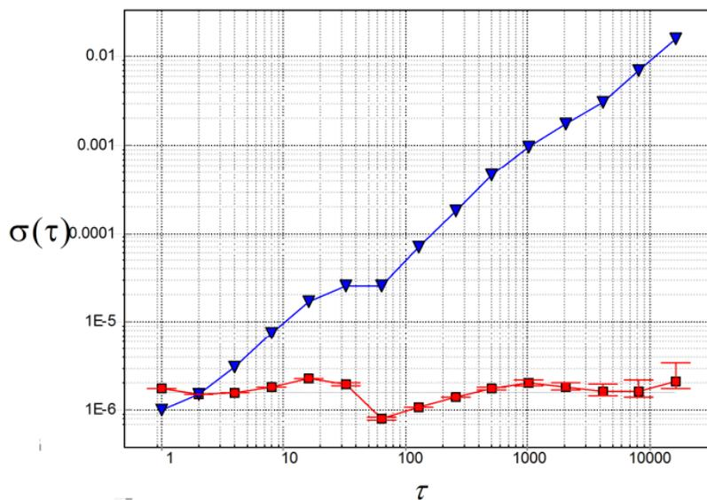
Figure 6(b) ~ TDEV (blue trace) and ADEV (red trace) with error bars for GpsNtp-Pi based on HAB Supplies board with uBlox receiver. Pooled mode with 1 s sampling interval ( $\tau = 1$  s). The TDEV plot shows a slightly more constant offset than the GTop receiver system. The ADEV plot shows that the stability is the best when the variance is calculated with an averaging time of approximately 67 s and is the worst at 17 s.
