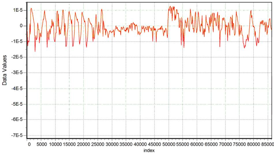
Figure 7(a) ~ Original data for GpsNtp-Pi based on Adafruit board with GTop receiver taken with 1 s sampling interval ( $\tau = 1$  s). The index is the sample number counted in sequence from the start time of 0000 UTC. The plot clearly shows systematic variations in the data, most likely caused by temperature variations. A setback thermostat engages at 0730 (index = 27 000 s) and disengages 7 h later (index = 50 000).
