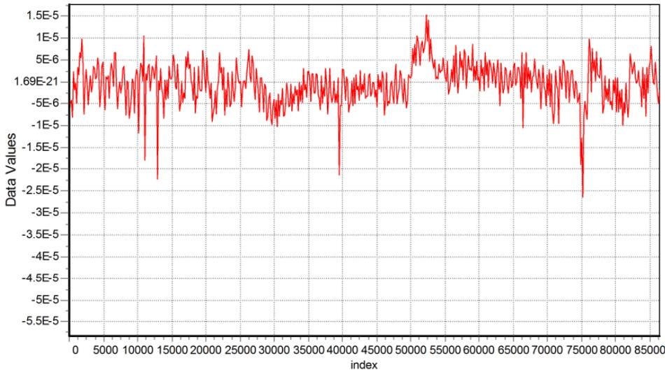
Figure 7(a) ~ Original data for GpsNtp-Pi based on HAB Supplies board with uBlox receiver taken with 1 s sampling interval ( $\tau = 1$  s). The index is the sample number counted in sequence from the start time of 0000 UTC. The plot shows systematic data variations similar to 7(a) but of a different character.
