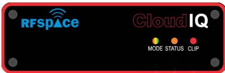
Figure 16 ~ Full scale image of Cloud-IQ front panel. The receiver requires 5 Vdc. It has two antenna input connectors on its rear panel that can be provisioned for specific frequency ranges between 9 kHz and 56 MHz. At HAARP the full range is setup on one connector (ANT1). Image source: RFSpace
