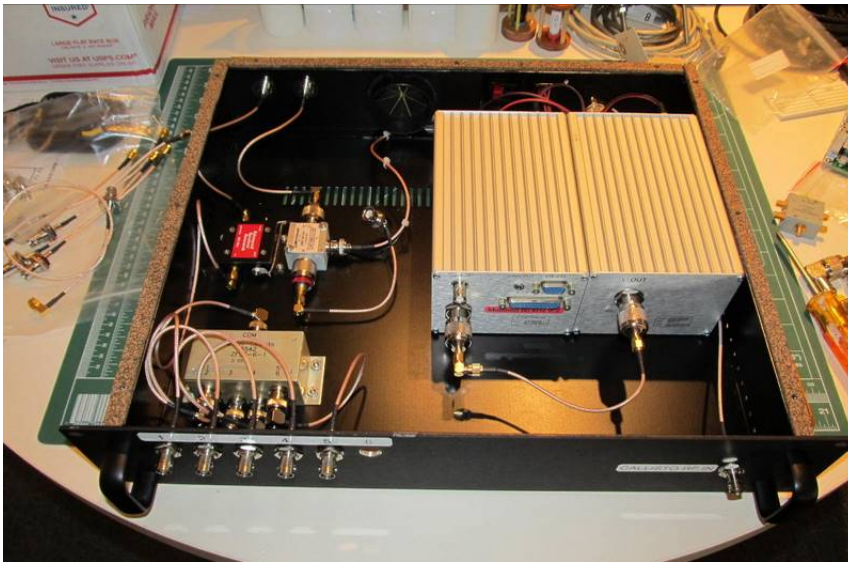
Figure 11 ~ RF enclosure. The bias-tees (an Advanced Receiver Research DC-INJ and a Mini-Circuits ZNBT-60-1W+) and splitter (Mini-Circuits ZFSC-6-1) are on the left side of the enclosure; the ARR bias-tee is active. The Callisto instrument is the extruded aluminum enclosure in the middle and the UPC232 up-converter is on the right side. Two 3 dB attenuators are connected to the Callisto RF input to control the transmission level point. Power connectors are on the rear panel behind the Callisto and converter. This image was taken in the shop prior to moving the unit to the HAARP site. Image © 2019 W. Reeve
