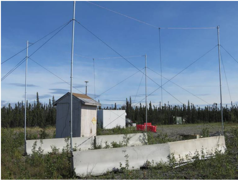
Figure 20 ~ Radio JOVE dual dipole antenna setup at HAARP. Concrete barriers were placed by HAARP staff in the east-west direction to support the four antenna masts. The masts were inserted in the ends of the barriers and then guyed with non-conducting strand to concrete block anchors (not visible in this image). The shed immediately behind the antenna houses a GPS antenna and receiver unrelated to this project. The equipment enclosure for the receivers and common equipment is in the middle-background. Image © 2019 W. Reeve
