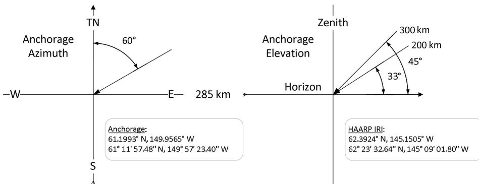
Figure 6 ~ Approximate azimuth (left) and elevation (right) for the propagation path to the F-region ionosphere directly above the HAARP site; Different HAARP beam angles will change the values slightly. Two ionosphere heights are shown because it can vary. Azimuth is with respect to True North (TN). Image © 2018 W. Reeve
