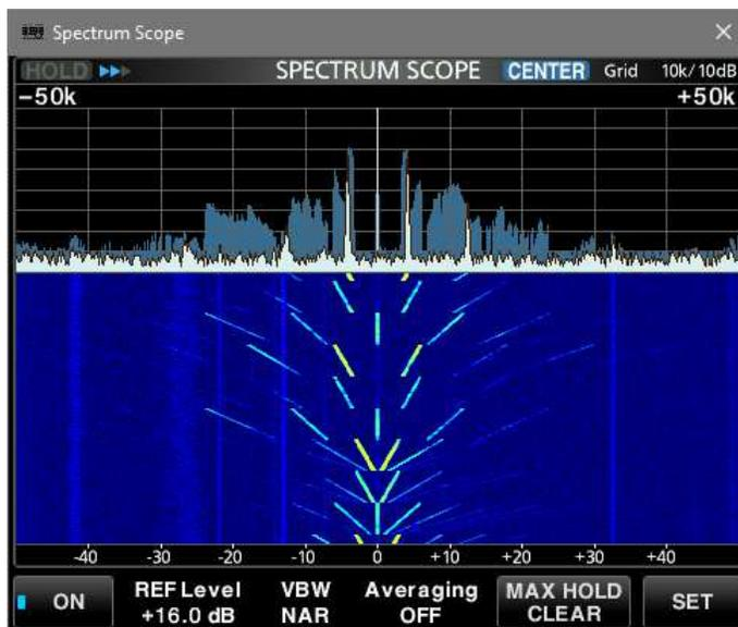
R-8600, 2.80 MHz, 100 kHz span, 4 December, 0141. HAARP setting 2.8 MHz. Chirp modulation.
