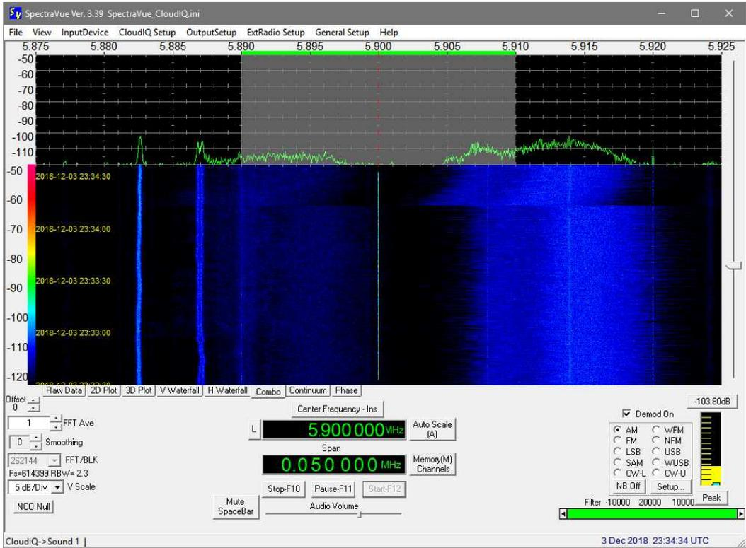
Cloud-IQ, 5.90 MHz, 50 kHz span, 3 December, 2324. Note that all indications on the waterfall are RFI except the line at 5.900 MHz. HAARP settings 5.9 and 7.2 MHz.
