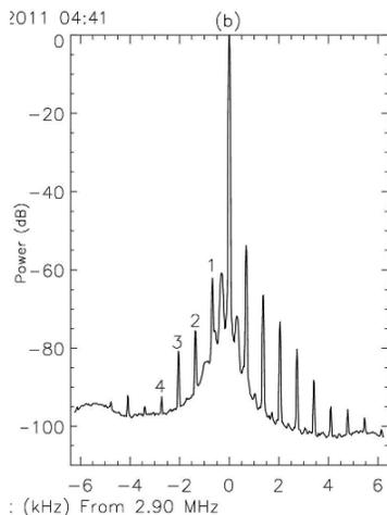
Figure 4 ~ Stimulated Electromagnetic Emissions (SEE) are seen as narrow spectra adjacent to the transmit frequency. This spectral plot has been normalized with the transmit frequency 2.90 MHz ( $2f_{ce}$ ) at the center of the horizontal scale. Image adapted from [Workshop]
