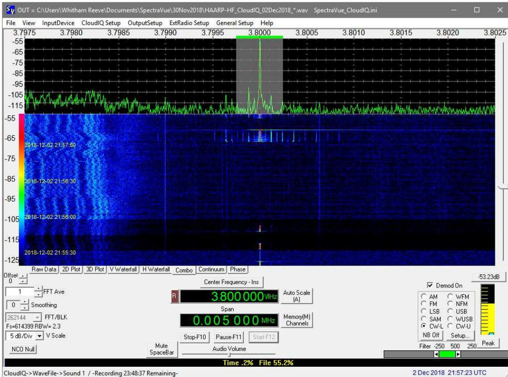
Cloud-IQ, 3.8 MHz, 5 kHz span, 2 December, 2157:23. Apparent powerline interference modulation of HAARP carrier. Note broad RFI to left.
