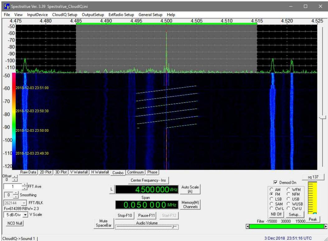
Cloud-IQ, 4.50 MHz, 50 kHz span, 3 December, 2351. FM sweep modulation. RFI is present to left and right of the HAARP transmitter frequency in the waterfall. HAARP settings 4.5 and 3.25 MHz.
