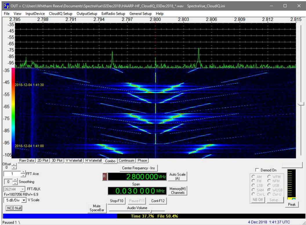
Cloud-IQ, 2.80 MHz, 30 kHz span, 4 December, 0141. HAARP setting 2.8 MHz. Chrip modulation.
