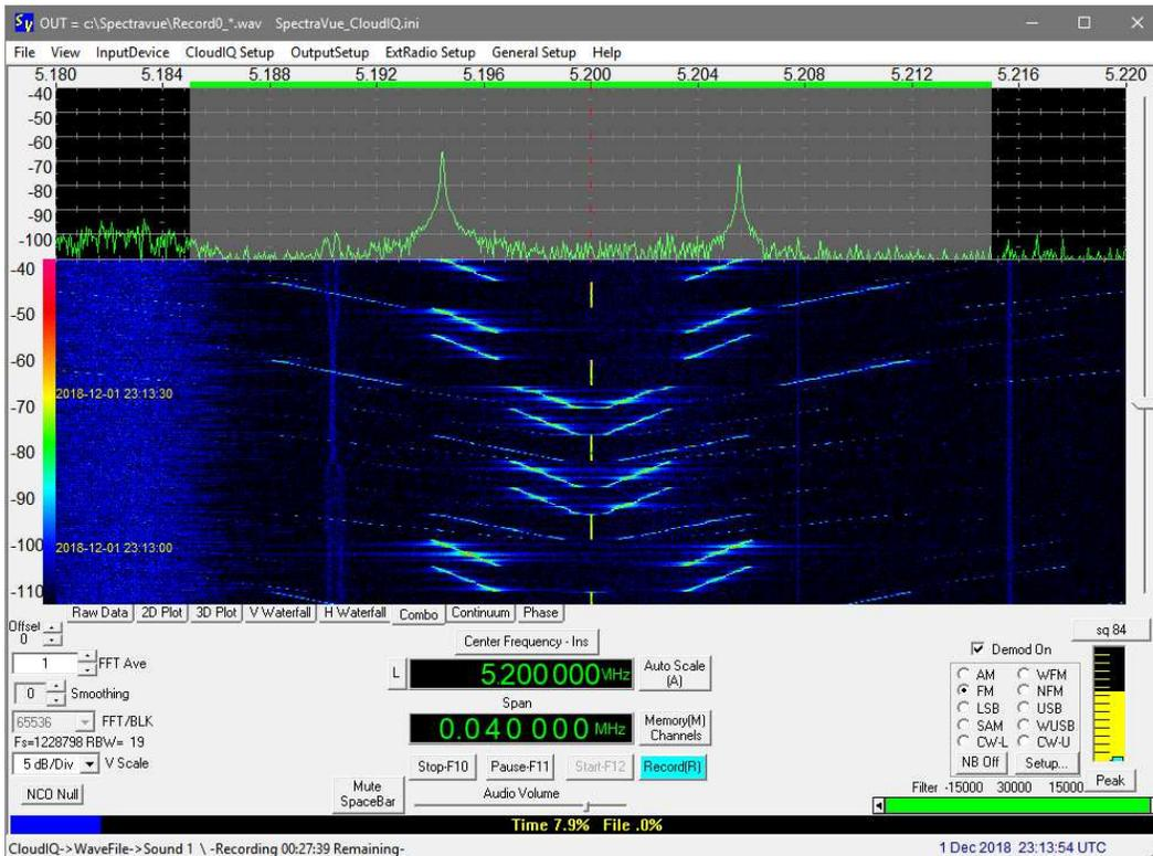
Cloud-IQ, 5.2 MHz, 400 kHz span, 1 December, 2313. Chirp modulation.
