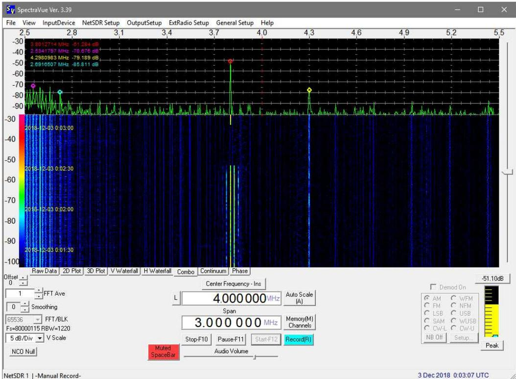
Cloud-IQ, 3.8 MHz, 3 MHz span, 3 December, 0003. Carrier near 4.3 MHz is weather fax transmitted by the Coast Guard station at Kodiak.
