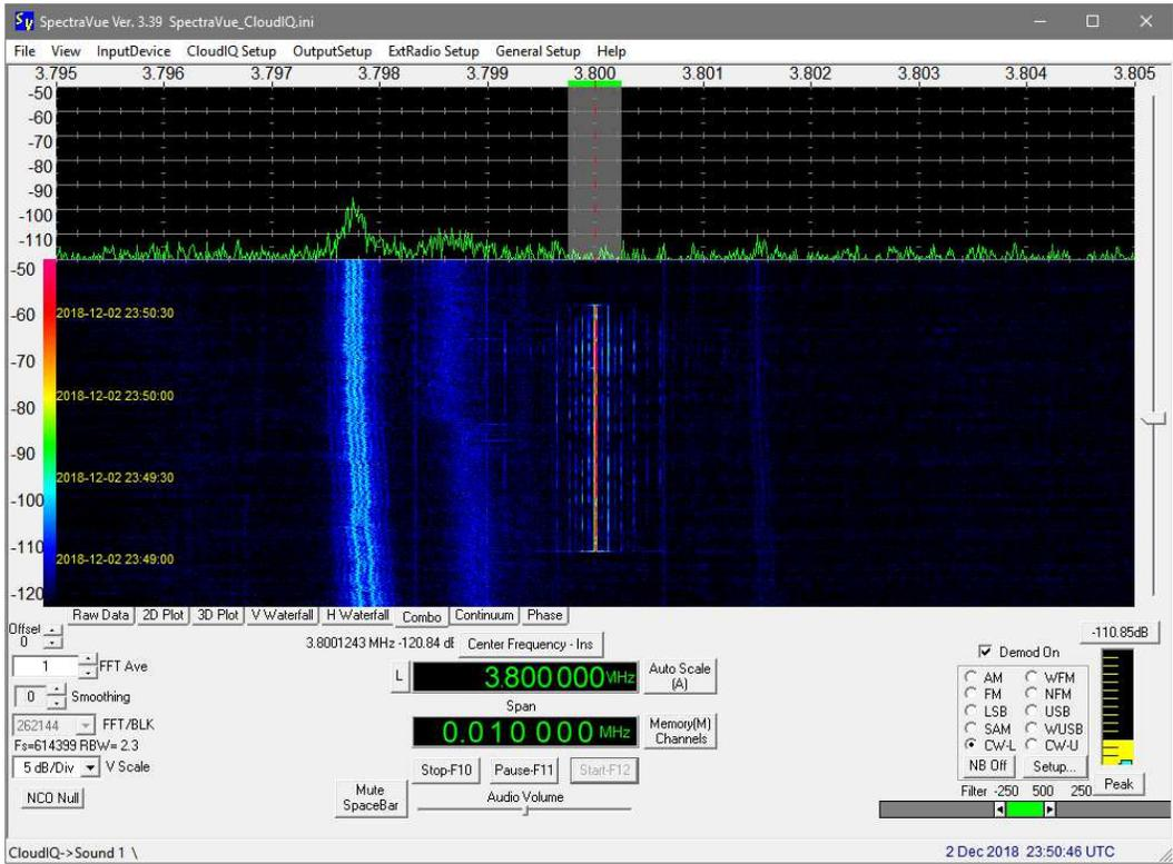
Cloud-IQ, 3.8 MHz, 1 kHz span, 2 December, 2350. Note drifting RFI between 3.797 and 3.798 MHz.
