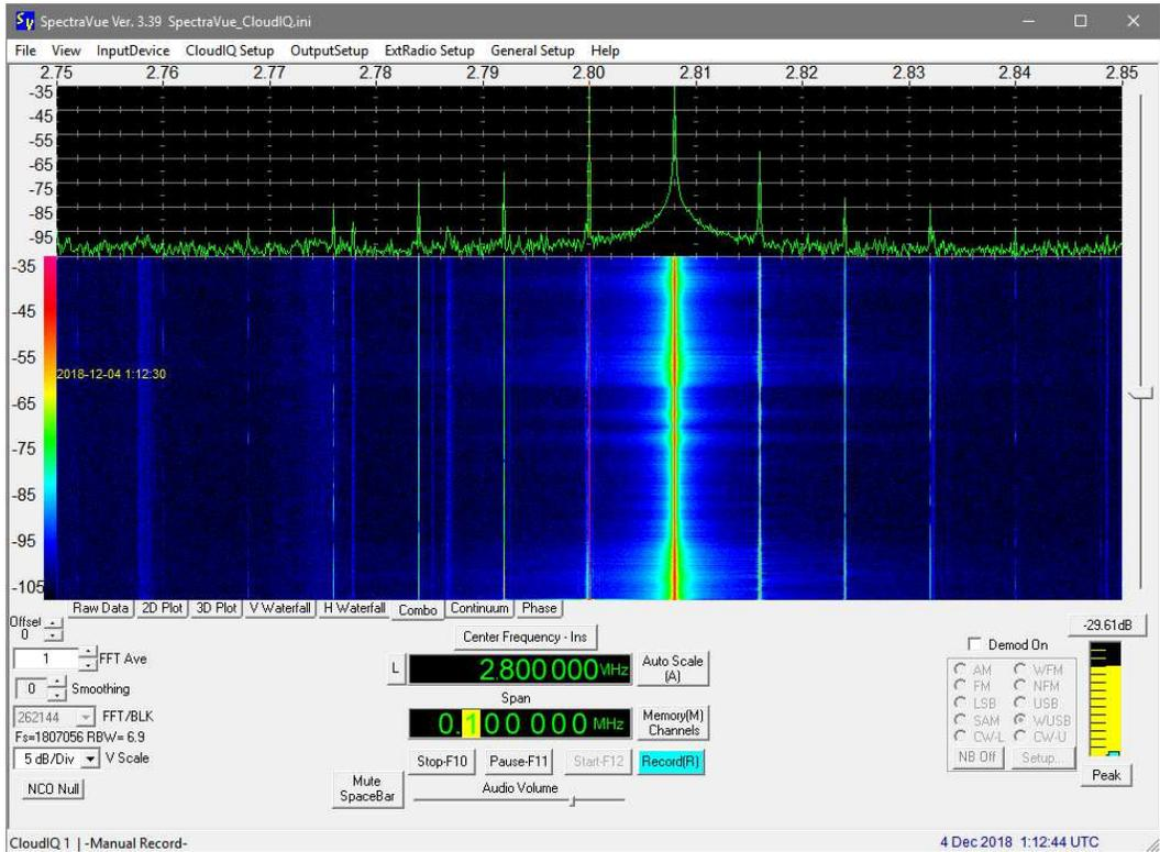
Cloud-IQ, 2.80 MHz, 100 kHz span, 4 December, 0112. HAARP setting 2.8 MHz. Multi-carrier with 8 kHz spacing. Carrier at 2.808 MHz much stronger for unknown reasons.
