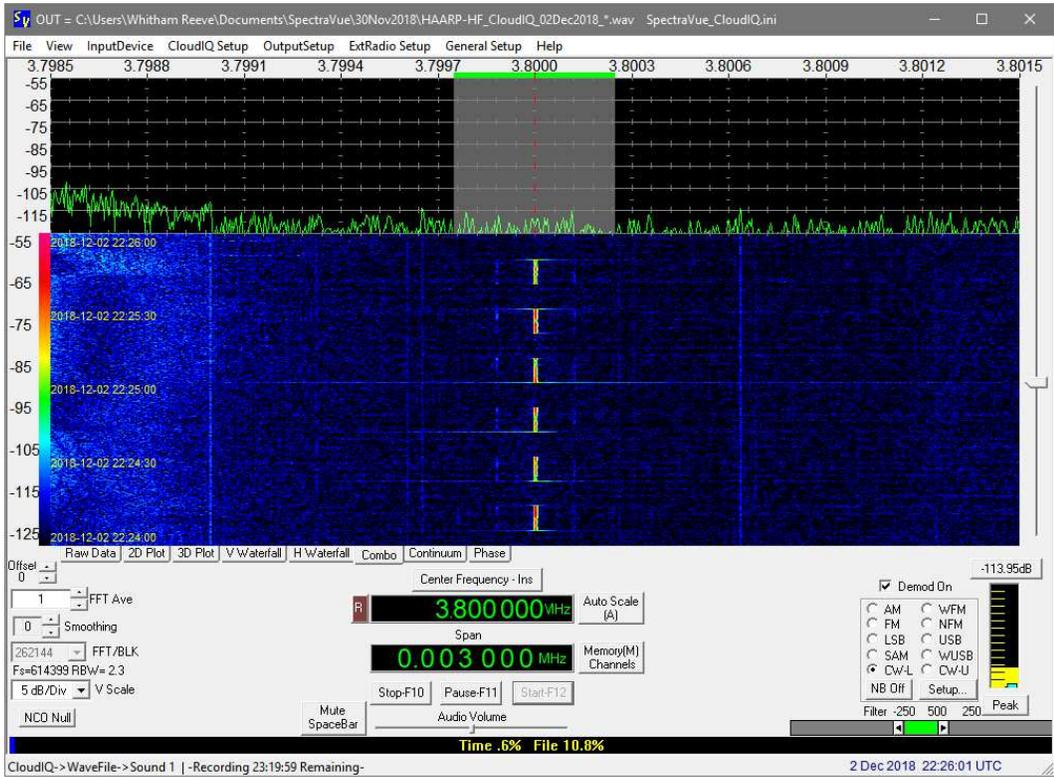
Cloud-IQ, 3.8 MHz, 3 kHz span, 2 December, 2226. Wideband radio frequency interference (RFI) can be seen on the left side of the spectrum and waterfall.
