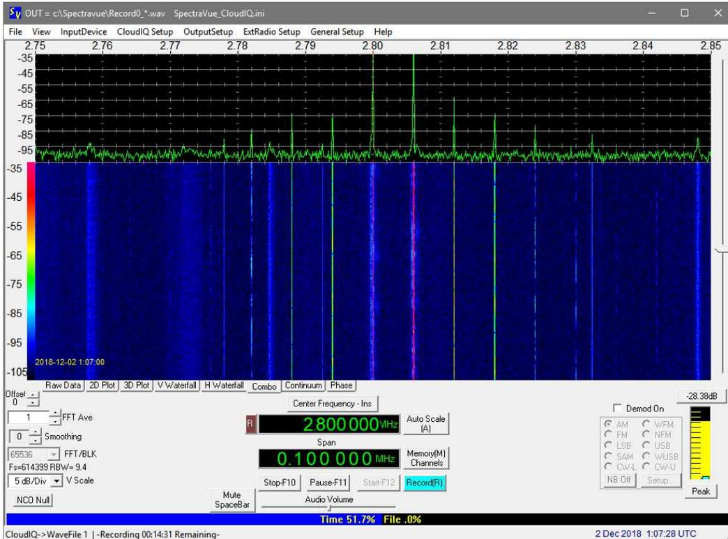
Cloud-IQ, 2.8 MHz, 100 kHz span, 2 December, 0107. Multi-carrier with 6 kHz spacing.
