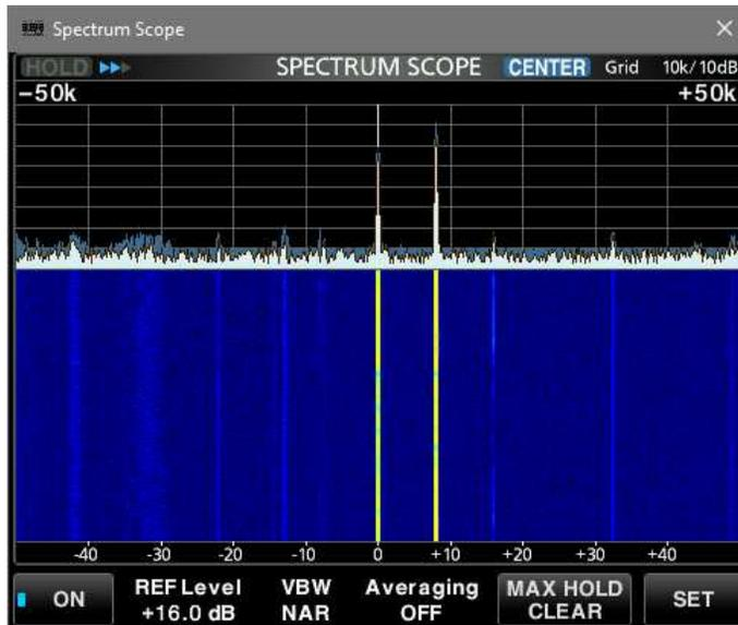
R-8600, 2.80 MHz, 100 kHz span, 4 December, 0127. HAARP setting 2.8 MHz. Second carrier at 2.808 MHz. See previous spectrogram.
