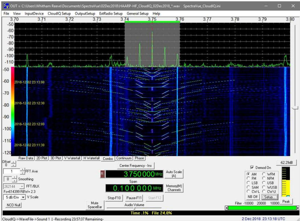
Cloud-IQ, 3.75 MHz, 100 kHz span, 2 December, 2313. Chirp modulation.
