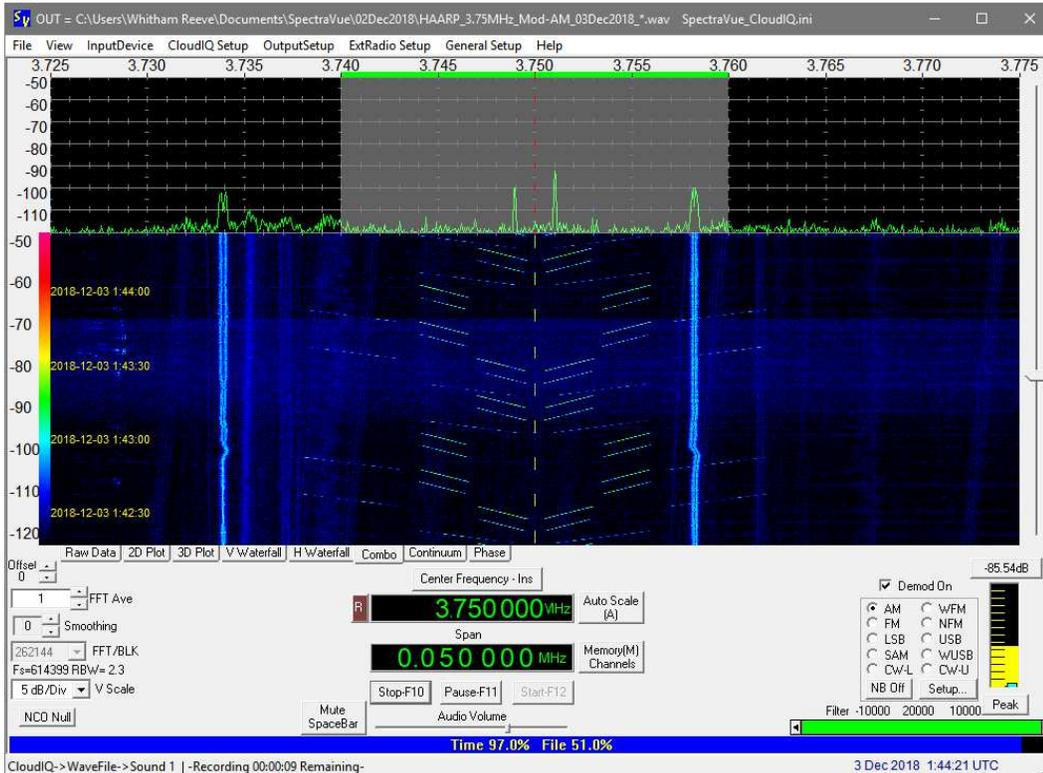
Cloud-IQ, 3.75 MHz, 50 kHz span, 3 December, 0144. Chirp modulation along with RFI (broad lines in waterfall).
