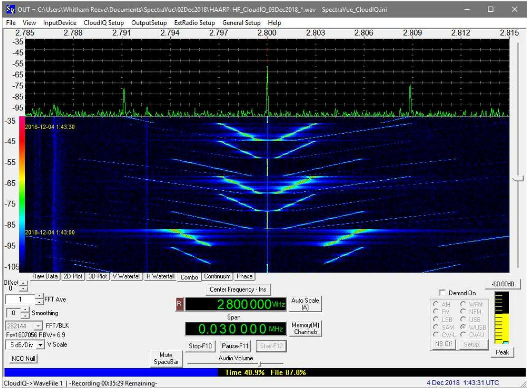
Cloud-IQ, 2.80 MHz, 30 kHz span, 4 December, 0143. HAARP setting 2.8 MHz. Chirp modulation.
