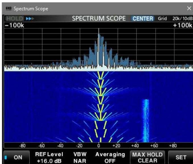
R-8600, 4.25 MHz, 200 kHz span, 1 December, 0028. Chirp modulation. RadioFax on 4.298 MHz to immediate right ended while waterfall in progress.
