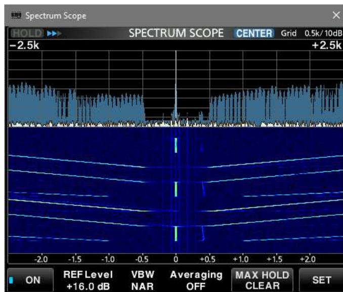
R-8600, 2.7 MHz, 5 kHz span, 1 December, 0028. Chirp modulation.
