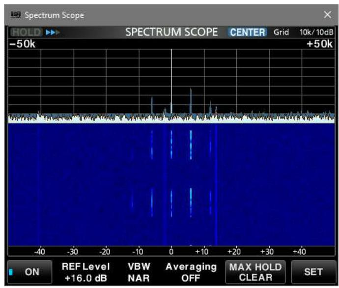
R-8600, 3.80 MHz, 100 kHz span, 2 December, 2223. Apparent multi-carrier transmission.
