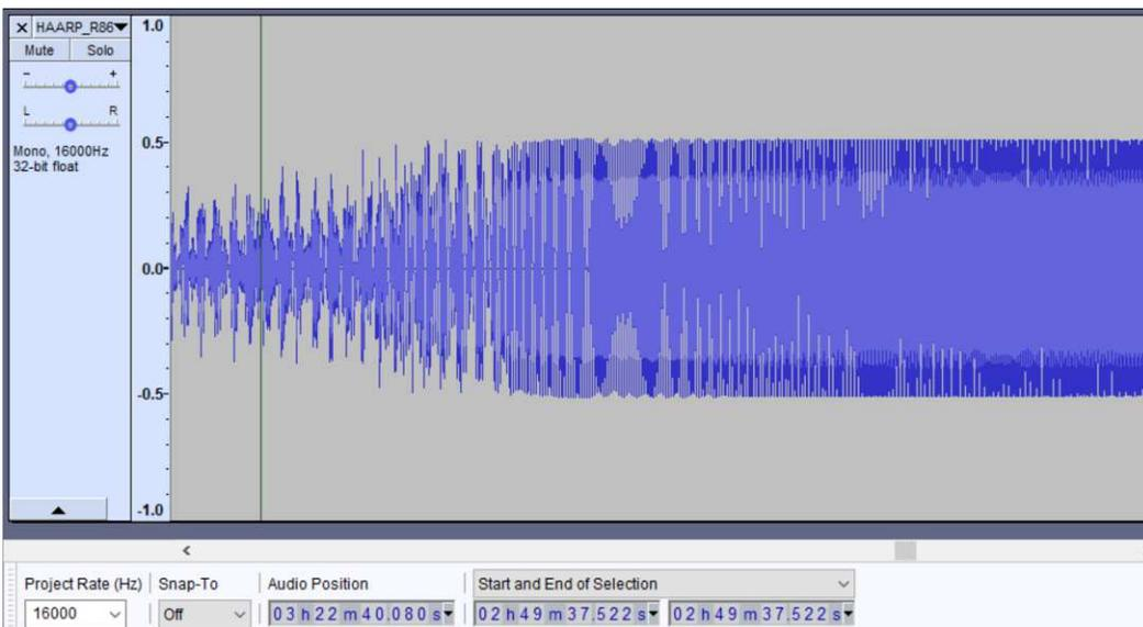
R-8600, Demodulated audio waveform corresponding approximately to the previous RF spectrogram on 1 December at 0027. The RF modulation far exceeded the audio passband of the receiver.
