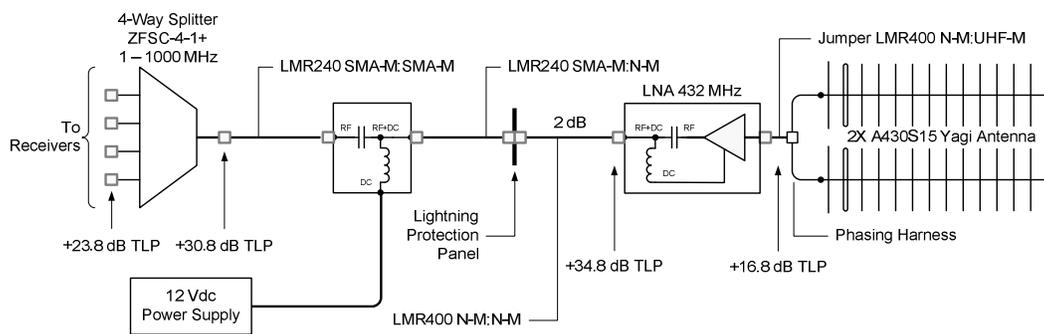
Figure 9 ~ Antenna system and low noise amplifier (right of protection panel) and bias-tee and splitter (left) used for the 432 MHz mixing and scattering experiment. The splitter allowed up to four receivers to be connected; both the NetSDR and R-8600 were temporarily repurposed from the HF observations and used for the UHF observations. Also shown are the estimated transmission level points (TLP) at locations along the transmission path. Image © 2019 W. Reeve
