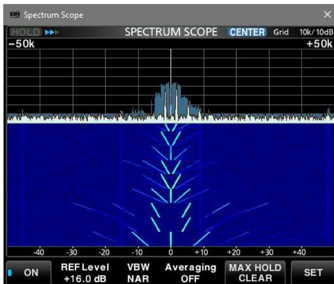
R-8600, 3.8 MHz, 100 kHz span, 2 December, 2330. Chirp modulation.
