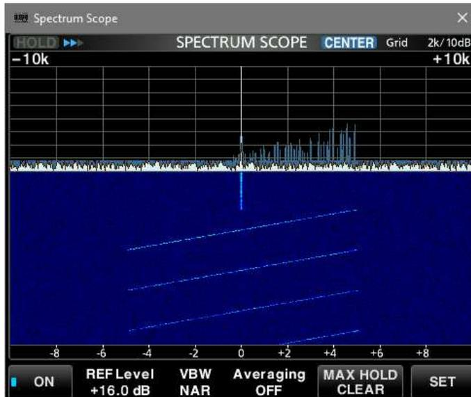
R-8600, 4.50 MHz, 20 kHz span, 4 December, 0004. Similar to previous except narrower span.
