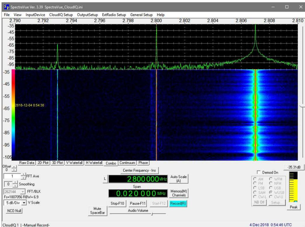
Cloud-IQ, 2.80 MHz, 20 kHz span, 4 December, 0054. Note carriers at  $2.8000 \pm 0.007$  MHz with stronger reception at 2.807 MHz weaker reception at 2.793 MHz. HAARP setting 2.8 MHz.
