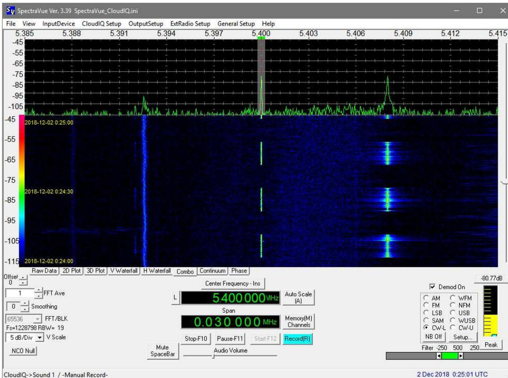
Cloud-IQ, 5.4 MHz, 30 kHz span, 2 December, 0025. A much stronger carrier at 5.408 MHz is visible but it may be signal processing artifact.
