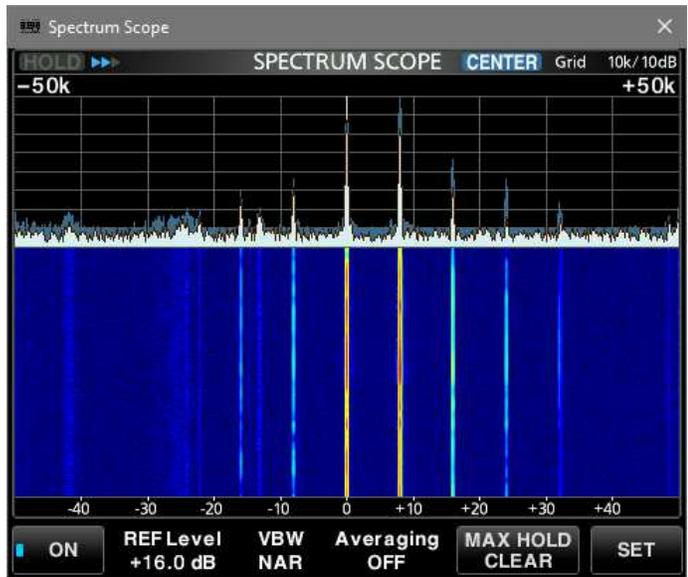
R-8600, 2.80 MHz, 100 kHz span, 4 December, 0112. HAARP setting 2.8 MHz. See previous spectrogram.
