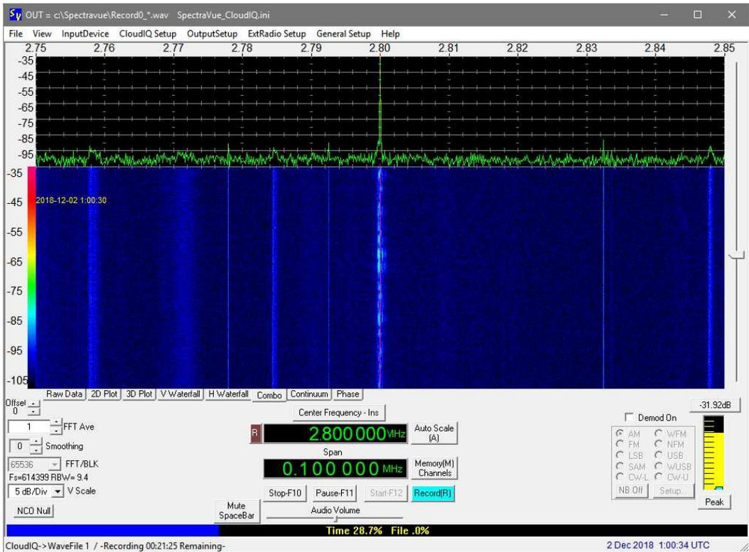
Cloud-IQ, 2.8 MHz, 100 kHz span, 2 December, 0100. Note variable intensity of received carrier.
