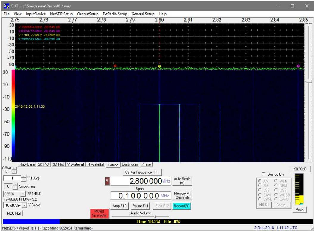
NetSDR, 2.8 MHz, 100 KHz span, 2 December, 0111. Multi-carrier with 6 kHz spacing off at 0111:30.
