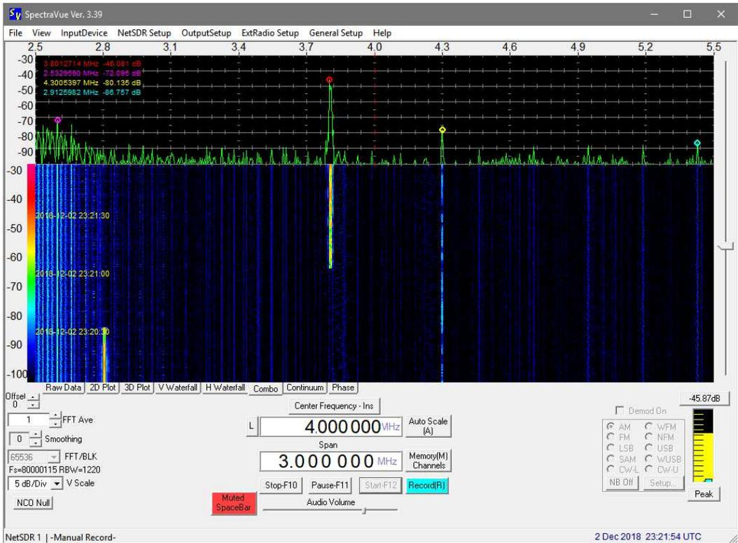
NetSDR, 3.8 MHz, 3 MHz span, 2 December, 2321. Note HAARP transmitter frequency  $f_0 = 3.8$  MHz. The spectra at about 4.3 MHz is the weather fax at the Kodiak Coast Guard station.
