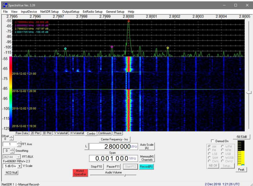
NetSDR, 2.8 MHz, 1 kHz span, 2 December, 0121. Some waterfall lines are RFI and some are multi-carriers around the primary.
