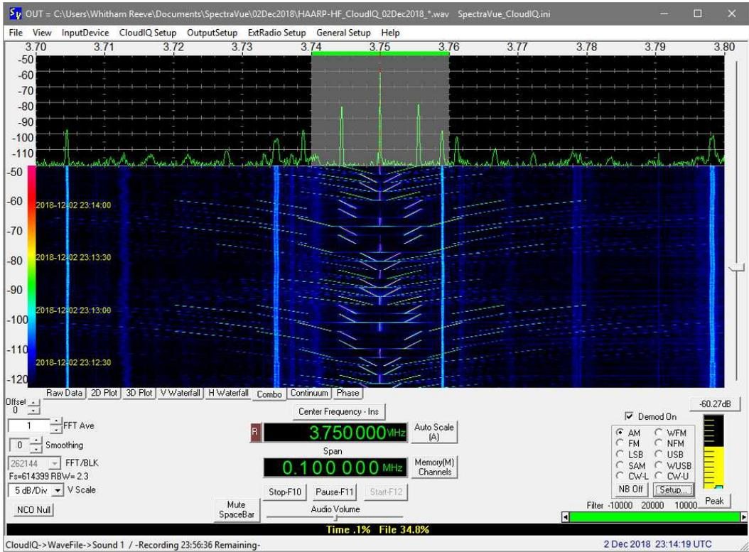
Cloud-IQ, 3.75 MHz, 100 kHz span, 2 December, 2314. Chirp modulation.
