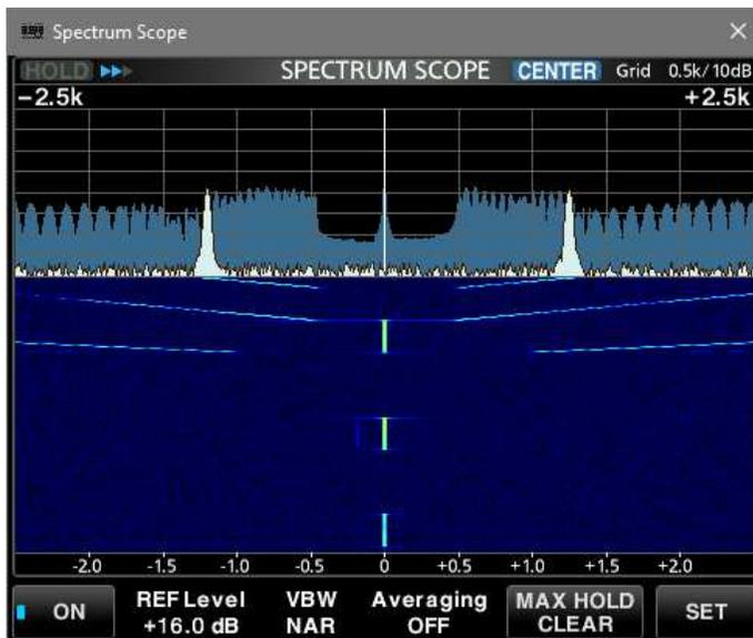
R-8600, 3.25 MHz, 5 kHz span, 30 November, 0200. Chirp modulation. Note the frequency of the current trace is indicated in the spectrum display by the white spikes.
