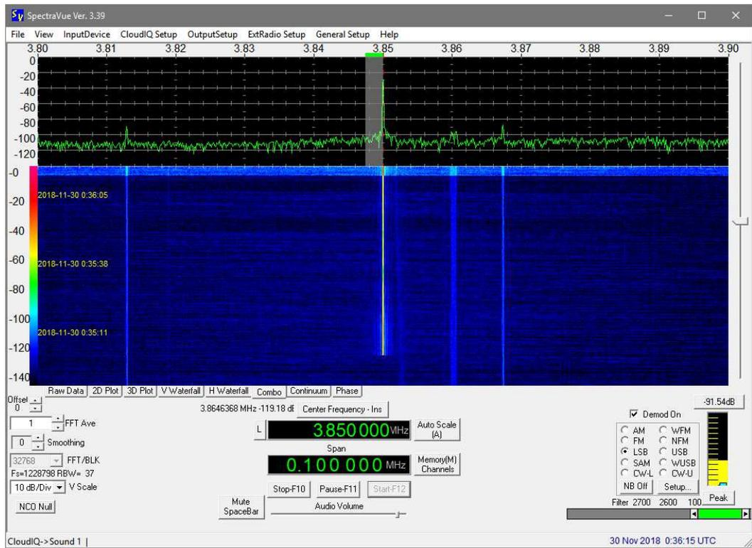
Cloud-IQ, 3.85 MHz, 100 kHz span, 30 November, 0036. Some persistent RFI is visible above and below the center frequency.
