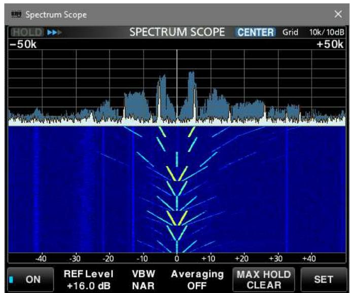
R-8600, 2.80 MHz, 100 kHz span, 4 December, 0141. HAARP setting 2.8 MHz. Chrip modulation.
