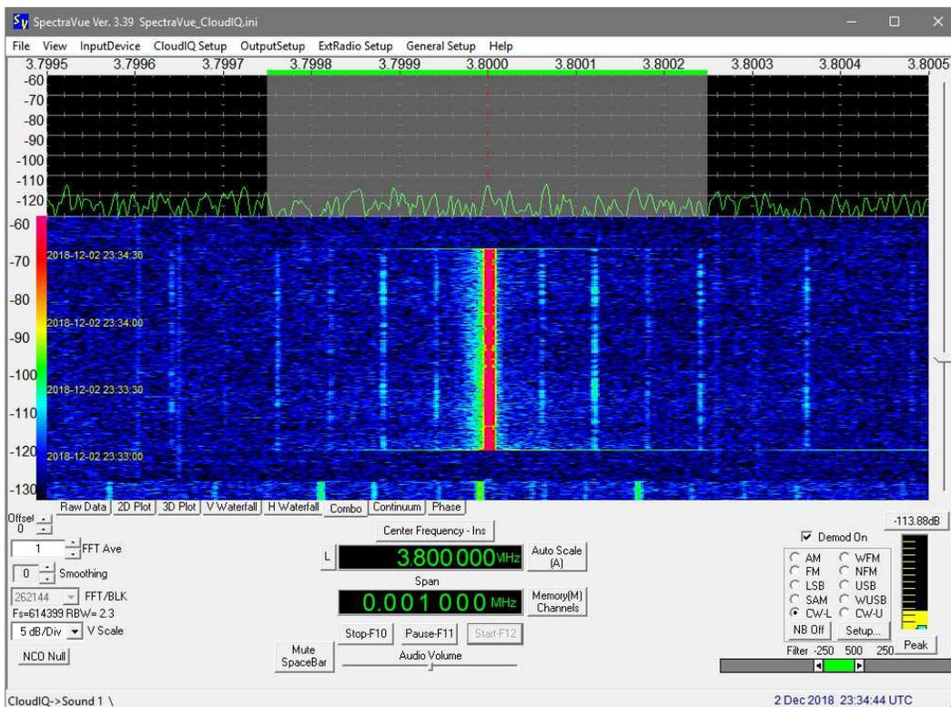
Cloud-IQ, 3.8 MHz, 1 kHz span, 2 December, 2334. Carriers with 60 Hz spacing may be inadvertent modulation of the primary carrier by the power system.
