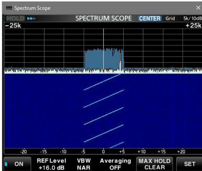
R-8600, 4.50 MHz, 50 kHz span, 4 December, 0004. FM sweep modulation.
