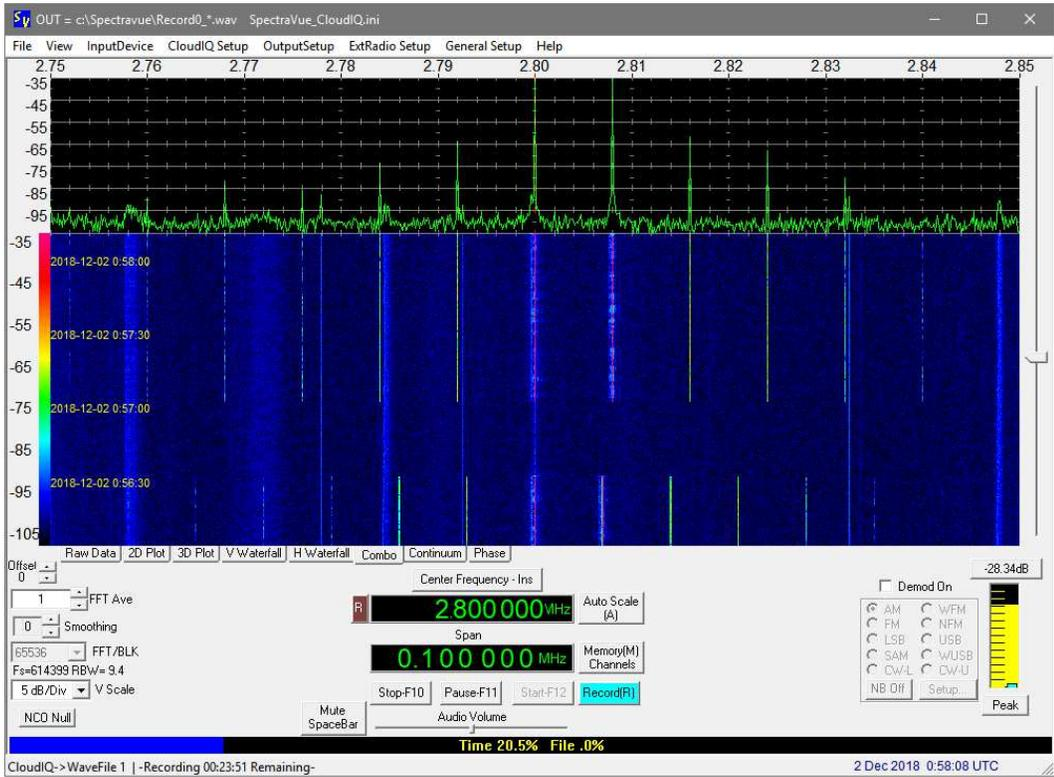
Cloud-IQ, 2.8 MHz, 100 kHz span, 2 December, 0058. Multi-carrier with 8 kHz spacing. Note shift in carrier spacing from 7 kHz spacing at 0056:30 and variable received power level at the various carrier frequencies. Some RFI also is visible.
