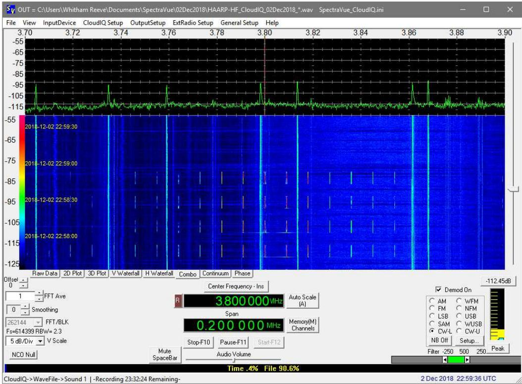
Cloud-IQ, 3.8 MHz, 200 kHz span, 2 December, 2259. Multi-carrier transmissions ended at 2259:00. The thicker lines in the waterfall are RFI.
