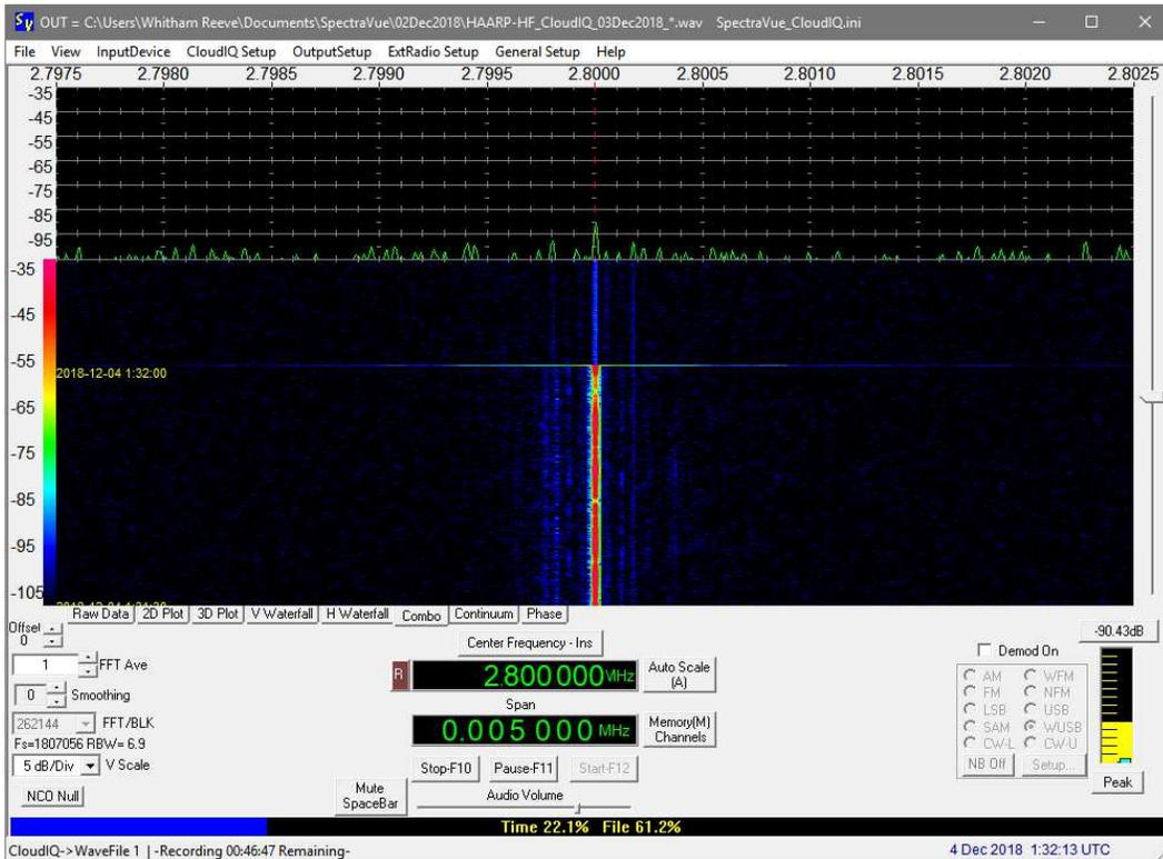
Cloud-IQ, 2.80 MHz, 5 kHz span, 4 December, 0132. HAARP setting 2.8 MHz. The horizontal line at end of transmission at 0132:00 is an artifact of signal processing.
