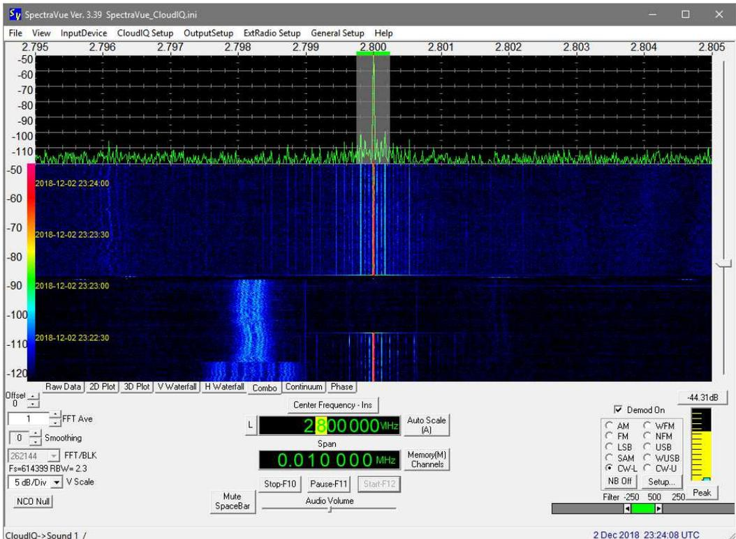
Cloud-IQ, 2.8 MHz, 10 kHz span, 2 December, 2324:08. Possible Stimulated Electromagnetic Emissions (SEE) around the HAARP carrier.
