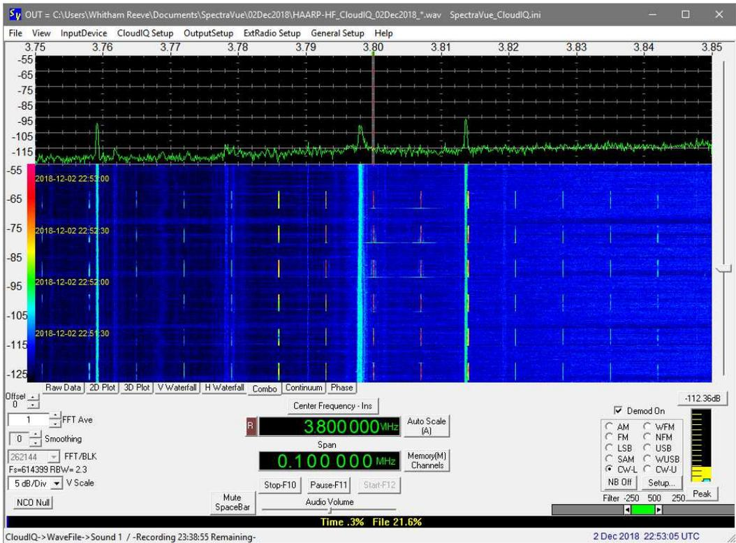
Cloud-IQ, 3.8 MHz, 100 kHz span, 2 December, 2253. Multi-carrier transmissions with 7 kHz spacing. The thicker lines in the waterfall are RFI.
