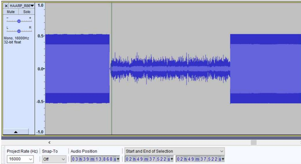
R8600 demodulated audio waveform corresponding to previous RF spectrogram on 1 December from 0043:30 to 0045:30. Note complete noise dropout immediately at the end of first section for about 1 s followed by recovery of background noise (cursor position). This probably was caused by the AGC function in the R-8600.
