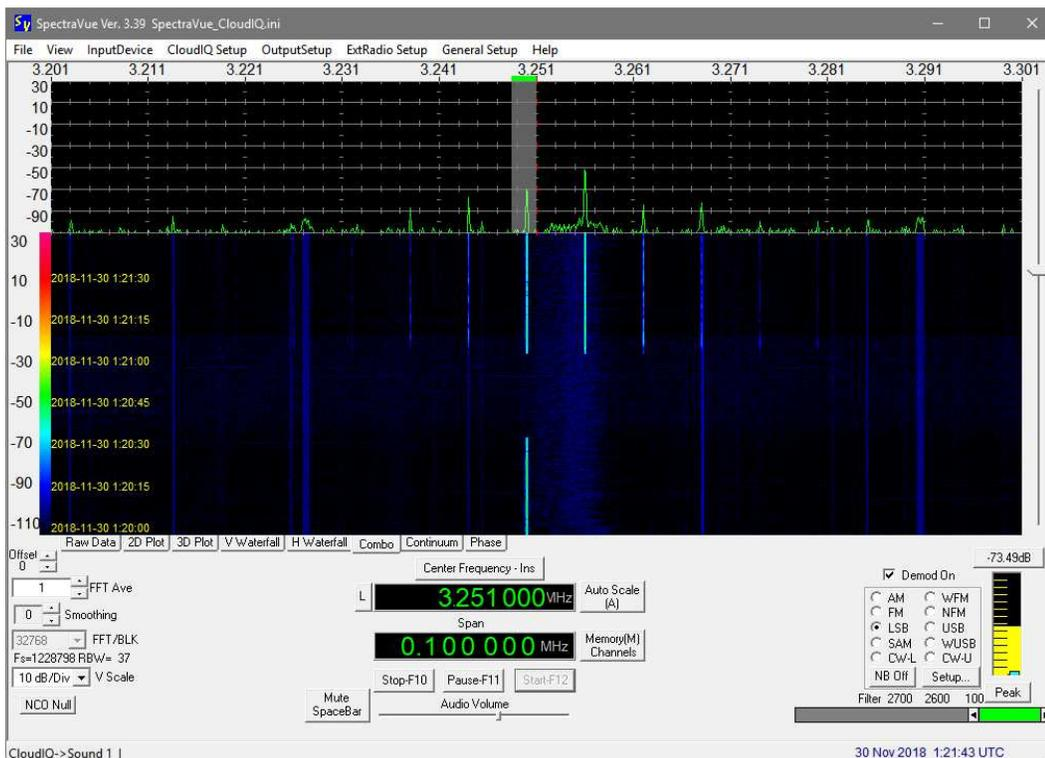
Cloud-IQ, 3.251 MHz, 100kHz span, 30 November, 0121. The strongest carrier of this multi-carrier transmission appears at 3.256 MHz with three additional carriers above and three carriers below. The carrier spacing is 6 kHz. The previous On sequence had only one carrier at 3.250 MHz.
