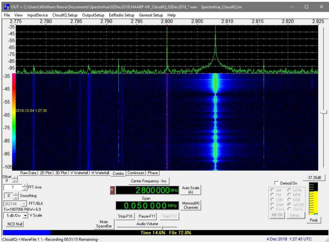
Cloud-IQ, 2.80 MHz, 50 kHz span, 4 December, 0127. HAARP setting 2.8 MHz. Why carrier at 2.808 MHz is so much stronger is unknown.
