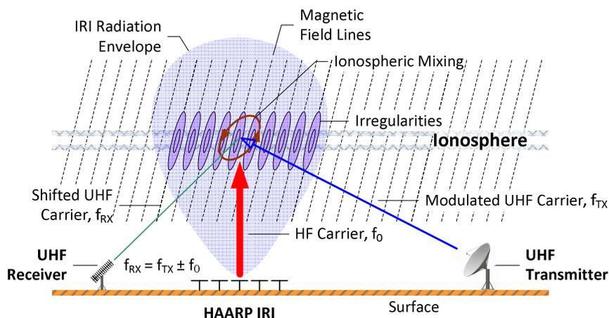
Figure 2 ~ Frequency mixing and scattering experiment schematic. The HAARP IRI produces electron density striations (irregularities) in the ionosphere. Frequency mixing can take place such that a signal transmitted toward the spot above HAARP is mixed with the HAARP transmitter frequency to produce sum and difference frequencies that are scattered. The winter 2018 campaign included attempts by radio amateurs to detect this phenomenon. Image adapted from {DTIC}
