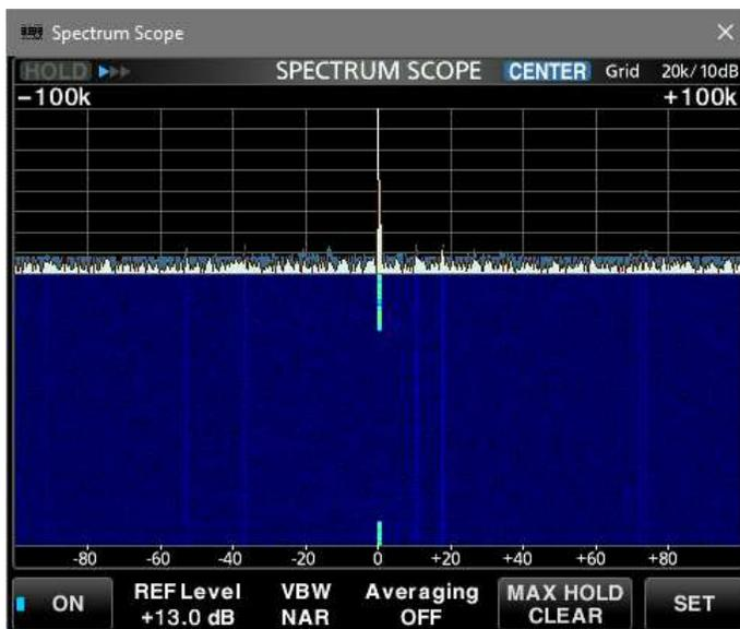
R-8600, 3.85 MHz, 200 kHz span, 30 November, 0036. The RFI clearly seen in the previous waterfall is less obvious in this one.
