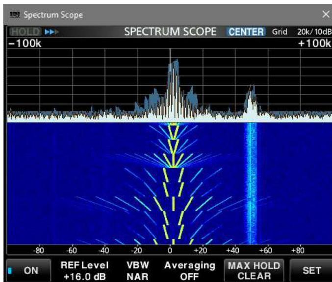
R-8600, 4.25 MHz, 200 kHz span, 1 December, 0027. Chirp modulation. RadioFax on 4.298 MHz to immediate right.
