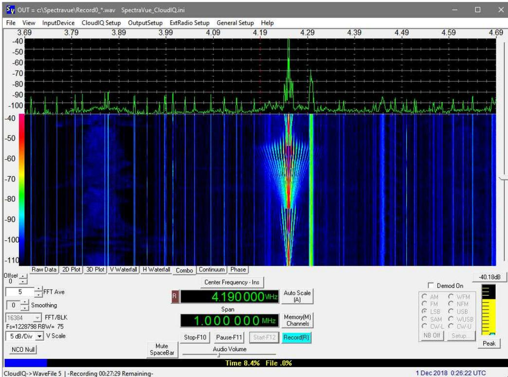
Cloud-IQ, 4.19 MHz, 1 MHz span, 1 December, 0026. Chirp modulation. Chirp modulation. RadioFax on 4.298 MHz to immediate right.
