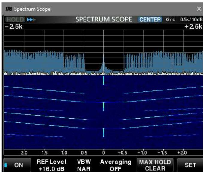
R-8600, 3.25 MHz, 5 kHz span, 30 November, 0200. Chirp modulation as shown previously except the span shown here is narrower. Note the display persistence of previous sweeps in the spectrum display.
