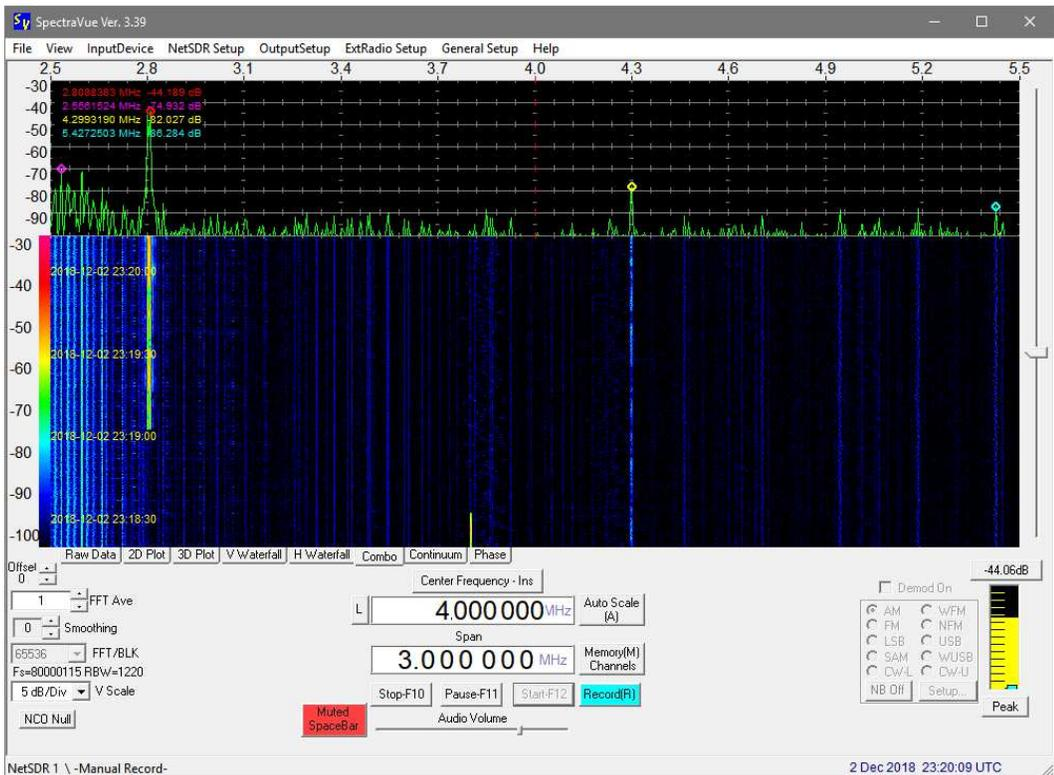
NetSDR, 4.0 MHz, 3 MHz span, 2 December, 2320. Note HAARP transmitter frequency  $f_0 = 2.8$  MHz. The spectra at about 4.3 MHz is the weather fax (RadioFax) transmitted by the Kodiak Coast Guard station.
