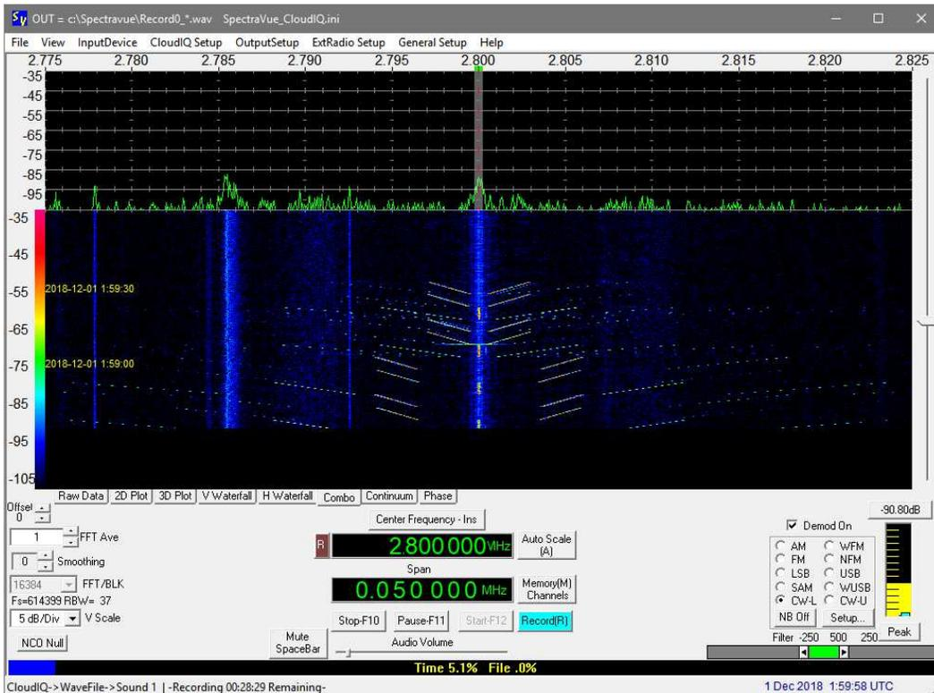
Cloud-IQ, 2.80 MHz, 50 kHz span, 1 December, 0159. Chirp modulation.
