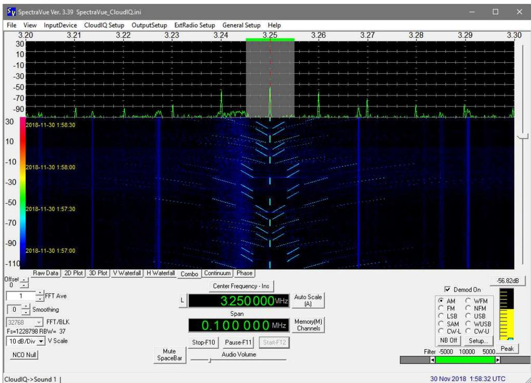
Cloud-IQ, 3.25 MHz, 100 kHz span, 30 November, 0158. Chirp modulation.
