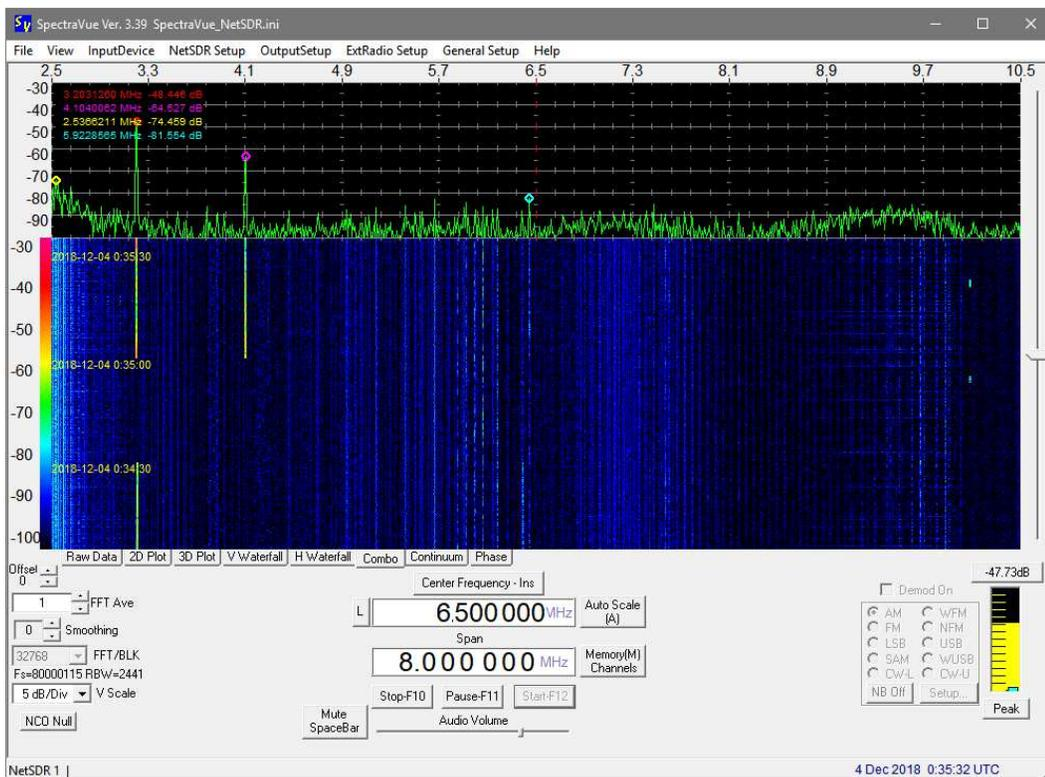
NetSDR, 6.5 MHz, 4 December, 0035. Note that the HAARP transmitter frequency  $f_0 = 3.2$  MHz. Unknown signal at 4.1 MHz.
