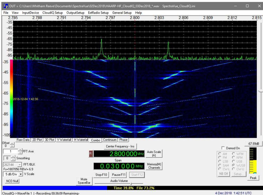
Cloud-IQ, 2.80 MHz, 30 kHz span, 4 December, 0142. HAARP setting 2.8 MHz. Chirp modulation.
