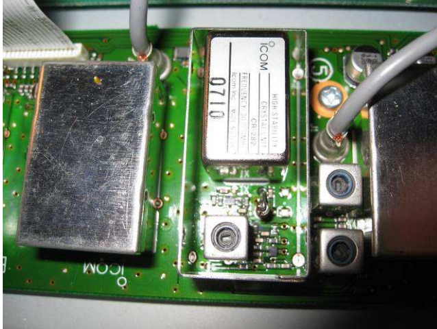
Figure 2 – New CR-282 Oven Controlled Crystal (top center of picture) installed in the oscillator fence after removal of the original CR-275A crystal. The CR-282 provides significantly higher frequency stability over a wider temperature range than the plain crystal it replaces and is recommended for mobile installations and fixed installations that require higher stability. The oscillator frequency is adjusted with L2, which is the variable inductor can below the new crystal.
