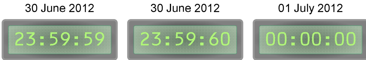
Fig. 3 ~ A leap second will be inserted to retard UTC at the end of June 2012. The clock shown here is conceptual and based on the UTC time scale, so it will occur at different local times depending on the user's time zone. It is unlikely that any real clock will show the digits "60" in the seconds field as shown here.
