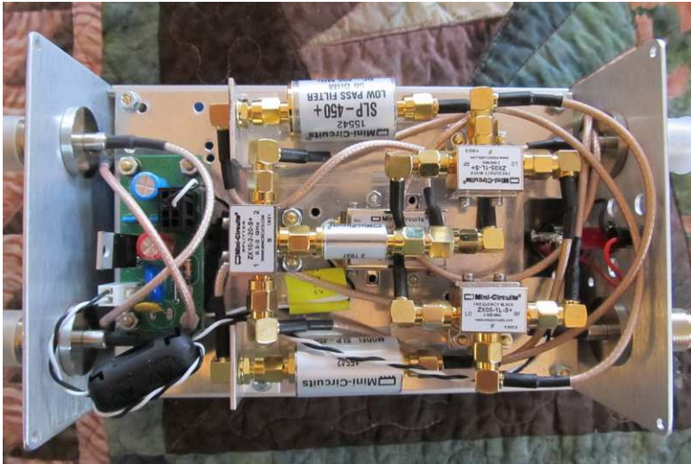
Figure 16.c ~ Final prototype of the experimental up-converter built with two aluminum chassis layers. The enclosure is the same as used with the Callisto instrument. The bottom chassis (not visible) holds two FL590 filters and has space for two input amplifiers (not installed here because amplifiers are not needed with the LWA antenna). The upper chassis holds two shielded mixers, an oscillator, splitter and three filters for the oscillator and IF outputs. Two identical converters are built in one enclosure and share the oscillator. This proved to be a good design and will be manufactured after selecting the LO frequency (see text). Image © 2020 W. Reeve
