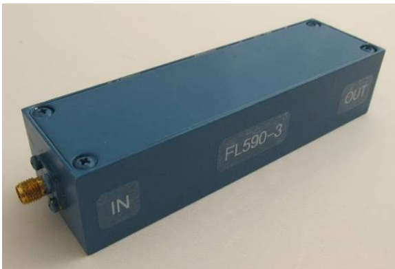
Figure 1 ~ FL590 filter ready for use. The filter components are housed in a milled aluminum enclosure with an SMA-female connector on each end. The enclosure is repurposed from an AEL bandpass filter. Dimensions are 120 L x 35 W x 27 H mm. Image © 2020 W. Reeve
