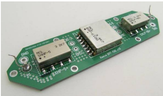
Figure 2 ~ Three shielded, surface mounted, lumped element filters installed on an in-house designed printed circuit board. From left-to-right, Mini-Circuits SXHP-5+ highpass filter, BSF-C100+ bandstop filter and SXLP-90+ lowpass filter. Tinned copper pigtail terminals can be seen at each end for soldering to the SMA connectors mounted on the enclosure. The PCB dimensions are 115 L x 30 W x 8 H mm, including the filter modules. Image © 2020 W. Reeve
