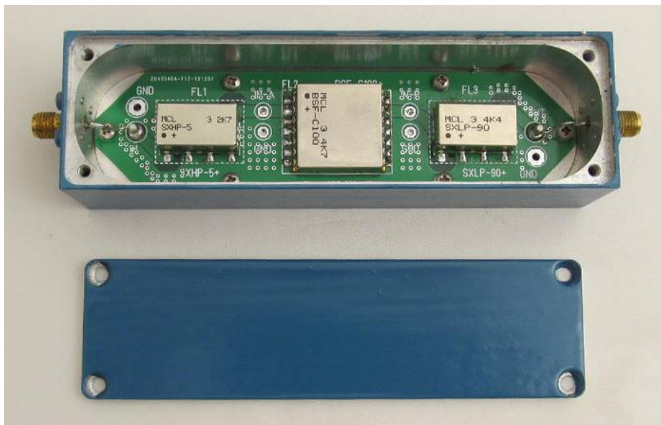
Figure 5 ~ Milled aluminum enclosure with the finished printed circuit board installed. The PCB is fastened with six 3-48 machine screws and lock washers, which bond the PCB ground reference plane to the enclosure. Image © 2020 W. Reeve
