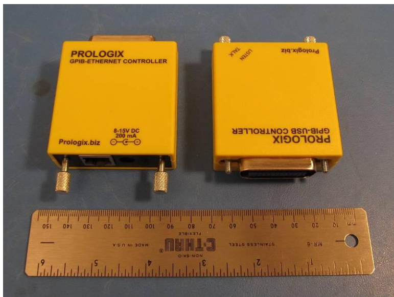
Figure 4 ~ Ethernet (left) and USB controllers for the IEE-488/GPIB interface. The new price for the USB controller is about US$150 and for the Ethernet controller is about US$200, but both occasionally appear online at slightly reduced prices. The Ethernet controller requires an external ac power adapter (not shown), and the USB controller is powered through the USB port.
