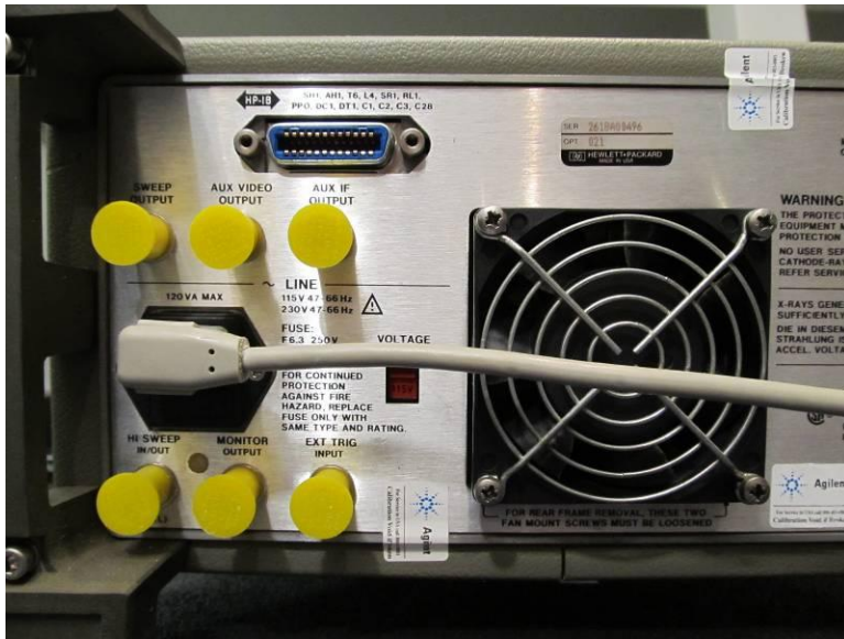
Figure 2 ~ IEEE-488 interface connector on the HP 8590A rear panel at top-left marked “HP-IB”. The interface controllers described in this article can be mounted directly on the test set connector or connected through an IEEE-488/GPIB cable.
