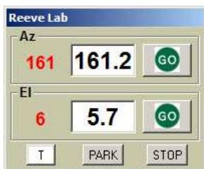
Figure 5 ~ PstRotator user interface compact view. Only the azimuth and elevation are shown.
