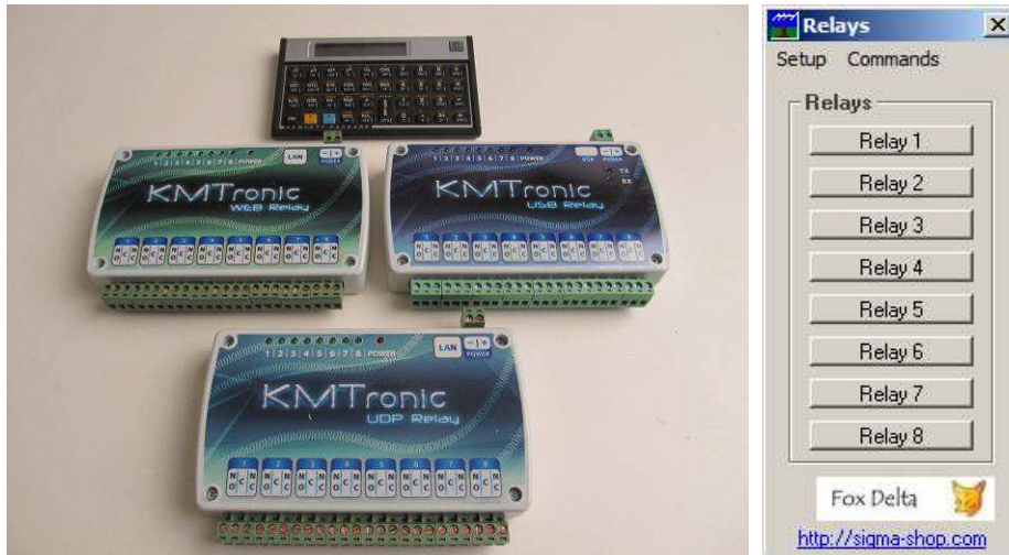
Figure 4 ~ PstRotatorAz can be used to remotely or locally control relays used for power control or other station control functions. The relay units shown here are KMTronic units compared to an HP calculator. The KMTronic units have 8 relays, each with Form C contacts (Normally Open, Normally Closed and Common). PstRotator does not yet have the relay control feature. (Image left © 2015 W. Reeve)
