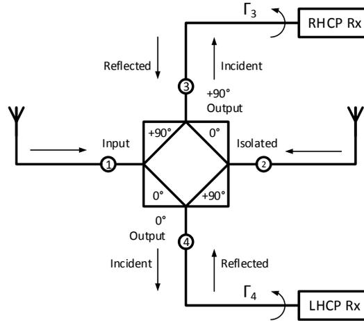
Figure 6 ~ Block diagram showing reflections at the coupler output ports 3 and 4. The waveforms from the two antennas are coupled and delayed as described in the previous section. A portion is reflected at each output port according to the reflection coefficients  $\Gamma_3$  and  $\Gamma_4$ . (Image © 2014 W. Reeve)
