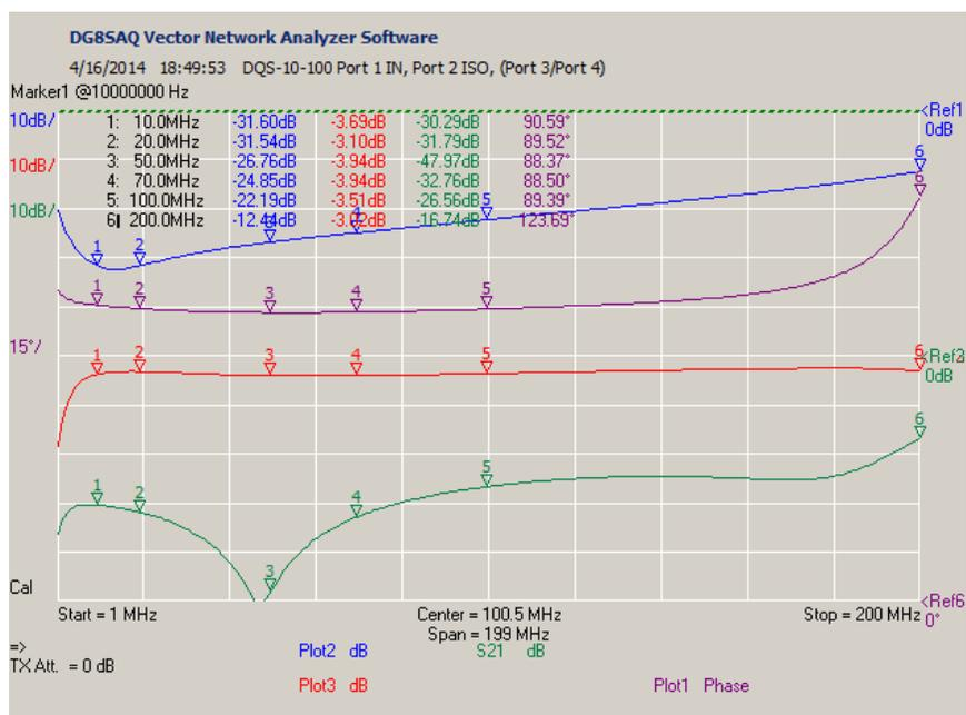
Figure 3 ~ Measurements from 1 to 200 MHz of the Synergy DQK-10-100S coupler showing the nominal 3 dB coupling loss (s-parameter S21, red trace) between ports 1 and 4, return loss (-S11, blue) of port 1, isolation (S21, green) of port 2 from port and phase difference between ports 3 and 4 (°, violet). The phase difference plot is the ratio [S21(port1 to port 4)/S21(port 1 to port 3)]. The coupling loss between
