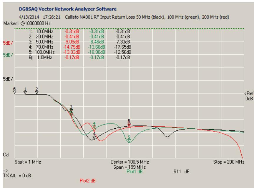
Figure 7 ~ Measured Callisto RF input return loss (–s11 parameter) while tuned to 50 MHz (black), 100 MHz (green) and 200 MHz (red). The marker table at upper-left indicates measured data at various frequencies. In the frequency band 10 to 100 MHz, the return loss varies from approximately 0 dB to 18 dB but typically  $RL > 10$  dB corresponding to a reflection coefficient < 0.316.
