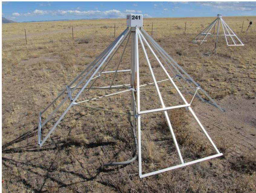
Figure 1 ~ Long Wavelength Array crossed-dipole antenna. The antenna consists of two independent tied-fork dipoles with their vertical planes perpendicular to each other. Each blade (or wing) is sloped 45° to improve response to radio waves whose plane of polarization is not aligned with the antenna axis. The horizontal components are fiberglass rod braces. The frequency range of the LWA antenna is approximately 10 to 90 MHz. (Image © 2014 W. Reeve)
