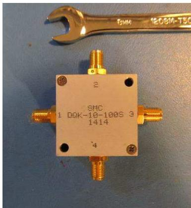
Figure 2 ~ Quadrature coupler conceptual schematic (left). The labels shown in the schematic correspond to the Synergy DQK-10-100S coupler (right) shown with an 8 mm wrench. Device dimensions are 1.25 in square x 0.75 in high and frequency range is 10 to 100 MHz. It is equipped with SMA-F connectors. (Images © 2014 W. Reeve)
