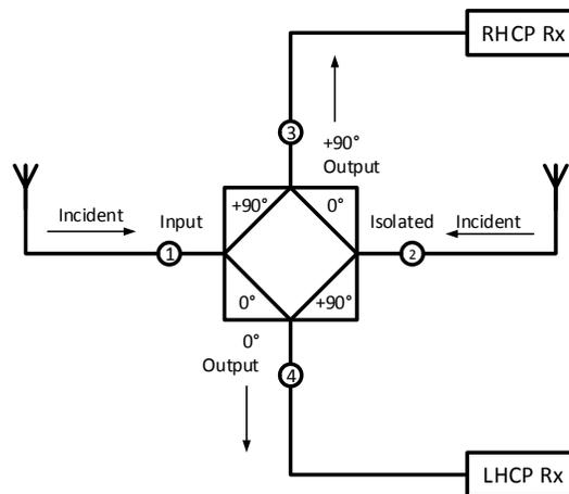
Figure 5 ~ Simplified block diagram of the quadrature coupler application showing port nomenclature. The designations for the two receivers, RHCP Rx and LHCP Rx, are based on the signal analysis. (Image © 2014 W. Reeve)
