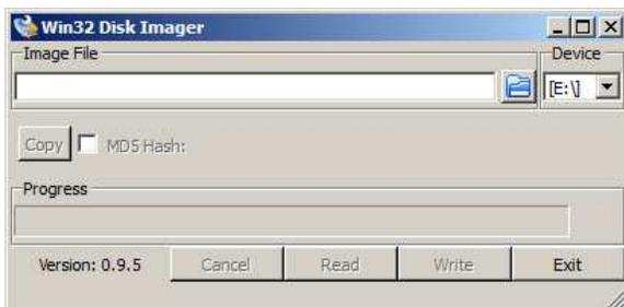
The drive letter for the memory card is shown in the Device field in upper-right. If you have more than one USB memory device plugged into the PC, select the letter corresponding to your memory card (drive letter E: in example above).
