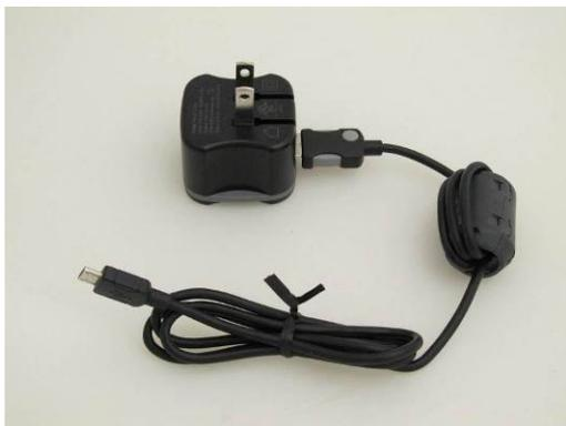
AC wall power adapter rated 12 W at 5 Vdc with North American ac input plug. One or more clamshell ferrite beads on the dc power lead may help reduce radio frequency interference from the switch-mode power supply. This image shows one bead on the right with three windings of the power lead. The Raspberry Pi uses a micro-USB connector for power. (Image © 2014 W. Reeve)
