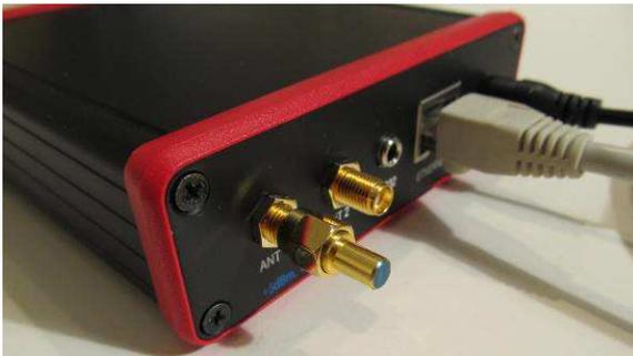
Figure 1-3.a ~ A 50 ohm SMA-M termination is connected to the ANT 1 RF input of an RFSpace Cloud-IQ SDR receiver (termination is in lower-middle of image). The other connections are an Ethernet LAN cable and 5 Vdc power input cable. For the measurements in this paper, the associated SpectraVue software collects the output data from the receiver over the LAN and computes, displays and stores the continuum power within the preset frequency span, typically 10 or 20 MHz. Image © 2016 W. Reeve
