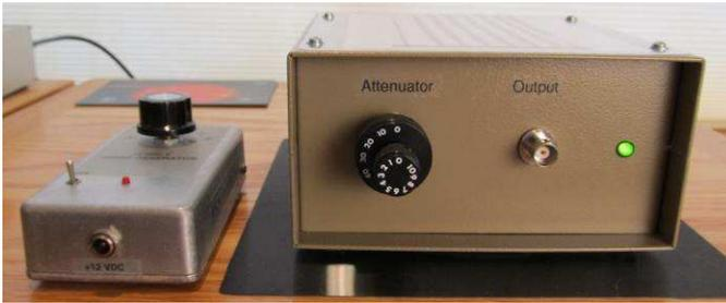
Figure 2-1 ~ Noise generators RF-2050S (left) and HOT-1 (right). These units are designed for HF and low VHF amateur radio astronomy applications and include attenuators to adjust the output noise temperature. For scale, the width of the HOT-1 is about 150 mm.
