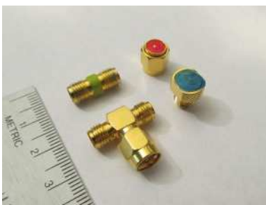
Figure 5 ~ Calibration kit used with the VNWA-3E, consisting of Short, Open, Load and Thru components that use SMA connectors. The Open and Thru are the same barrel connector shown upper-left. The slightly different reference plane locations of the Open and Short affect the calibration so a phase delay is manually entered into the software configuration to compensate. The Short and Load components are mechanically similar and have been color-coded for easy identification (red for the short and blue for the load). A coaxial tee-junction connector – used for the T-Check accuracy test described later – is shown lower-left.
