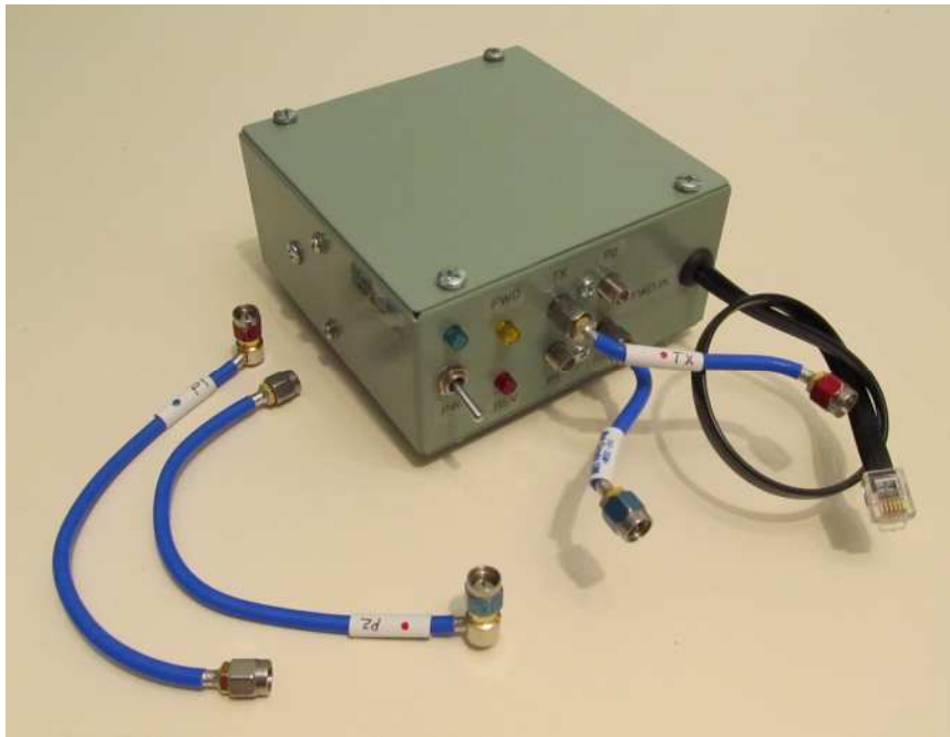
Figure 4 ~ S-Parameter Test Set described in this article. Cost of all parts except coaxial cables was around US$100. Cables cost about US$40. The test set dimensions are 102 mm wide x 50 mm high x 102 mm deep (4 in x 4 in x 2 in). The black cable on the right is the control cable that connects the test set to the VNWA-3E control port. The two blue coaxial cables connected to the transfer switch in the middle-front of the test set connect to the transmit and receive ports of the VNWA-3E. The two loose blue cables on the left are used to connect the test set to the device under test.
