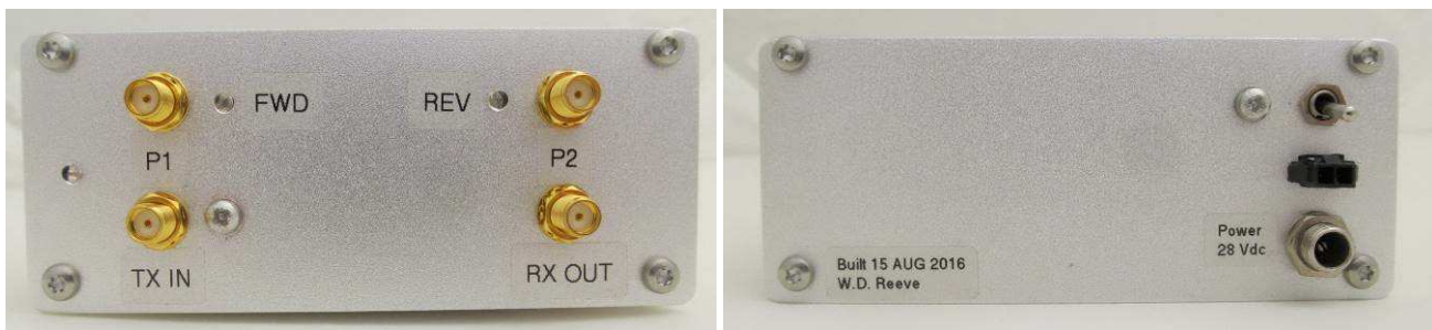
Figure 6 ~ Front (left) and Rear (right) end panels. Labeling is with black on clear labels. What appear to be three empty holes in the front panel are the clear lenses of the power and transfer switch position indicating LEDs. In the right image, the control connector is between the power toggle switch (above) and dc power jack (below), but after cutting the holes I realized the dc power jack should have been placed between the switch and control connector to eliminate minor mechanical interference between the two cables. The Visio layout drawing in the previous figure is correct. Images © 2016 W. Reeve
