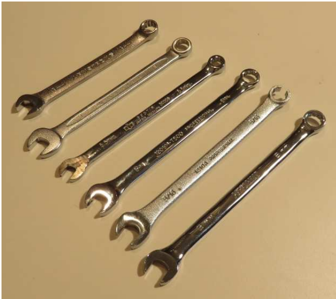
Figure 5 ~ Combination wrenches for the SMA connector. Both 6-point and 12-point box ends are shown. All are 5/16 in or 8 mm except the 3 rd wrench from the top, which is 5.5 mm. I ground down the open end so that it fits the narrow flats on an SMA female-female coupler. Also, I cut the box end of the 2 nd wrench from the bottom to allow it to fit over RG-316/U and RG-174/U coaxial cable pigtailed. These types of wrenches are never used for final tightening of an SMA connector, only to aid in closing the threads before applying a torque wrench. Image © 2015 W. Reeve
