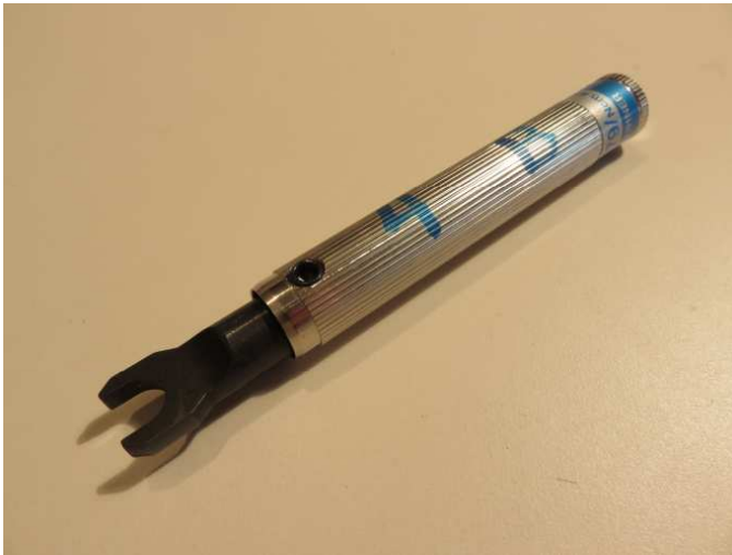
Figure 8 ~ Huber+Suhner 5/16 in click-type torque wrench. When the torque setting is reached, the handle clicks and breaks over a few degrees. This wrench is fixed at 0.45 N-m (4 lb-in) but may be adjusted over a small range with a screw on the handle end. It has been marked with fingernail polish to indicate the torque value (in lb-in) and connector material (B – brass). Image © 2015 W. Reeve
