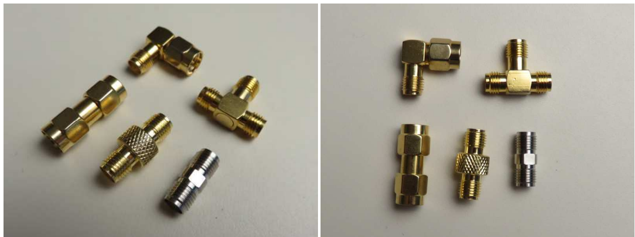
Figure 3 ~ Variety of SMA couplers. The silver female-female coupler at lower-right is nickel plated brass and others are plain brass. The female-female coupler with knurled center grip is used only in quick-test applications where the connectors are not torqued. Images © 2015 W. Reeve
