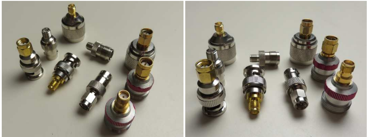
Figure 4 ~ Variety of SMA adapters. Shown here are type N to SMA and BNC to SMA and one TNC to SMA. Images © 2015 W. Reeve
