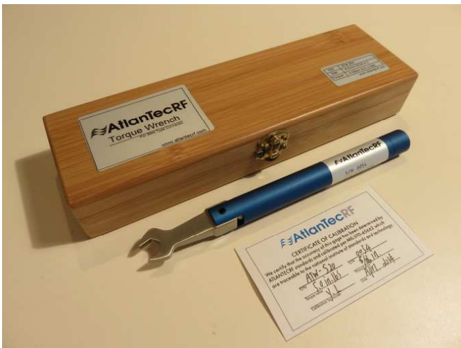
Figure 9 ~ AtlanTech RF 5/16 in break-type torque wrench, which is supplied in a wood case with calibration certificate. Setting is 0.56 N-m (5 lb-in). Image © 2015 W. Reeve
