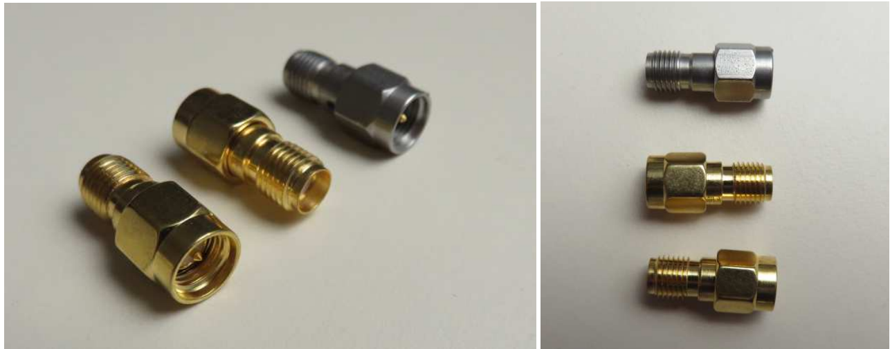
Figure 2 ~ Male-Female SMA adapters commonly used to protect test equipment connectors from wear and damage. When the adapter wears out it is simply replaced at much lower cost than the equipment connector. The upper adapter is stainless steel. Images © 2015 W. Reeve
