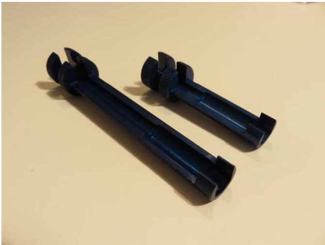
Figure 6 ~ Mini-Circuits HT-series “tight spot” SMA wrenches, one long (102 mm) and one short (63 mm). These finger wrenches are convenient where several SMA connectors are closely spaced. They appear to be made of an aluminum alloy and have been dark blue anodized. Both have an open 5/16 in hex at the lower end for the SMA connector. There is an open slot for the coaxial cable from the lower end to knurled finger grips at the upper end. Between the two finger grips are flats for a 5/16 in or 8 mm open end wrench or torque wrench. Image © 2015 W. Reeve
