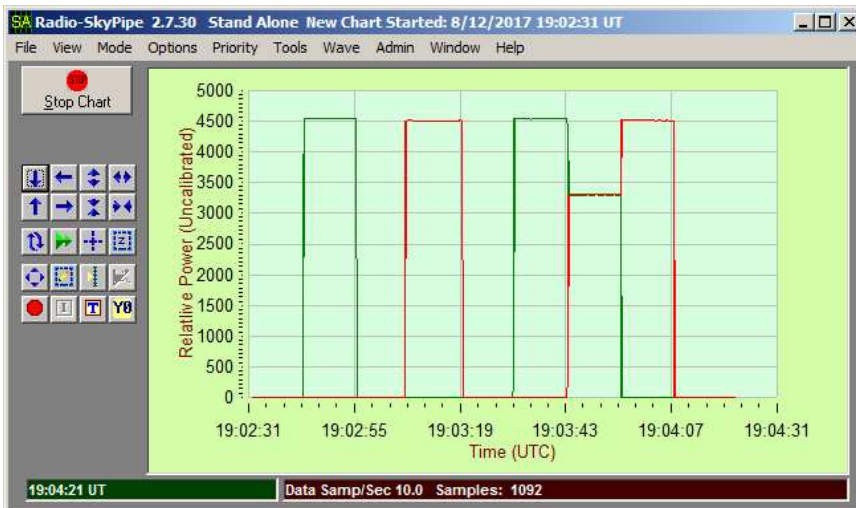
Figure 12 ~ Radio-SkyPipe was setup to use the Left (green trace) and Right (red trace) channels of the PC's internal soundcard. Test sequence: Both Off: ~12 s Left On, Right Off: ~12 s Left Off, Right Off: ~12 s Left Off, Right On: ~12 s Left Off, Right Off: ~12 s Left On, Right Off: ~12 s Left On, Right On: ~12 s Left Off, Right On: ~12 s Left Off, Right Off: ~12 s These measurements were made while running on the internal battery.
