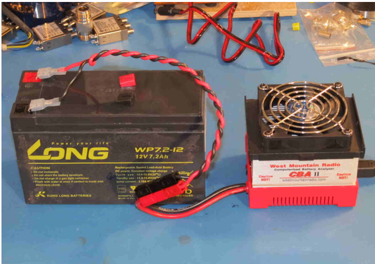
Figure 9 ~ West Mountain Radio CBA-II battery analyzer (right) connected to a 12 V battery for a discharge test. CBA-II dimensions are 90 W x 75 D x 77 H mm. The analyzer and its regularly updated software can be used with numerous battery technologies. The analyzer connects to a PC through a USB 2.0 port (far right in image). The CBA-II is equipped with PowerPole connectors on a short input cable. Any number of adapter cables can be shop-built for various terminations. In this case, a 14 AWG adapter cable was built with push-on connectors matching the F2 battery terminals. The CBA-II is a 2 nd generation analyzer and is rated the higher of 40 A or 150 W at up to 48 V. The latest model is the 4 th generation CBA-IV. Image © 2019 W. Reeve
