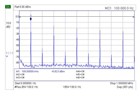
Figure A.4  $^{\sim}$  100 kHz spectra with 20 dB attenuator between the output and spectrum analyzer. Horizontal sweep is from 0 to 1 MHz.
