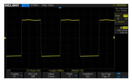
Figure 5 ~ Oscilloscope screenshot of voltage (vertical scale) over time (horizontal scale) showing the measured output waveform at 1 MHz. For this measurement, the scope's vertical channel impedance was set to 50 ohms, and the signal generator output was connected directly to the scope vertical channel. Note the vertical scale is 500 mV/div and the actual peak-peak voltage is 2.40 V (not 3.3 V as specified in the user guide). The horizontal scale is 200 ns/div.
