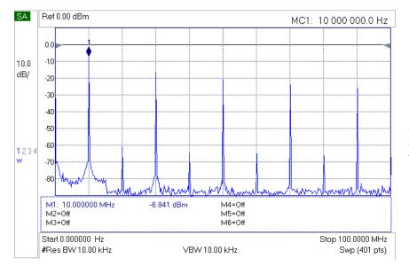
Figure A.8  $^{\sim}$  10 MHz spectra with 20 dB attenuator between the output and spectrum analyzer. Horizontal sweep is from 0 to 100 MHz.
