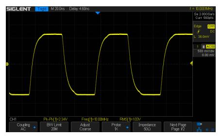
Figure A.7  $^{\sim}$  10 MHz oscilloscope screenshot. Vertical scale 500 mV/div and horizontal scale 20 ns/div.
