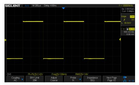
Figure A.1  $^{\sim}$  1 kHz oscilloscope screenshot. Vertical scale 500 mV/div and horizontal scale 200  $\mu$ s/div.
