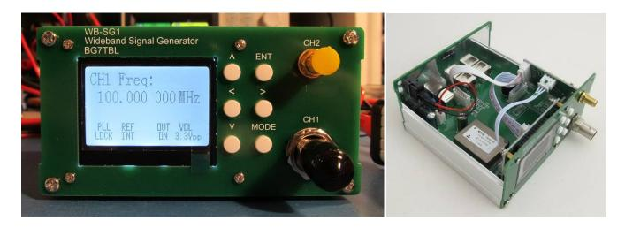
Figure 1  $^{\sim}$  BG7TBL WB-SG1 wideband RF signal generator front view (left) and with top cover removed (right). The dimensions are 106 W x 55 H x 106 L mm (not including connectors) and the weight is 0.35 kg. The connectors for the two output channels, six push-button controls and liquid crystal display are located on the front panel. Images © 2020 W. Reeve
