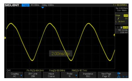
Figure A.9 ~ 100 MHz oscilloscope screenshot. Some, or maybe all, of the harmonics are suppressed by the oscilloscope input circuits. Vertical scale 100 mV/div and horizontal scale 2 ns/div.
