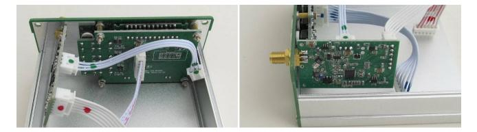
Figure 3 ~ Display PCB (left) and Channel 2 RF PCB (right). Before disassembly, I marked the ribbon cable connectors with a little finger nail polish to ensure I reassembled everything properly; however, the connectors are different sizes so mistakes are improbable. The type SMA-F connector visible in the right image is soldered to the PCB and also mechanically fastens the PCB to the front panel. Images © 2020 W. Reeve
