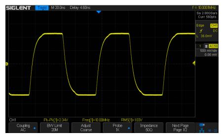
Figure 7 ~ Oscilloscope screenshot showing the measured output waveform at 10 MHz. The measurement conditions are the same as above. The peak-peak voltage has decreased slightly to 2.34 V compared to 2.40 V for 1 MHz. The vertical scale is 500 mV/div and the horizontal scale is 20 ns/div.
