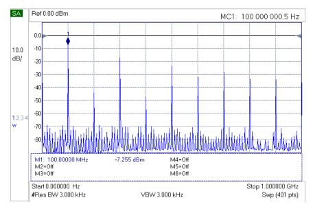
Figure A.10  $^{\sim}$  100 MHz spectra with 20 dB attenuator between the output and spectrum analyzer. Note the many low-level (approximately –60 dBc) spurious signals compared to lower frequencies.
