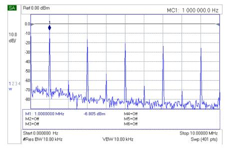
Figure 6 ~ Spectrum analyzer screenshot showing the signal generator channel 1 output when tuned to 1 MHz. The horizontal scale indicates 0 to 10 MHz. Nine harmonics can be seen, primarily odd harmonics indicating a good square wave. The 3<sup>rd</sup> harmonic is about 10 dB down from the fundamental. The spectrum analyzer was connected through a 20 dB attenuator so 20 dB needs to be added to the vertical scale. Horizontal sweep is from 0 to 10 MHz.
