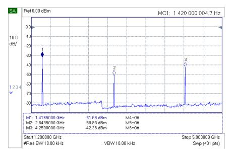
Figure A.11  $\sim$  1420 MHz spectra with 30 dB attenuator between the output and spectrum analyzer. Horizontal sweep is from 1200 to 5000 MHz.
