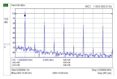
Figure A.6  $^{\sim}$  1 MHz spectra with 20 dB attenuator between the output and spectrum analyzer. Horizontal sweep is from 0 to 10 MHz.
