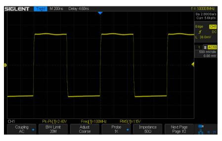
Figure A.5 ~ 1 MHz oscilloscope screenshot. Vertical scale 500 mV/div and horizontal scale 200 ns/div.
