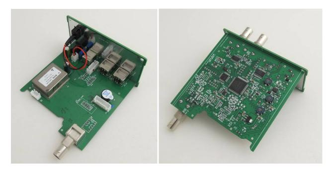
Figure 2 ~ Main printed circuit board top (left) and bottom (right) views, both with the PCB fastened to the rear panel (it is removeable). All components on the main PCB except the oven-controlled crystal oscillator, piezoelectric beeper and ribbon connectors are surface mounted devices on the bottom. The oven-controlled crystal oscillator is the rectangular metal box
