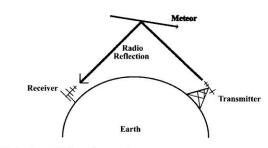
Fig. 3.1. Forward scattering of radio waves from meteor trails.
