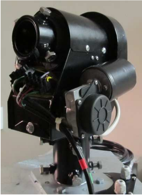
Figure 7 ~ SPID Elektronik model RAS azimuth-elevation rotator. The azimuth motor is visible at middle-right and associated gear and position sensing switch cover is just below it. Except for the vertical main mounting sleeve at the bottom, the entire assembly rotates. The elevation motor is on the opposite side. The elevation gear cover, visible at back-right, encloses one end of the elevation shaft sleeve. The control cable termination compartment is on the front immediately below the elevation sleeve. Eight 10 mm stainless steel bolts clamp the antenna boom (not shown) to the elevation sleeve. The bottom mounting sleeve also has eight 10 mm bolts to secure the vertical pipe mast. The rotator assembly weighs about 31 lb and is approximately 14 in high x 10 in wide x 9 in deep. The manufacturer, SPID Elektronik, is located in Żyrardów, Poland. I purchased the unit from RF HamDesign in The Netherlands. (Image © 2014, W. Reeve)
