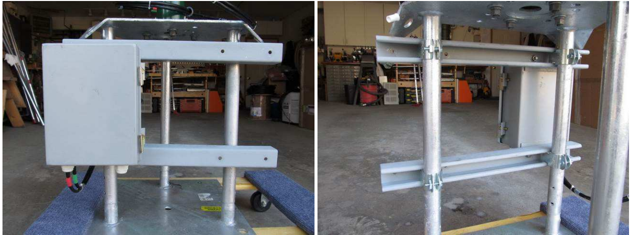
Figure 12 ~ Front (left image) and rear view of channel struts for mounting the tower junction box and tower-mounted amplifier assembly. In the front view, the rotator cable junction box is seen mounted on left side. Holes for the tower-mounted amplifier enclosure are visible on right side. (Image © 2014, W. Reeve)
