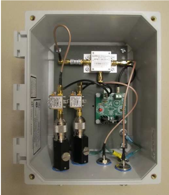
Figure 16 ~ Model TMA-2 tower-mounted amplifier shown without weatherproof cover. The polyester enclosure is 8 in high x 6 in wide x 4 in deep and has a rubber gasket on the removable cover. This unit is equipped with two low noise amplifiers (middle-left), lightning arrestors (bottom-left), bias-tee (top) with voltage limiter (top-left), step-down linear power supply and a bonding/grounding stud for the conductive components and lightning arrestors. (Image © 2014, W. Reeve)
