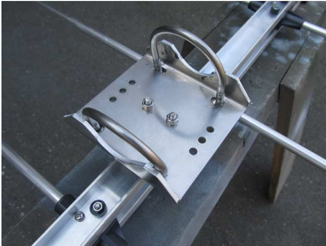
Figure 6 ~ One of two aluminum saddle clamps and stainless steel U-bolts supplied with each antenna for mounting on the antenna boom structure. The clamps are fastened to the bottom of the antenna's transmission line boom structure seen crossing the image diagonally bottom-left to top-right. (Image © 2014, W. Reeve)
