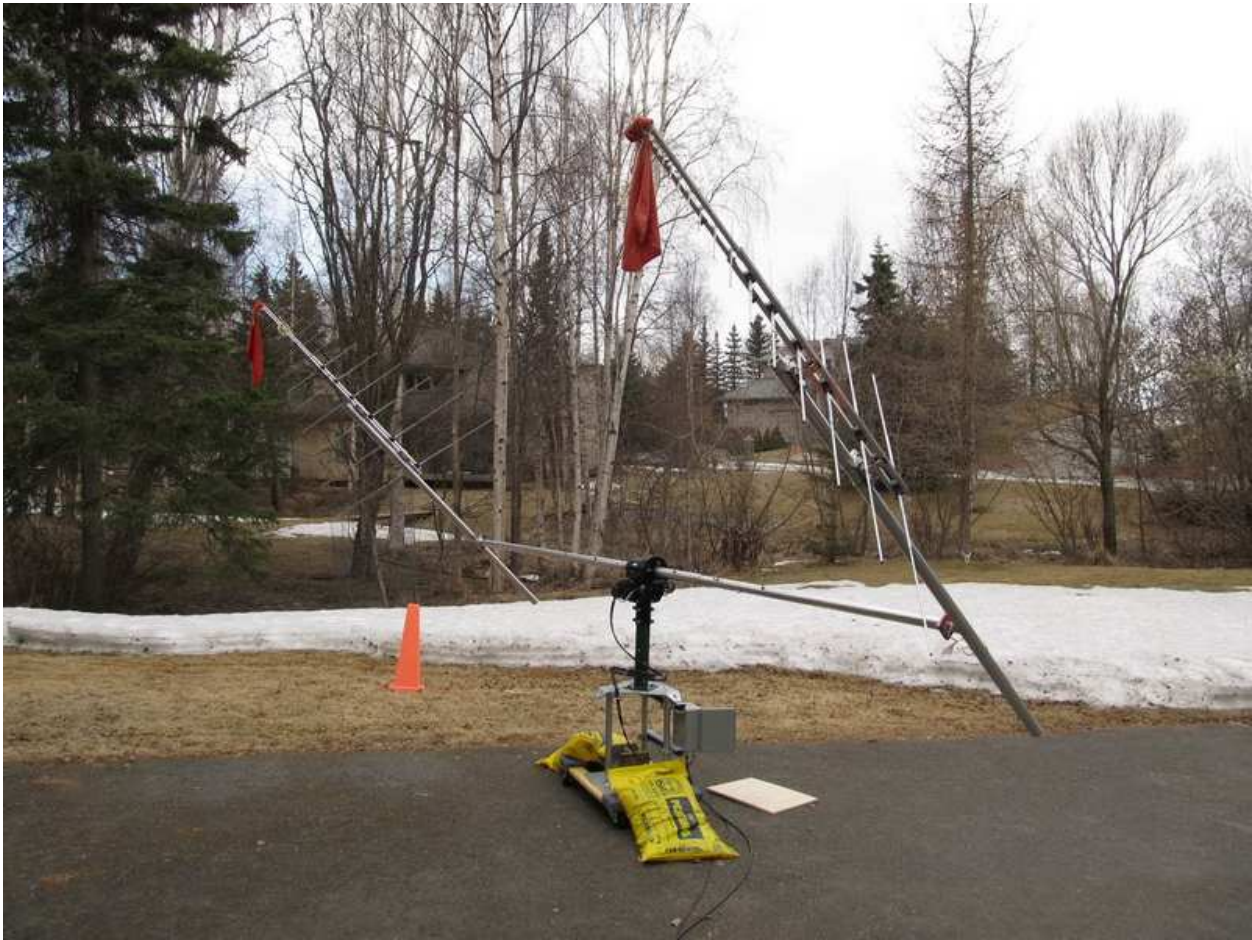
Figure 15 ~ Rotator test setup. The tower top plate is on a spare tower base plate held down with 50 lb lead weight on a furniture dolly (the two 60 lb bags of pea gravel prevent movement). The rotator mast adapter, rotator mast, rotator, junction box and rotator cables have been permanently installed, and the support booms and antennas are temporarily installed for testing. Red flags warn passerby's of the low visibility antennas. When this image was taken on 23 April 2014, the system was tracking the Sun, which was near transit (transit is when a celestial body crosses a north-south line about halfway between rising and setting). (Image © 2014, W. Reeve)
