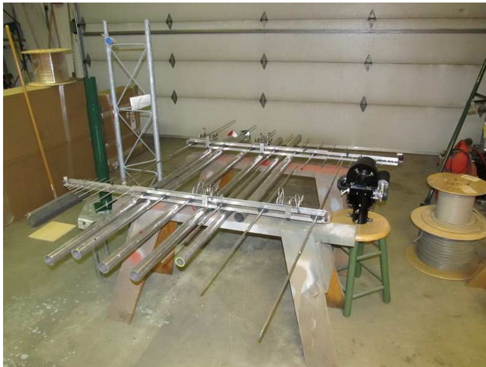
Figure 1 ~ Pile of parts: Callisto-High antenna system components fabricated and ready for assembly and testing. Components include dual horizontal support booms (on saw horses), two log periodic antennas (pointed left and right on top of support booms), rotator (black object at right) and tower extensions and top plate (on left) that raise the tower height about 6 ft above the 60 ft height described in Part 3 [Reeve3]. The transmission lines, control cables, tower-mounted amplifier and junction box enclosures are not shown. (Image © 2014, W. Reeve)
