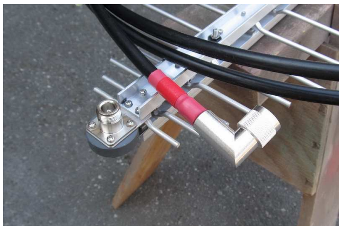
Figure 18 ~ Antenna RF connector (left) and associated right-angle type N cable connector. LMR-400 coaxial cable is shown adjacent to the antenna RF connector prior to connection and routing (the antenna is shown upside down; the connector is pointed downward in actual installation). The antennas will be mounted on their respective booms and RF connections made and sealed prior to raising the boom structure to the tower top. (Image © 2014, W. Reeve)
