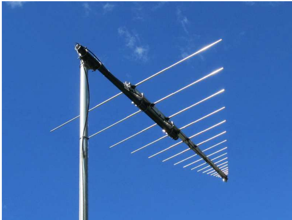
Figure 2 ~ The Creative Design CLP5130-2N log periodic antenna setup for horizontal polarization on a test mast. The antenna is 1.4 m long and the longest element is 1.45 m. The rear boom mount is called a “dragon-fly” mount and adds 0.5 m to the antenna length. The type N RF connector is at the front of the antenna and points down. (Image © 2014, W. Reeve)
