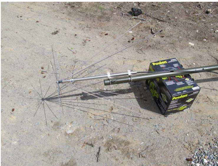
Figure 7 ~ Discone antenna fastened to mast top section with clamps. A discone antenna is broadband, omnidirectional and has zero gain. The mast rests on a cardboard box before being raised.
