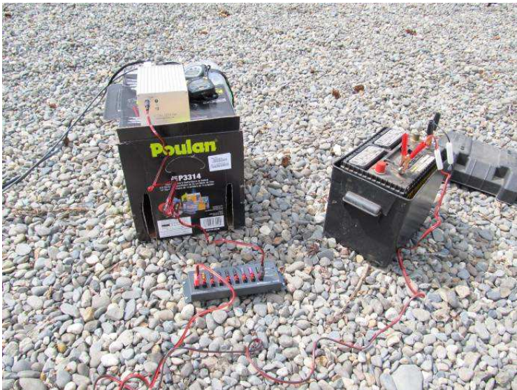
Figure 5 ~ Outdoor equipment setup on gravel pad at site. Power was supplied by battery (right) through a PowerPole distribution panel (foreground) to the receiver (silver object on box, upper-left).
