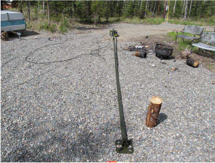
Figure 8 ~ Mast and antenna were completely assembled on the ground with guy ropes attached to a guy ring located about 2 m below the top (guy ropes are on the ground and angled away from mast). The mast base (middle-bottom) is secured by two pegs driven into the ground. The mast itself is hinged at the base and it is a simple matter to raise the assembly and secure the guy ropes. The tree log to the right and above the mast base was used as a chair.
