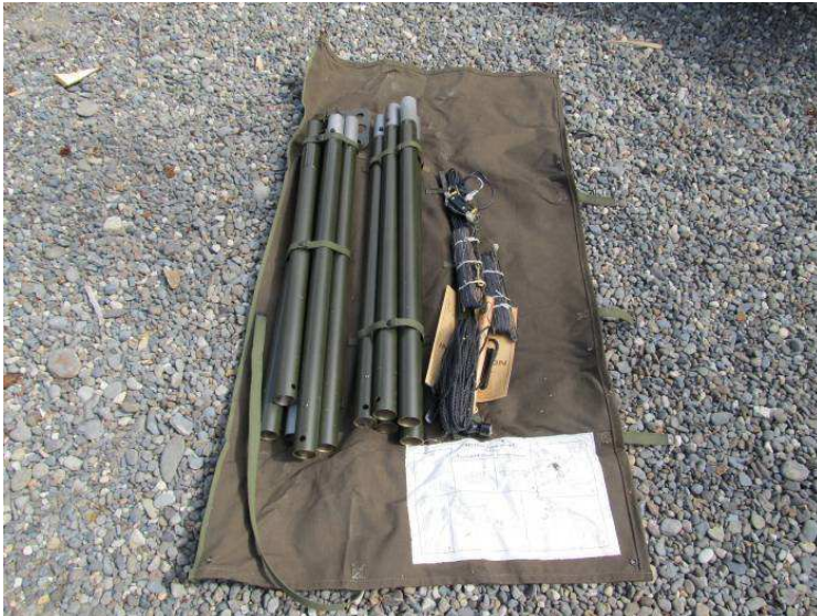
Figure 6 ~ Portable aluminum mast sections in canvas pouch ready for assembly. Each section is about 48 in long x 2-1/8 in diameter (1220 x 54 mm); one end is necked down (swaged) to fit inside the section above it. Three Dacron guy ropes and associated anchor pegs are packed to the right of the mast sections. The mast originally was designed to support an adjustable-length HF dipole antenna and associated coaxial feedline included with it (seen bundled above the guy ropes).
