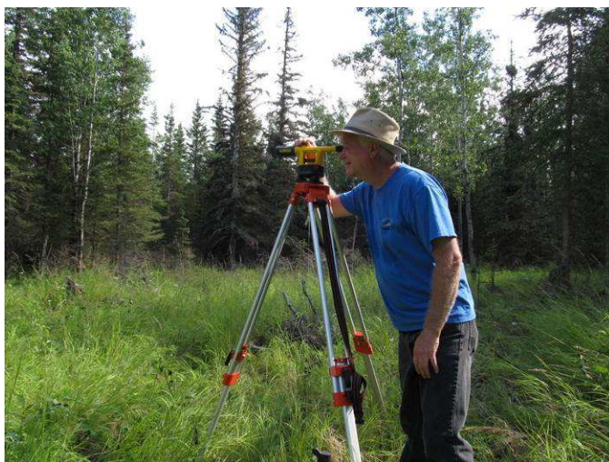
Figure 2 ~ Tower layout was done with a builder's level and surveyor's tape while working alone on a nice summer day.
