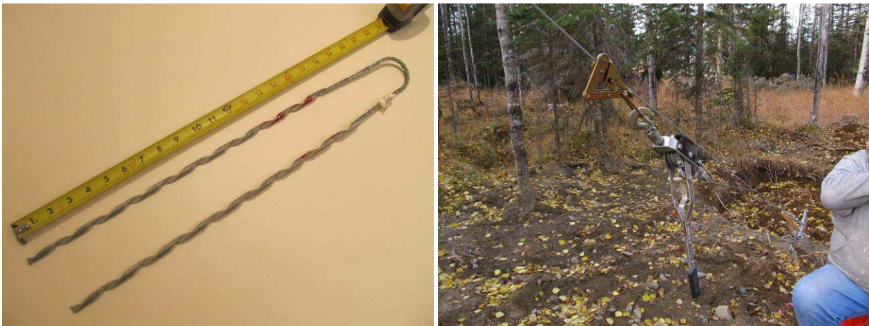
Figure 6 ~ Left : Preformed Line Products “Big Grip” deadend. The grip is wrapped around the guy strand and, after installation, has a breaking strength that exceeds the strand. The holding force is the rough galvanizing on the two surfaces. The grips can be removed and reapplied twice for guy adjustment and re-tensioning but must be discarded if removed a third time. The grip uses a thimble (not shown) to prevent damage from chafing where it is looped around the guy bracket or turnbuckle pin. Right : A cable hoist and Klein “Chicago”-style wire pulling grip were used to tension the guy strand while the deadend was installed. (Images © 2014, W. Reeve)
