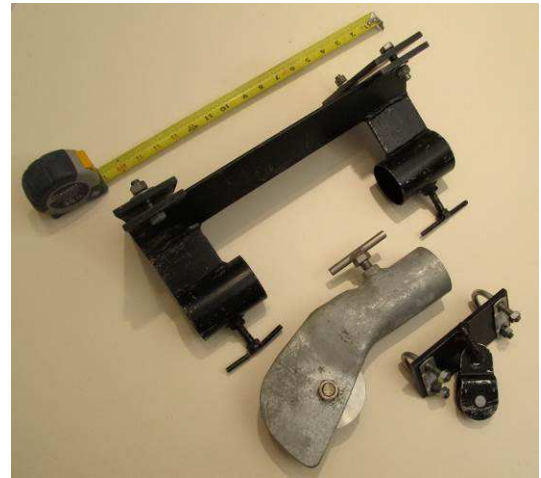
Figure 8 ~ Gin pole setup (left). The gin pole is schedule 15, hot-dipped galvanized pipe purchased at a fence company in Anchorage, which cut it to length for me. The sheave at the top of the gin pole is part of my gin pole kit that includes the pipe, clamp and upper and lower pulleys (above right). (Images © 2014, W. Reeve)
