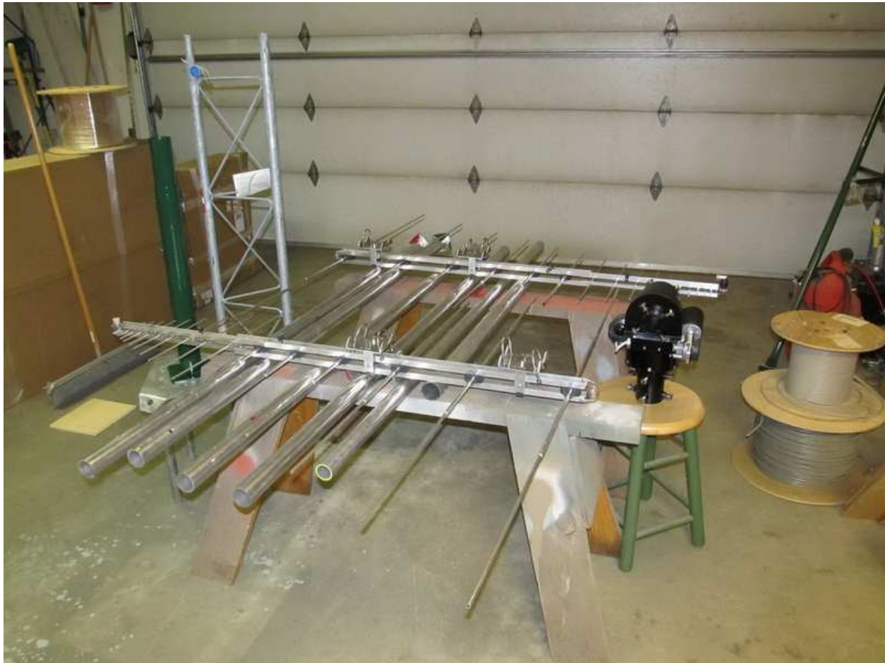
Figure 15 ~ Pile of parts – Callisto antenna system components to be described in Part 4. Components include dual horizontal support booms (on saw horses), two log periodic antennas (pointed left and right on top of support booms), rotator (black object at right) and tower extensions (on left) that will raise the tower height about 7 ft above the 60 ft height described in Part 3. (Image © 2014, W. Reeve)
