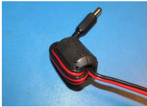
Figure 8 ~ Bifilar winding on clamshell noise suppression ferrite bead. Both positive and negative leads are wound side-by-side on the bead. (Image © 2014 W. Reeve)
