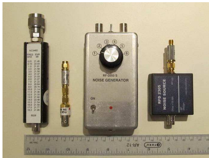
Fig. 1-3 ~ Calibrated noise sources. Left-to-right: Hewlett-Packard 346D (ENR 21 dB), Renz RQ6 with 20 dB attenuator (ENR 55 dB without attenuator), RF Associates RF-2050S (Noise temperature switchable 43 thousand to 1.4 million kelvin), RF Design RFD2305 with 10 dB attenuator (ENR 5 dB with 10 dB attenuator). ENR (excess noise ratio) is discussed in Part V.
