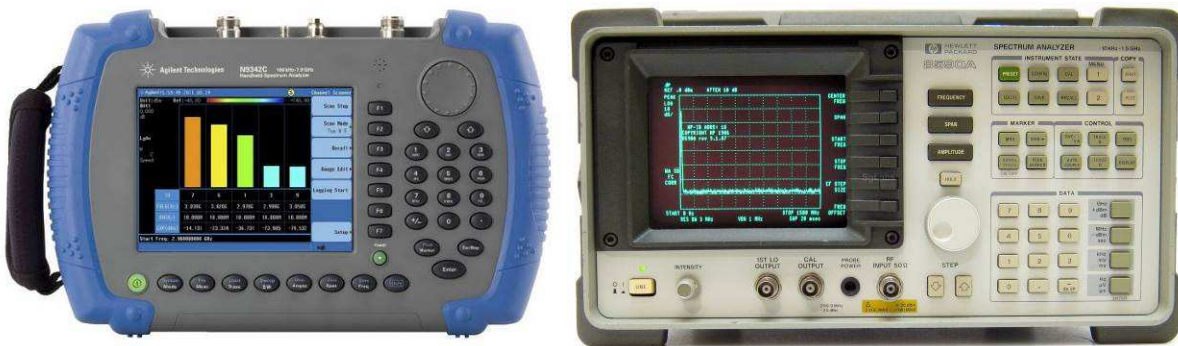
Fig. 6-1 ~ Spectrum analyzers. Left: Agilent N9342C Handheld Spectrum Analyzer (HSA) weighs 3.2 kg. This high-performance instrument has many built-in features that simplify noise measurements including a power spectral density function, noise markers and a built-in low noise preamplifier. However, even with these features, additional gain from an external low noise amplifier still is needed to boost the HSA's sensitivity for noise factor measurements of external devices. Right: Hewlett-Packard 8590A is a high-performance instrument marketed in the mid-1980s as "Portable". It weighs 13.5 kg, and compared to the previous generation of spectrum analyzers it was very portable.
