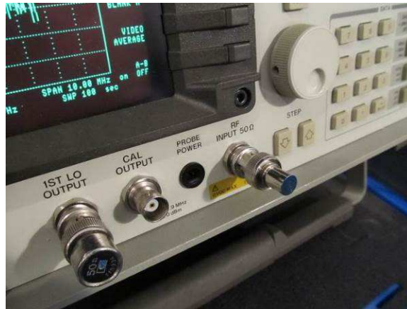
Fig. 6-2 ~ Hewlett-Packard 8590A spectrum analyzer terminated in 50 ohms (just right of center) to measure the spectrum analyzer's noise floor and noise factor.
