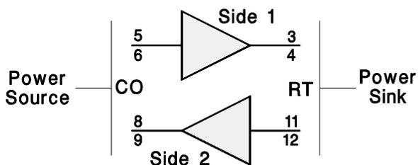
Fig. 6(a) shows the simplified schematic of a repeatered T1-carrier line repeater with the connections necessary on the upstream side of the line repeater to loopback the upstream signal. This configuration is used to check the signal up to the line repeater but does not check the repeater itself. Unplug the repeater and connect the test set as shown. The test set receiver should be set for “Auto” framing, the transmitter framing and payload set for “As Input” and transmitter timing
