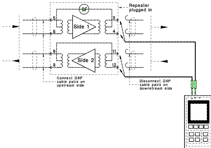
The output signal level on either side 1 or side 2 will be close to 0.0 dBdsx. Be sure to observe the test set termination rule: If the line being tested terminates in an active device, the “Bridging” mode should be used. If the test set is to terminate the line (as in the case with the outside plant cables disconnected from the repeater), the “Terminate” mode should be used.
