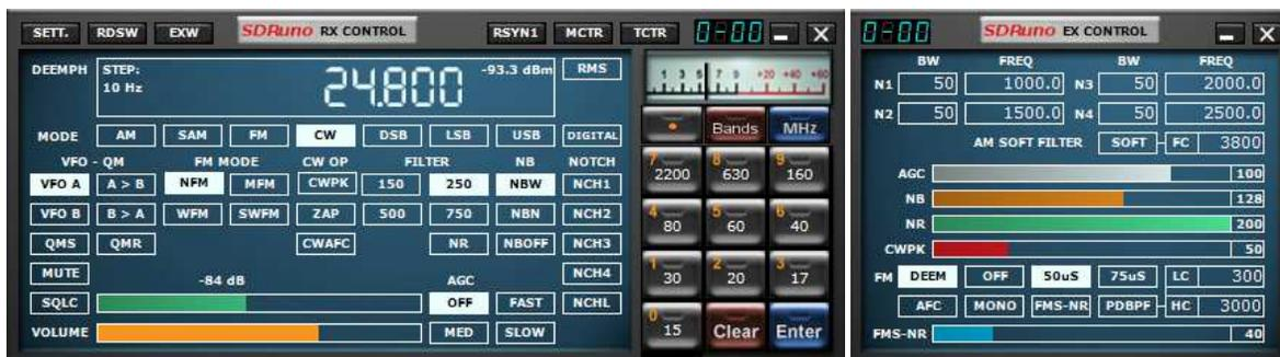
Figure II.8 ~ RX Control (left) and EX Control (right) windows for station NLK (24.8 kHz). These windows are used to control the settings for individual virtual receivers. Except for receiver frequency the same settings were used for all data recordings. The noise blanker (NB) threshold setting of 128 in the EX Control was determined experimentally as a compromise between loss of sensitivity and noise spike reduction.
