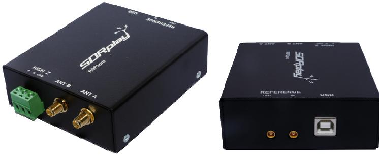
Figure II.4 ~ SDRPlay RSP2Pro software defined radio receiver. Dimensions are 99 x 87 x 33 mm, 0.3 kg. The balanced high-impedance antenna interface is the green pluggable connector on far-left. The receiver is powered through its USB connection and draws about 170 mA at 5 Vdc. Images source: SDRPlay, used with permission.
