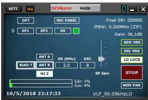
Figure II.7 ~ SDRuno Main window shows general and common receiver settings including antenna port, RF gain, sampling rate and decimation. Also, the receiver is started and stopped and virtual receivers are assigned from this window. Only one virtual receiver was used during this propagation study. The two horizontal meters at bottom-left indicate the PC system and software loads. In this case, the SDRuno software added 1% to the overall system load of 4%.
