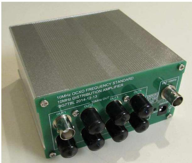
Figure 10 ~ Two views of the BG7TBL distribution amplifier. Seven of the eight output connectors are covered with rubber protective caps. The input from the reference source is on the upper-right of the front panel. Enclosure dimensions are 100 W x 103 L x 55 H mm not including connectors
