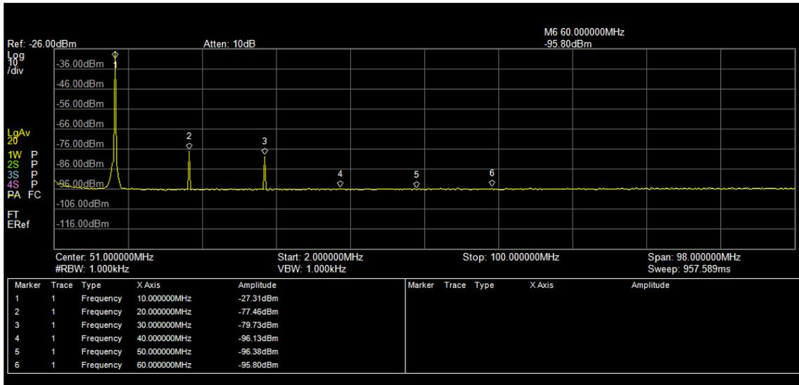
Figure 13 ~ Wider spectrum view of the same output as in the previous figure. At least six harmonics are visible. The 2<sup>nd</sup> harmonic is about 50 dB below the fundamental.
