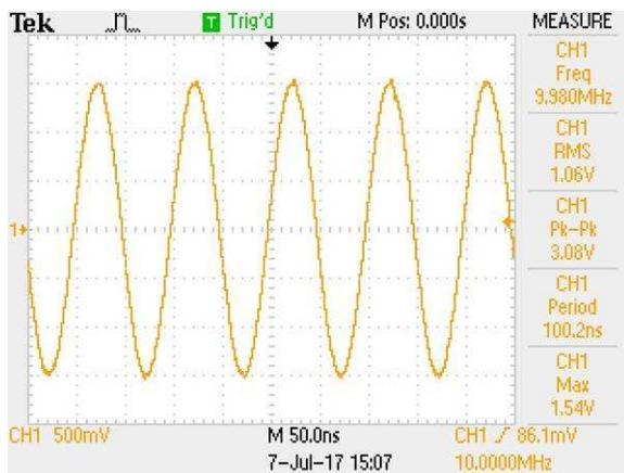
Figure 11 ~ Oscilloscope screenshot of the waveform for one output channel on the BG7TBL distribution amplifier. Note that the output is very close to the desired 1.0 Vrms nominal value. The output was terminated with 50 ohms for this measurement.
