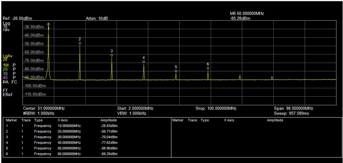
Figure 9 ~ Wider spectrum view of the same output as in the previous figure. At least eight harmonics are visible. The 2<sup>nd</sup> harmonic is about 27 dB below the fundamental.
