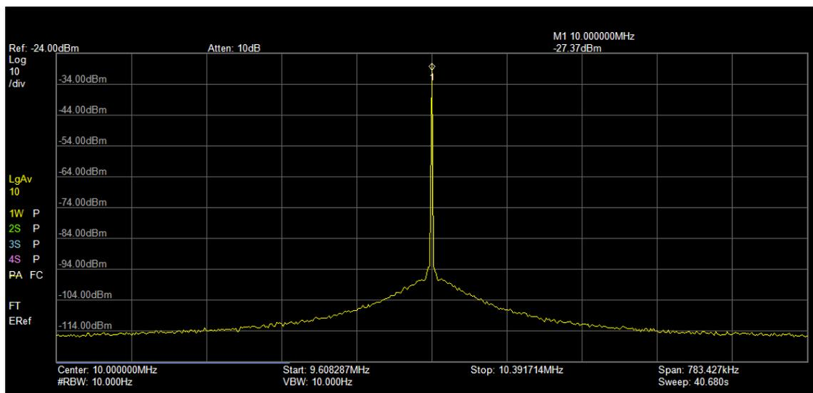
Figure 12 ~ Narrow spectrum view of the 10 MHz reference output from one of the channels of the BG7TBL amplifier. The span shown here is about 783 kHz.
