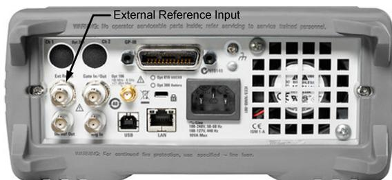
Figure 2 ~ Test equipment usually have a BNC-F connector on the rear panel for connection to an external reference source. The 10 MHz reference input on this Keysight 53220A frequency counter is labeled *Ext Ref* and is the upper connector on the far left. This frequency counter was used for the phase measurements described later.
