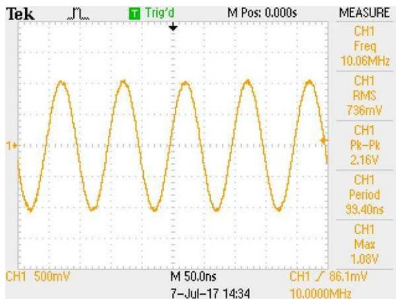
Figure 7 ~ Oscilloscope screenshot of the waveform from the G4HUPRF distribution amplifier. Note that the output is about 0.74 Vrms, slightly below what is usually considered the acceptable range at the output of a 10 MHz reference. The output was terminated with 50 ohms for this measurement.
