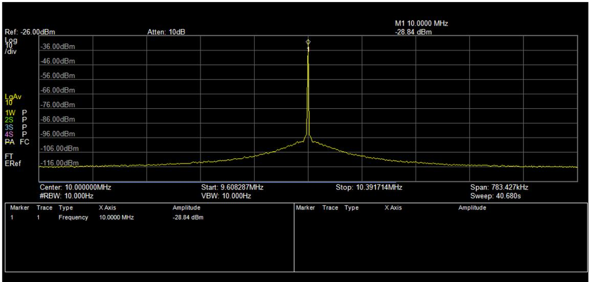
Figure 8 ~ Narrow spectrum view of the 10 MHz reference output from one of the channels of the G4HUPRF amplifier. The span shown here is about 783 kHz, which resulted from using the analyzer *Autotune* function.
