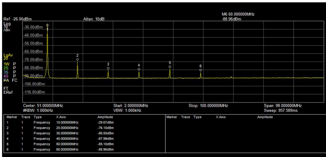
Figure 4 ~ Spectrum of the TS-2700 reference source. The first seven harmonics are visible. The 2<sup>nd</sup> harmonic at 20 MHz is about 46 dB below the 10 MHz fundamental.
