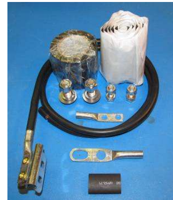
Fig. 7 – Coaxial cable bonding clamp (right). Bonding clamps usually cover a range of coaxial cable diameters. The cable jacket is carefully cut away to expose the shield. The preformed copper strap (lower-left corner of photo) is installed over the shield, sealed with the included mastic tape (upper) and then bonded to the earth electrode system using the wire provided. This particular kit costs about US$35 and is used with LMR400 coaxial cable. Less expensive kits are available for about US$10 that loop around and then clamp the exposed cable shield
