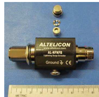
Fig. 5 – Antenna discharge unit for coaxial cable with type N connectors and a replaceable gas-tube element. The gas-tube element has been removed and is the small cylinder just above the main body and below the spring and cap. When the voltage across the gas-tube reaches its threshold value, the gas inside the element conducts. The resulting current is diverted to earth ground where it is safely dissipated. The screw for connection of the bonding conductor is on the bottom of the body. This type of arrestor device has redundant features with respect to the NEC – voltage limitation of the antenna discharge unit and shield grounding. This device is shown for illustration of concepts and is not listed in UL 452
