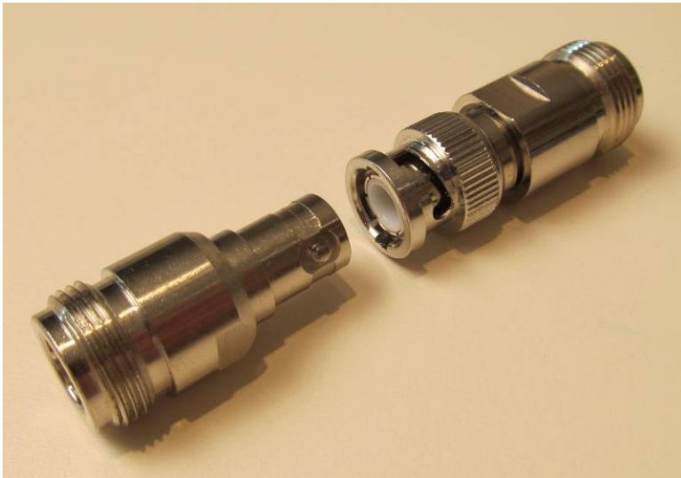
Figure 6 ~ Type BNC-female to N-female (left) and BNC-male to N-female (right) adapters used during the measurements but not during calibration. These adapters introduced a 10 dB reduction in return loss when they were attached to the VNA test cables. The manufacturer and model is unknown. Note the flats for a wrench. A wrench normally is not used to tighten type N connectors; however, a wrench may be used to hold the adapter and prevent it from turning while the mating connector is tightened by hand. Image © 2019 W. Reeve
