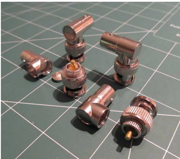
Figure 1 ~ Poor quality right-angle BNC adapters. The two pieces at lower-right are the male and female parts of the adapter that fell apart in my hand. The knurled press-fit barrel is visible in the lower-right foreground. More detailed images are shown later. The three pieces to the left are from another identical adapter that I easily pulled apart with pliers. The end-cap for the female barrel part was removed and is partially hidden behind the male body part. The two adapters in the back are intact but went to the garbage can. Image © 2019 W. Reeve
