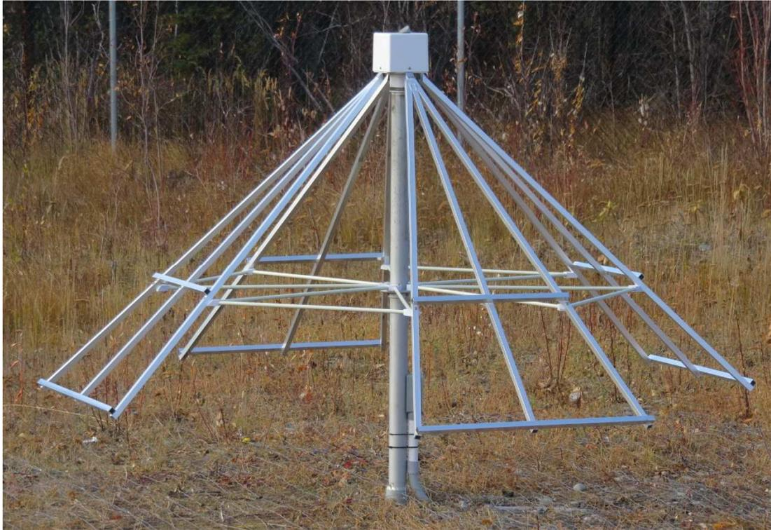
Figure 2 ~ LWA Antenna installed at the Modular UHF Incoherent Scatter Radar (MUIR) site on the HAARP facility. The antenna consists of aluminum, tied-fork, crossed-dipoles supported on a 1.5 m steel mast. Frequency range is approximately 10 to 100 MHz but is usable only to about 85 MHz because of FM broadcast station interference. Image © 2021 W. Reeve
