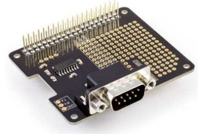
Figure 2 ~ *Serial Pi Plus* Hat used in Callisto-Lx includes a MAX3232 transceiver, a few charge pump and decoupling capacitors, a DB-9M connector and a 40-pin GPIO connector. The DB-9M connector is shown soldered to the PCB in this image but is removed to reduce space requirements when the RPi assembly is installed in an enclosure. Image source: AB Electronics.
