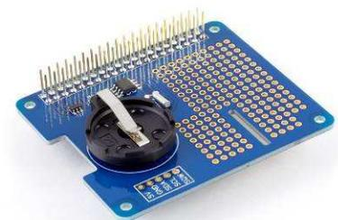
Figure 3 ~ *RTC Pi Plus* Hat used in Callisto-Lx includes a DS1307 integrated circuit, an I<sup>2</sup>C bus interface IC, a few passive components, battery holder and a 40-pin GPIO connector. The battery is supplied by the user. Image source: AB Electronics.
