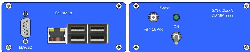
Figure 6 ~ Callisto-Lx front and back panels. Left: The front panel is cutout for flush-mounting the RPi USB and Ethernet interfaces and also includes a DB-9M connector for the serial interface, which is wired to the RPi through a wire-mount socket housing. Right: The power input jack, on-off switch and power indicating LED are on the back panel. The rear panel also is wired to the RPi through a wire-mount socket housing.
