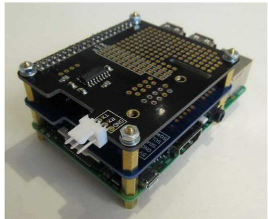
Serial interface: The Callisto-Lx serial interface uses signals available on the RPi general-purpose input/output (GPIO) connector. The GPIO is based on 3.3 V CMOS logic and is not directly compatible with the EIA-232 interface required by the Callisto instrument. Therefore, it is necessary to use a voltage level converter transceiver. The
