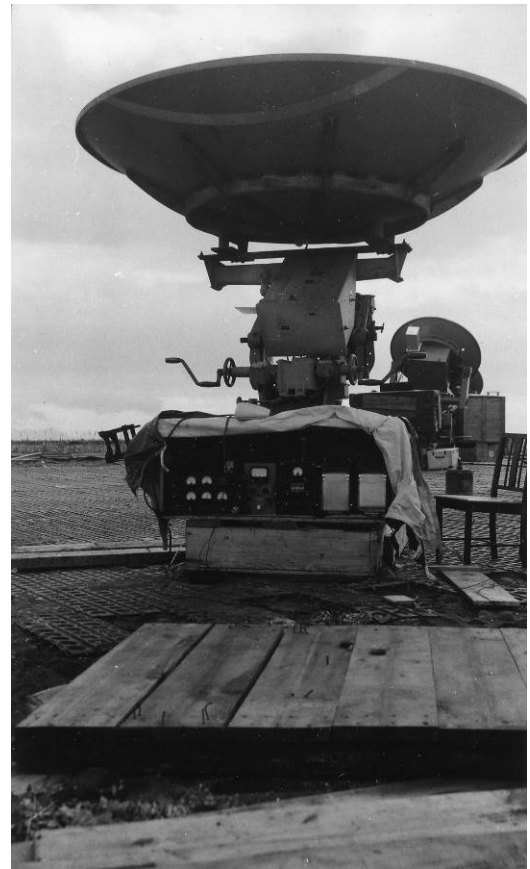
465 mc apparatus (10 foot radar mirror) from north, close view, Attu, Alaska, eclipse expedition site
