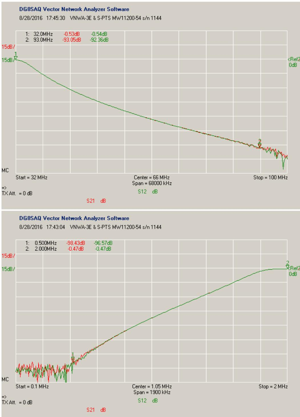
Figure 13 ~ Stopband measurements setup for 15 dB/division with 0 dB reference on the 8<sup>th</sup> grid line. Upper: Linear frequency sweep from 32 to 100 MHz shows the loss approaches 100 dB but measurements are limited by the VNWA-3E noise floor. Lower: Linear frequency sweep from 0.1 to 2 MHz indicates the stopband loss exceeds 100 dB but, as above, the measurements are limited by the instrument's noise floor.
