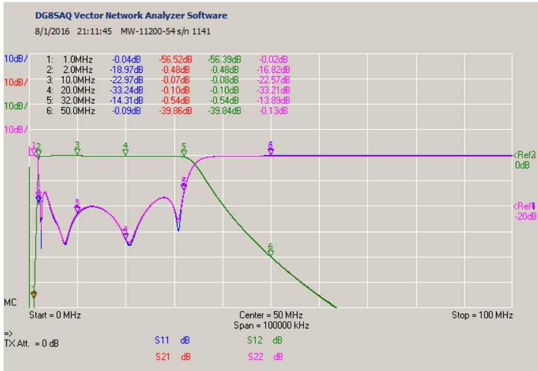
Figure 4 ~ Typical s-parameter plots from the VNWA-3E analyzer. The vertical scale shows dB. The 6<sup>th</sup> division is the 0 dB reference. The horizontal scale is frequency from 0 to 100 MHz. The s-parameters and their corresponding trace colors are indicated at the bottom. The marker table at the upper-left shows the marker frequency and corresponding values for each trace. This plot has four traces but two are hidden underneath another trace.
