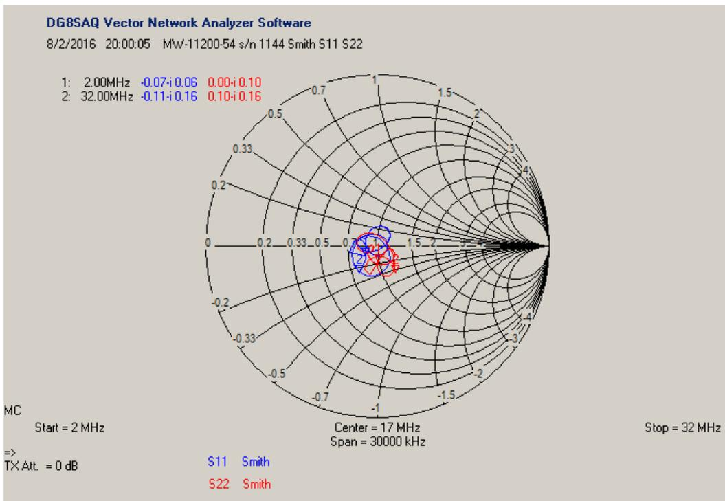
Although the Smith Chart grid is setup to show normalized impedance, the marker tables shows the corresponding reflection loss. Because the traces are near the center of the chart, the filter is very well matched to 50 ohms over the frequency range indicated.
