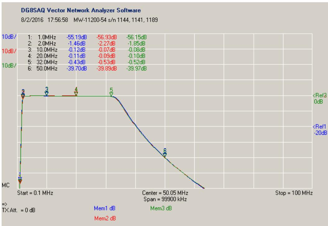
Figure 10 ~ Passband loss (S21) for the three filters overlaid on each other for comparison. This plot shows that for practical purposes the three filters have identical loss with frequency.
