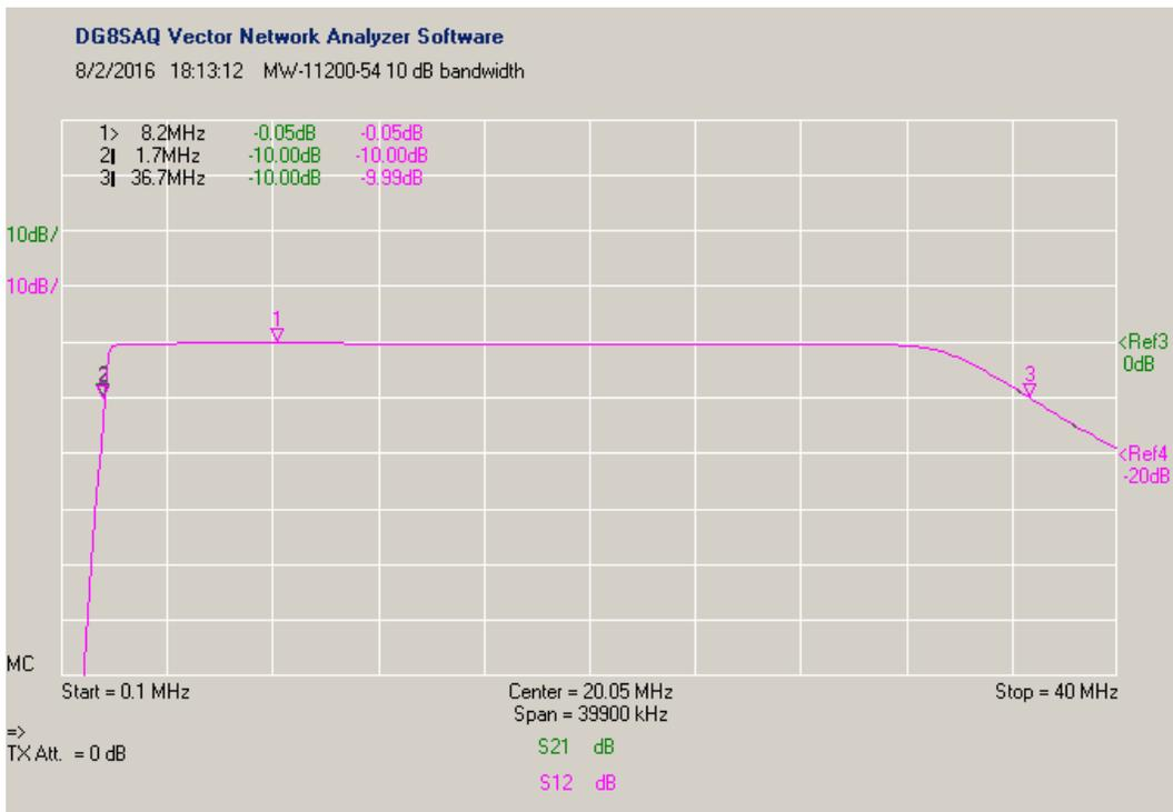
Figure 11 ~ The 10 dB bandwidth is determined by adjusting the vertical scale and then placing left and right markers (markers 2 and 3) one division below the reference (marker 1). In this case, the bandwidth is 36.7 – 1.7 MHz = 35 MHz.
