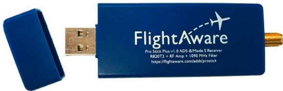
Figure 6 ~ FlightAware USB Pro Stick Plus receiver. The receiver is powered by 5 Vdc through the USB connection on the left. The SMA antenna connector is on the right. This version of the receiver has a built-in bandpass filter to reduce interference. Principle dimensions are 70 L x 30 W x 13 D mm. Image source: FlightAware
