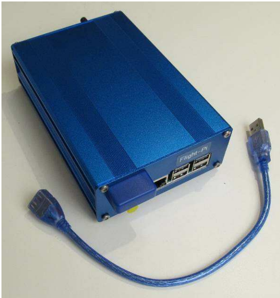
Figure 1 ~ Flight-Pi eliminates flying leads and exposed electronics by packaging the receiver, Raspberry Pi computer and a converter power supply in an extruded aluminum enclosure. The USB-A extension cable in the foreground is used to connect the receiver USB port on the upper-left of the front panel to one of the Raspberry Pi USB ports on the lower-right. The receiver USB port is shown here with the protective cover. The power jack, power indicating LED and power switch are located on the rear panel. The Flight-Pi principle dimensions are 160 D x 109 W x 45 H mm. Image © 2018 W. Reeve
