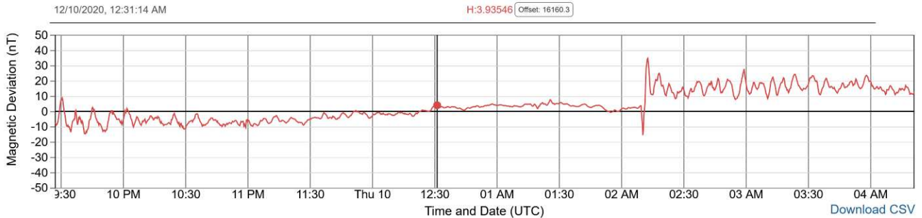
Figure 3 ~ Plot of the H-component of the magnetic field measured by magnetometers at Gakona and Kenai Peninsula College. These magnetometers are operated by University of Alaska Fairbanks – Geophysical Institute. Note the similar signature of the sudden impulse compared to the SAM-III at Anchorage. However, the UAF-GI magnetometers have lower time resolution. Image source: {UAF-GI}. Magnetometer data, Geophysical Institute, UAF 2020. Retrieved from Research Computing Systems 10 December 2020.
