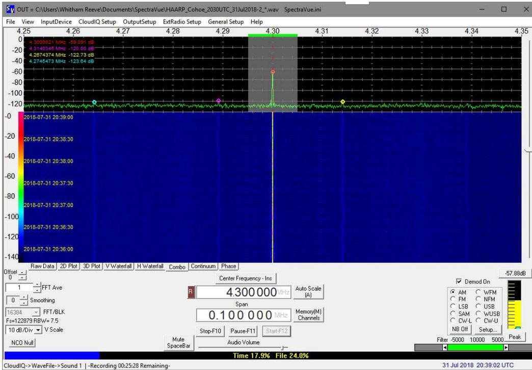
Figure 12.a ~ SpectraVue: 2039 UTC, 31 July, Live: 4.300 MHz. Displayed frequency span is 100 kHz and demodulation is set to AM.
