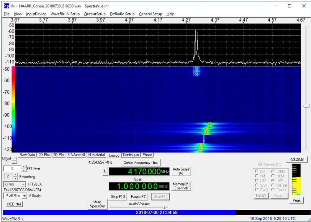
Figure 10.c ~ 30 July 2018, 2105 UTC. Playback: Stepped followed by multi-carrier, 4.17 MHz. There are a few minutes dead-time between the end of the stepped and multi-carrier transmissions.
