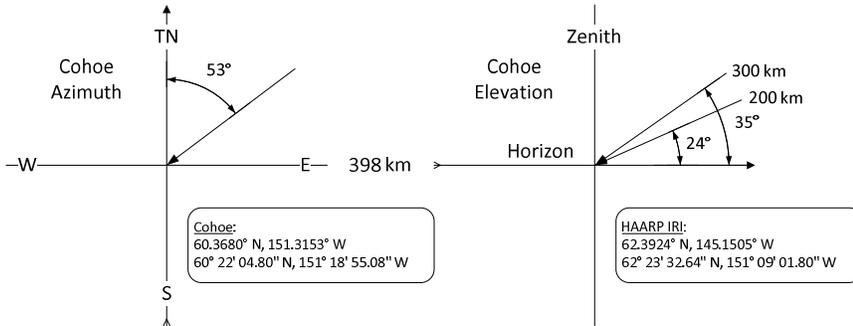
Figure 5 ~ Azimuth (left) and elevation (right) for propagation path to the F-region ionosphere directly above the HAARP site; these assume a vertical beam at HAARP. Different beam angles will change the values slightly. Two ionosphere heights are shown because it can vary. Azimuth is with respect to True North (TN). Image © 2018 W. Reeve
