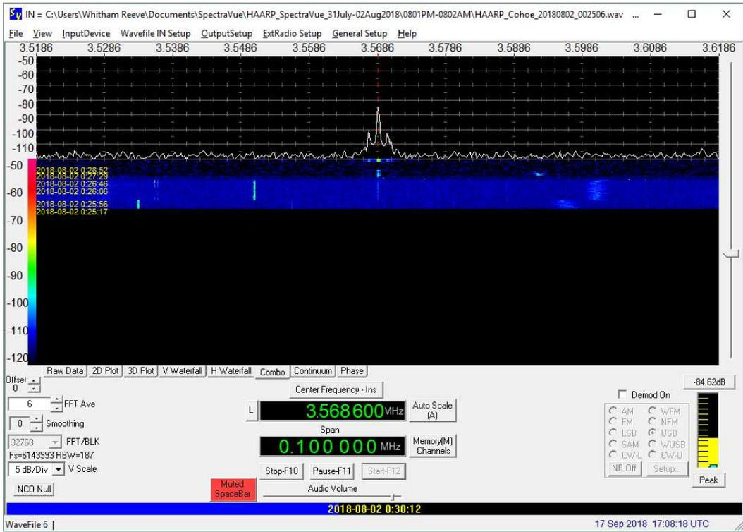
Figure 10.g ~ 02 August 2018, 0030 UTC. Playback: 3.5686 MHz (WSPR), 100 kHz span showing sidebands at approximately  $\pm 1500$  Hz.
