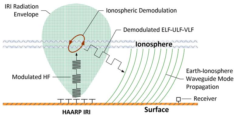
Figure 3 ~ Low frequency radio waves may be produced by ionospheric demodulation of the modulated signals from the HAARP IRI. These emissions then propagate over great distances in the Earth-ionosphere waveguide. Image adapted from {DTIC}
