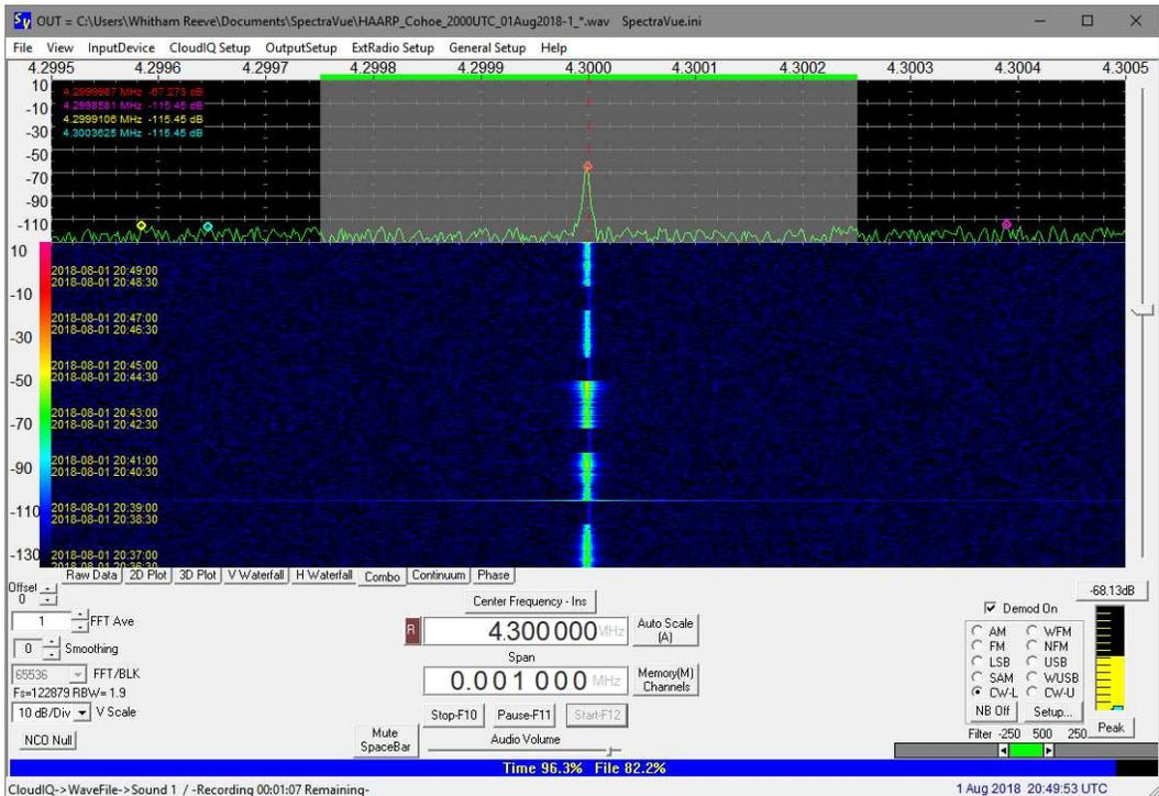
Figure 13.b ~ SpectraVue: 2049 UTC, 01 August, Live: 4.300 MHz. The shaded area in the spectrum indicates the limits of the filter used during demodulation, in this case CW-Low (sideband). The displayed frequency span is 1000 Hz and demodulation is set to CW-low.
