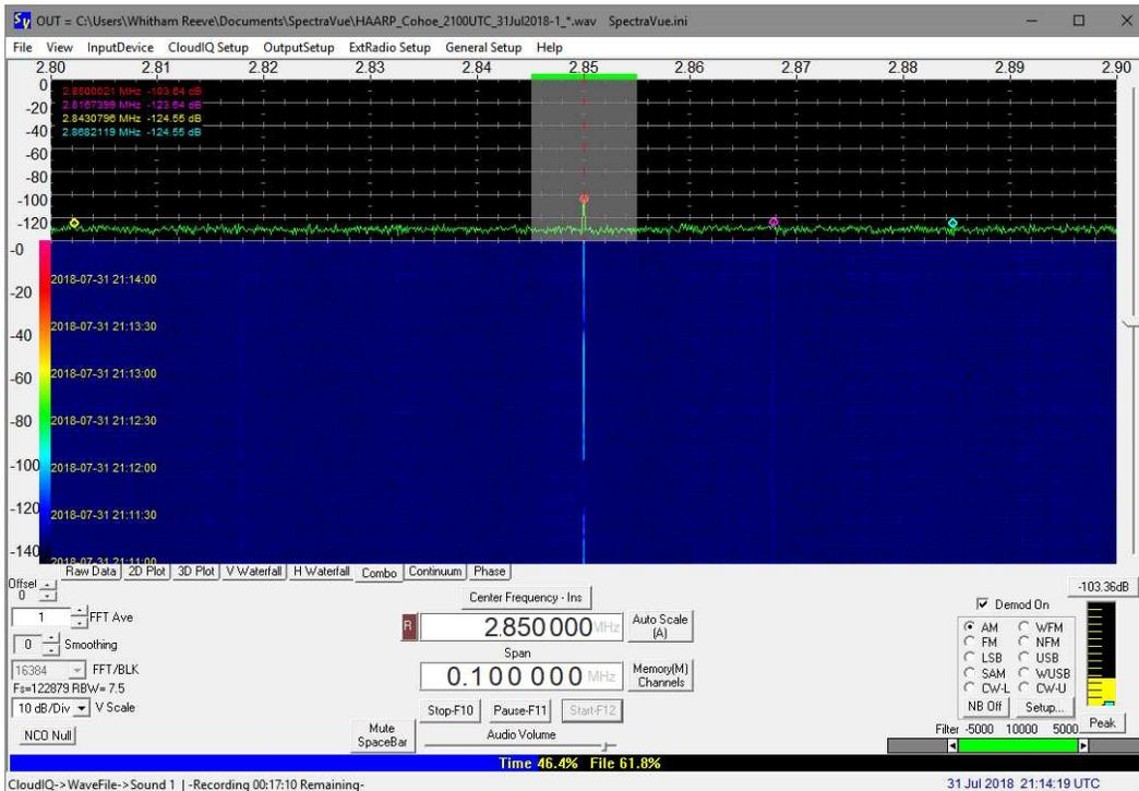
Figure 12.b ~ SpectraVue: 2114:19 UTC, 31 July, Live: 2.850 MHz. Displayed frequency span is 100 kHz and demodulation is set to AM.
