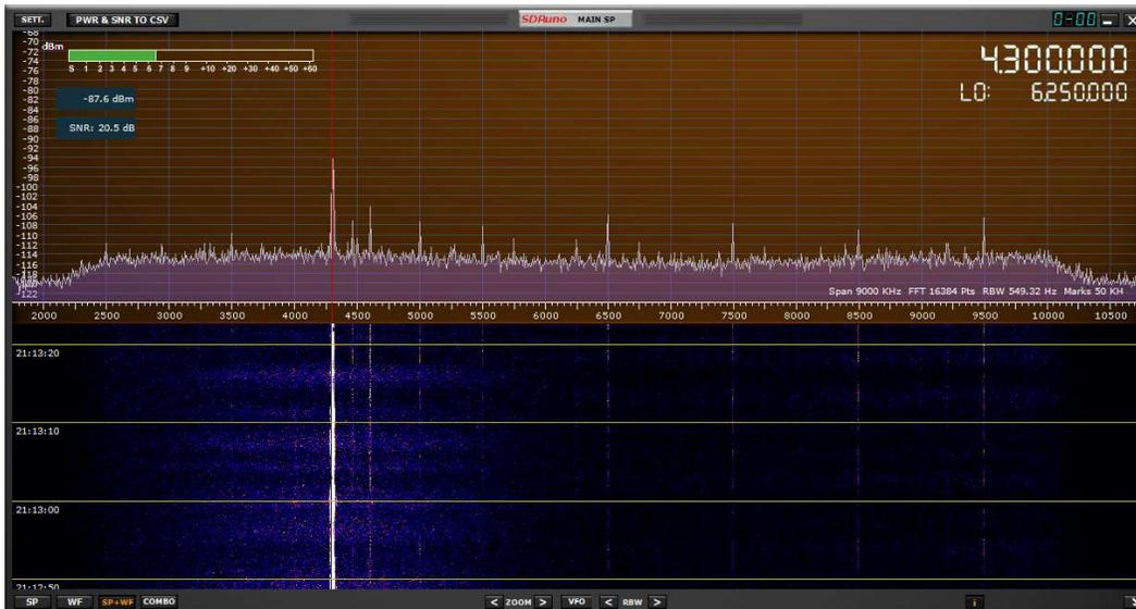
Figure 10.a ~ Comparison of SDRuno and SpectraVue spectrum/waterfall displays for multi-carrier reception on 30 July 2018, 2113 UTC, 4.3 MHz. Both displays have 8 MHz span.
