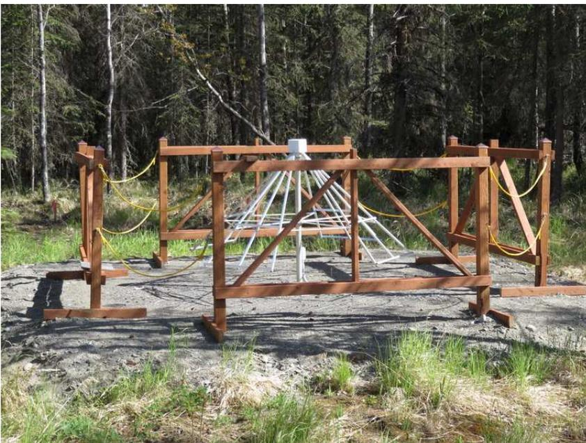
Figure 7 ~ Long Wavelength Array (LWA) antenna at Cohoe Radio Observatory. The crossed-dipole assembly is protected from rampaging moose by the wood fence and is placed with a ground screen on a sandy-gravel pad behind the observatory building. The pad is shown entirely in this image, and its dimensions are 7.6 x 7.6 m. The antenna itself is 1.5 m high. Image © 2018 W. Reeve
