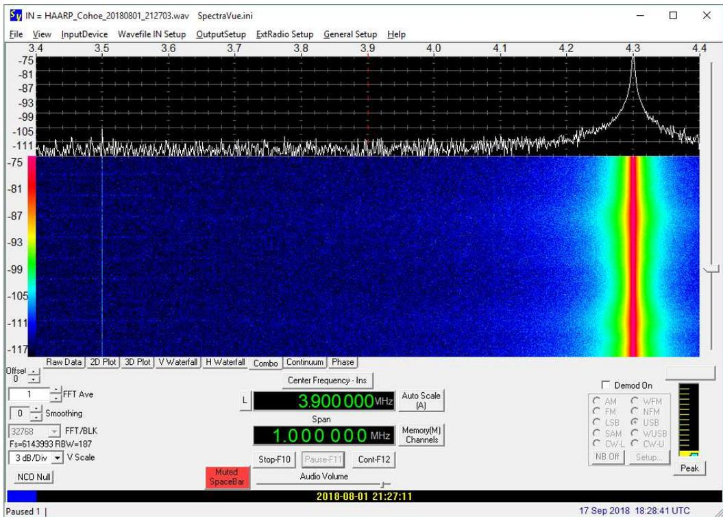
Figure 13.g ~ SpectraVue: 2127 UTC, 01 August, Recording: 4.300 MHz. Displayed frequency span is 1 MHz with no demodulation.
