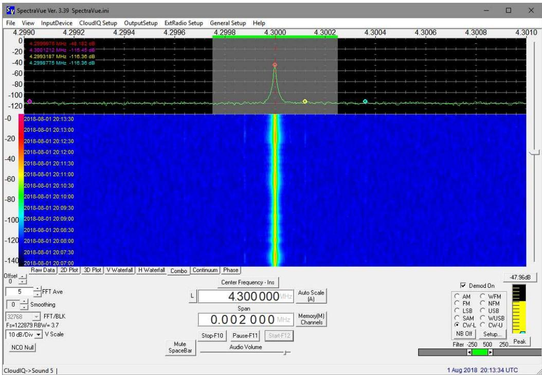
Figure 13.a ~ SpectraVue: 2013:34 UTC, 01 August, Live: 4.300 MHz, source of spectral blooming unknown but it may be due to the very high received signal levels. The displayed frequency span is 2000 Hz and demodulation is set to CW-low.
