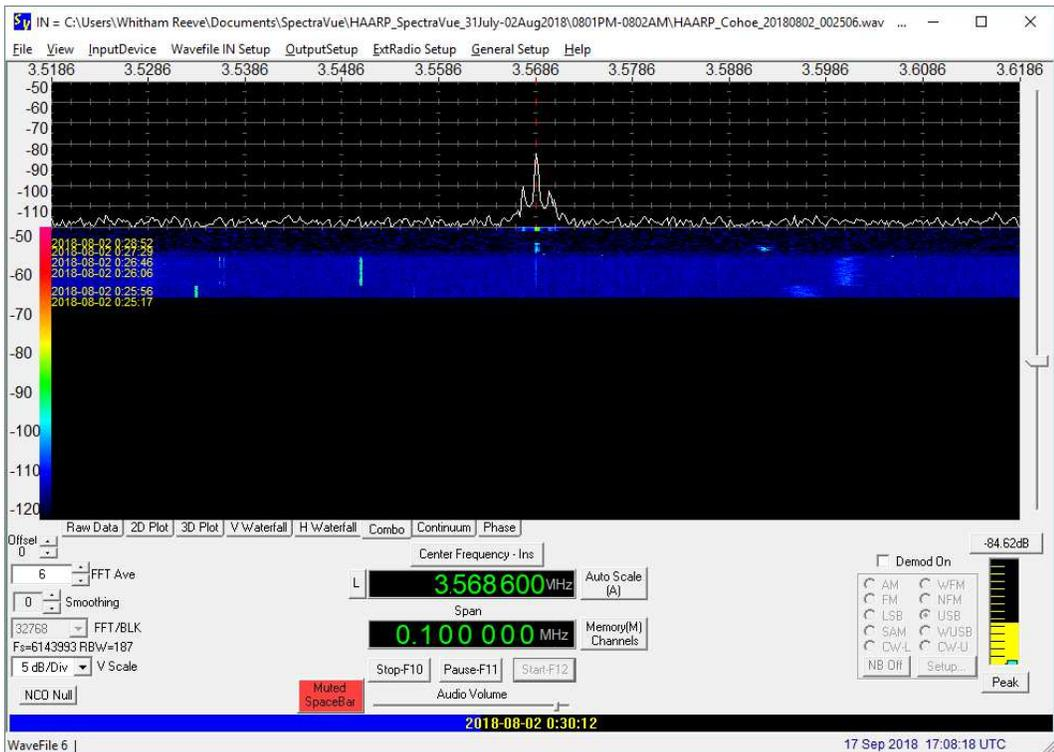
Figure 15.b ~ SpectraVue: 0030:12 UTC, 02 August, Recording: 3.5686 MHz WSPR (“low elevation”); no demodulation.
