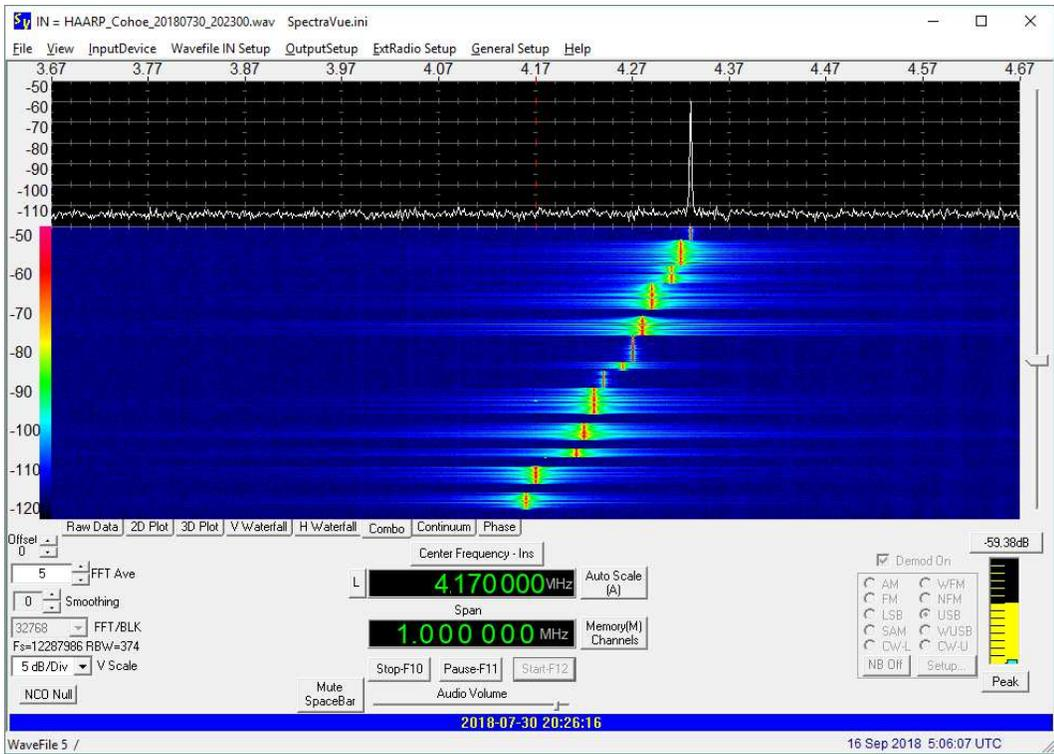
Figure 11.f ~ SpectraVue: 2026 UTC, 30 July, Recording: Stepped frequencies with different separation and duration. Displayed frequency span is 1 MHz.
