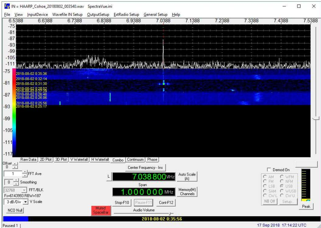
Figure 15.c ~ SpectraVue: 0035 UTC, 02 August, Recording: 7.0386 MHz WSPR (“low elevation”); no demodulation.
