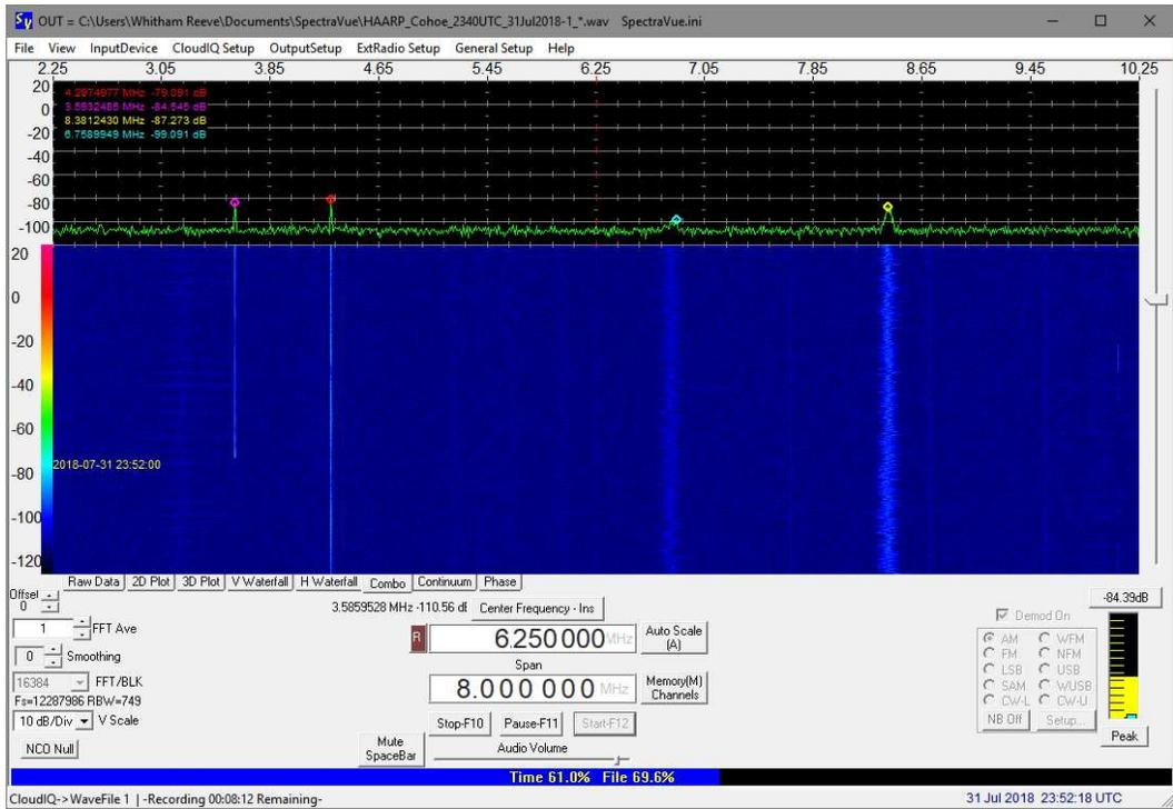
Figure 12.e ~ SpectraVue: 2352 UTC, 31 July, Live: 3.5926 MHz WSPR. Displayed frequency span is 8 MHz with no demodulation.
