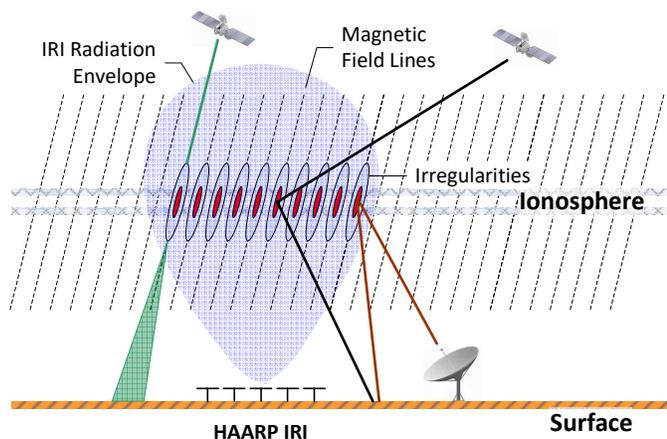
Figure 2 ~ FAIS experiment schematic. The HAARP IRI produces electron density striations (irregularities) in the ionosphere, which scatter man-made ground-ground and ground-space signals. The scattering, which occurs in the HF through UHF frequency bands, can enable or disrupt communication links. Image adapted from [{DTIC}](#)
