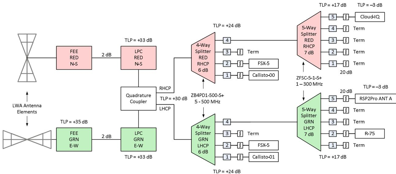
Figure 9 ~ RF transmission level diagram for the LWA antenna and receiver systems at CRO. All transmission levels shown are nominal. All unused splitter ports are terminated in 50 ohms. TLP: Transmission Level Point. Image © 2018 W. Reeve
