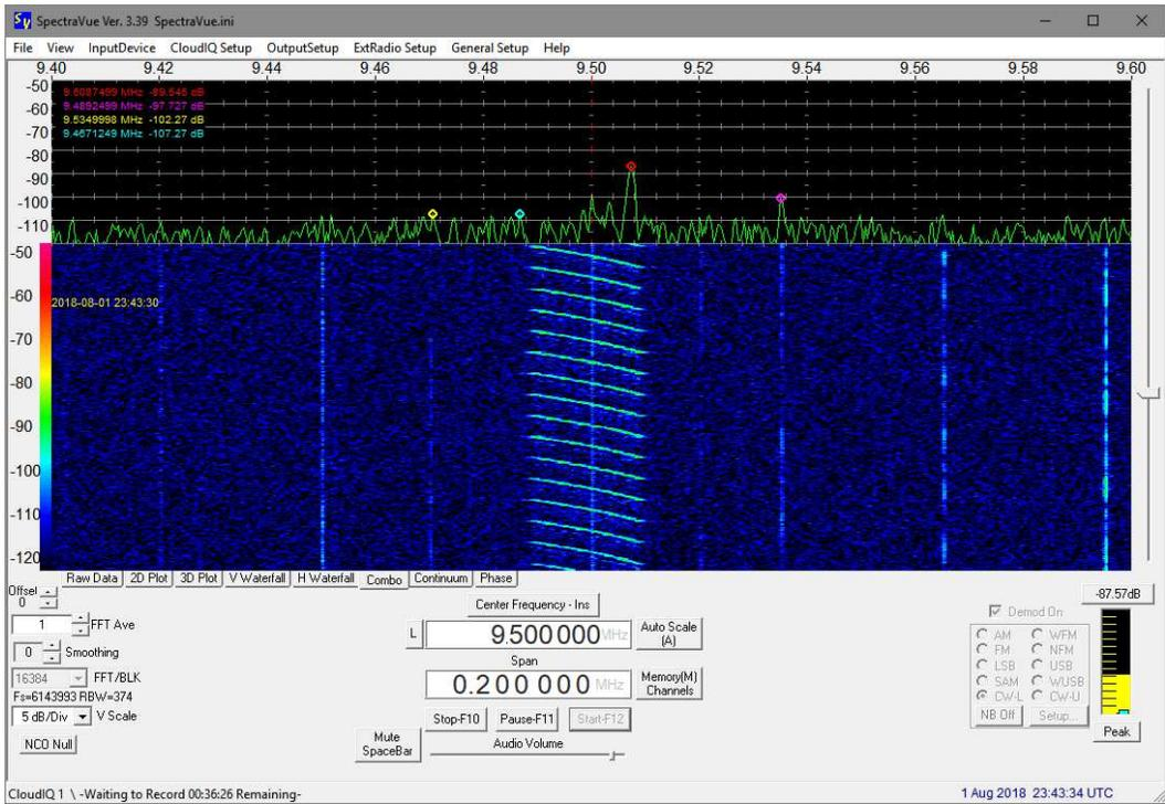
Figure 10.d ~ 01 August 2018, 2343 UTC. Live: 9.5 MHz, 200 kHz span, Frequency Modulation.
