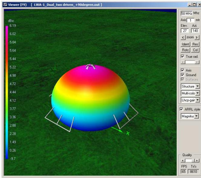
Figure 8 ~ Long Wavelength Array antenna radiation pattern. The antenna is most sensitive near vertical but has good response at low angles as well. The 3-D image shown here was produced by 4NEC2 numerical electromagnetic code modeling software {4NEC2}. A description of the LWA antenna model may be found at {ReeveLWA}.
