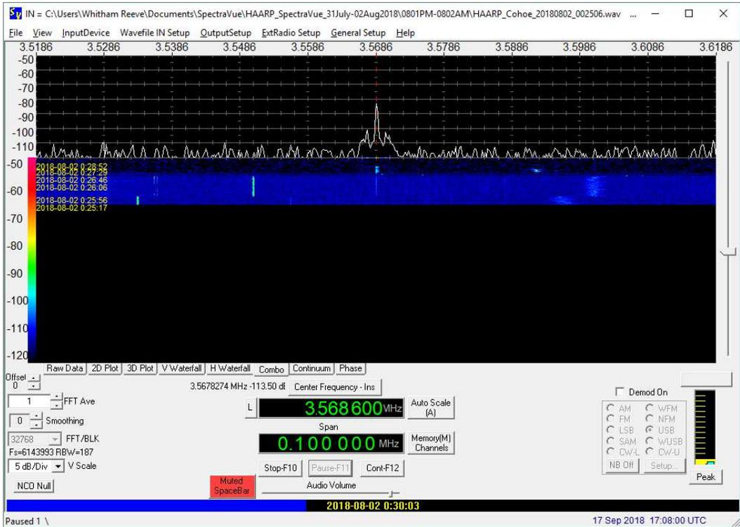
Figure 15.a ~ SpectraVue: 0030:03 UTC, 02 August, Recording: 3.5686 MHz WSPR (“low elevation”); no demodulation.
