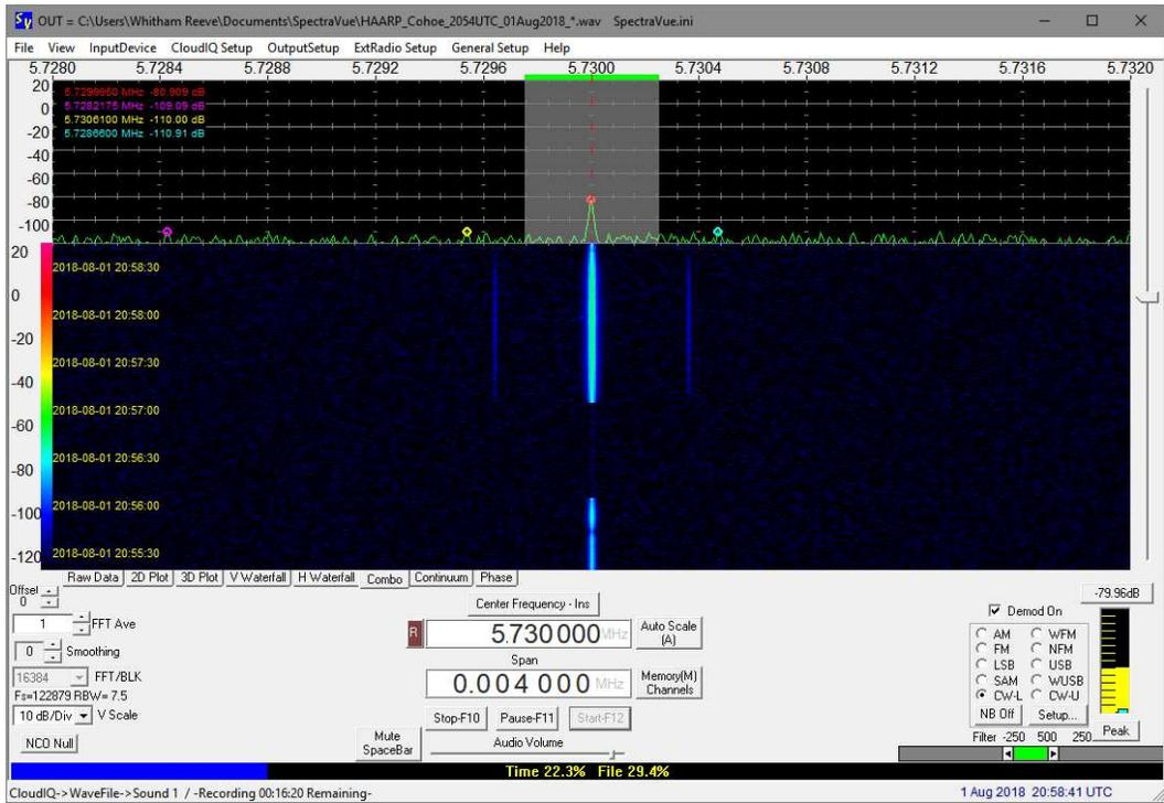
Figure 13.c ~ SpectraVue: 2058 UTC, 01 August, Live: 5.730 MHz. Displayed frequency span is 4000 Hz and demodulation is set to CW-low.
