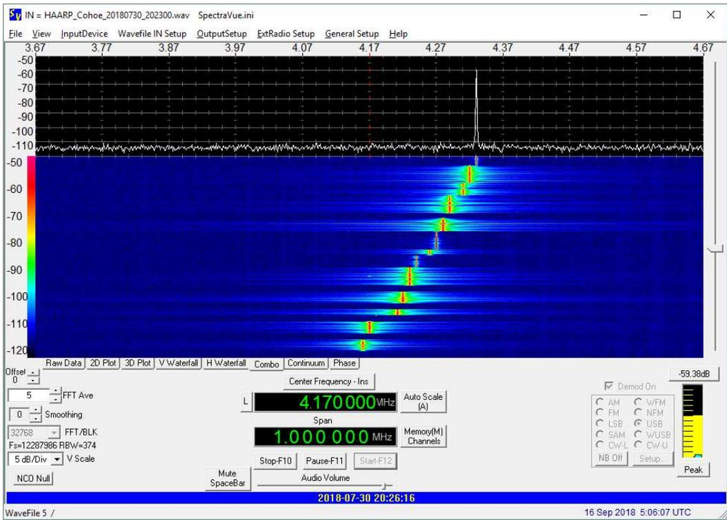
Figure 10.b ~ Stepped carrier, 30 July 2018, 2026 UTC. Playback: Display centered at 4.17 MHz. the step size and transmission time duration varies. The “blooming” effect may be due to the modulation being used. It is not caused by the receiver or software – it disappears during reception of the last carrier displayed here.
